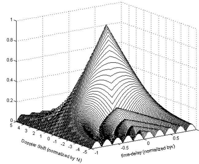
Zero Doppler Cut    Zero Time-Delay Cut
