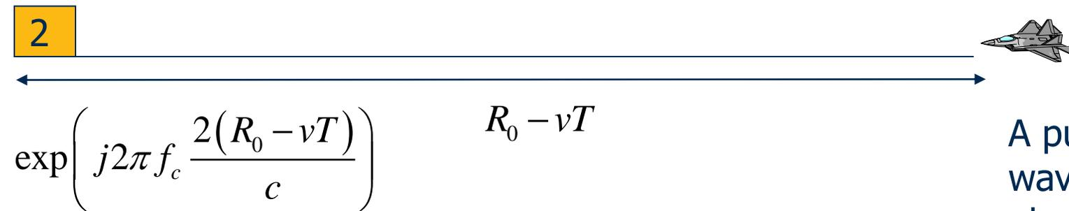
A pulsed Doppler waveform measures the phase change between pulses
