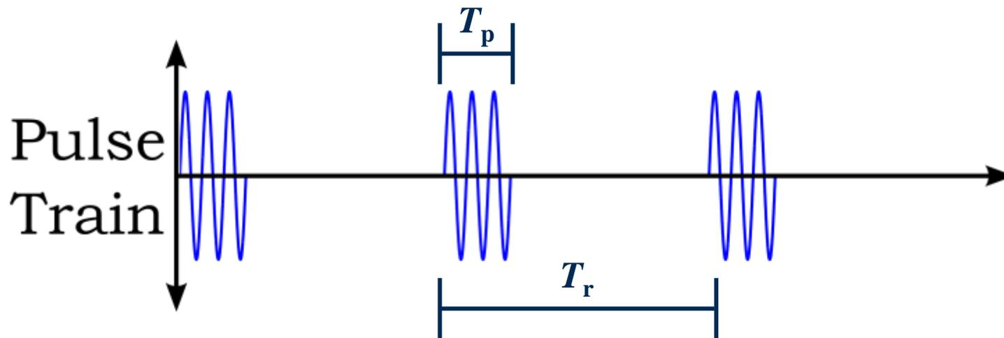
$$\text{Duty Cycle: } d \triangleq \frac{T_p}{T_r}$$
