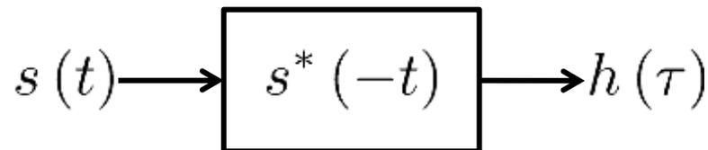
The range response,  $h(\tau)$ , of a waveform is the auto-correlation function of the transmitted signal.
