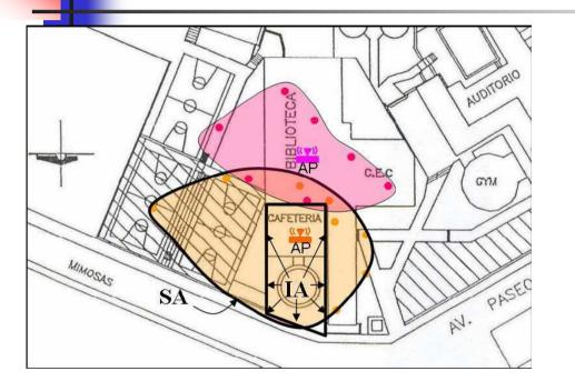
The cell-id location method: wireless devices associated to one AP are geographically located within that AP service area.
