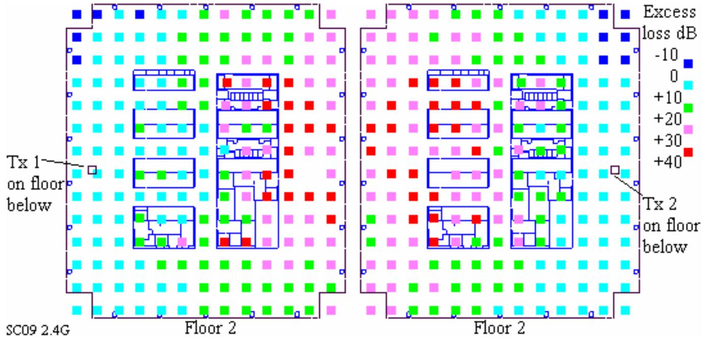
**The distribution of excess losses on floor 2 reflect the transmitter positions, but the effect of the adjacent building is not obvious.**
