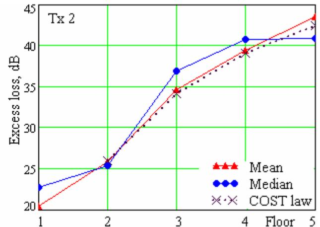
**Performance of inter-floor models optimised for all floors taken as one dataset, for each transmitter at 2.4 and 10 GHz,  $b = 0.54$ ,  $G_r = 3.5$  dB**
