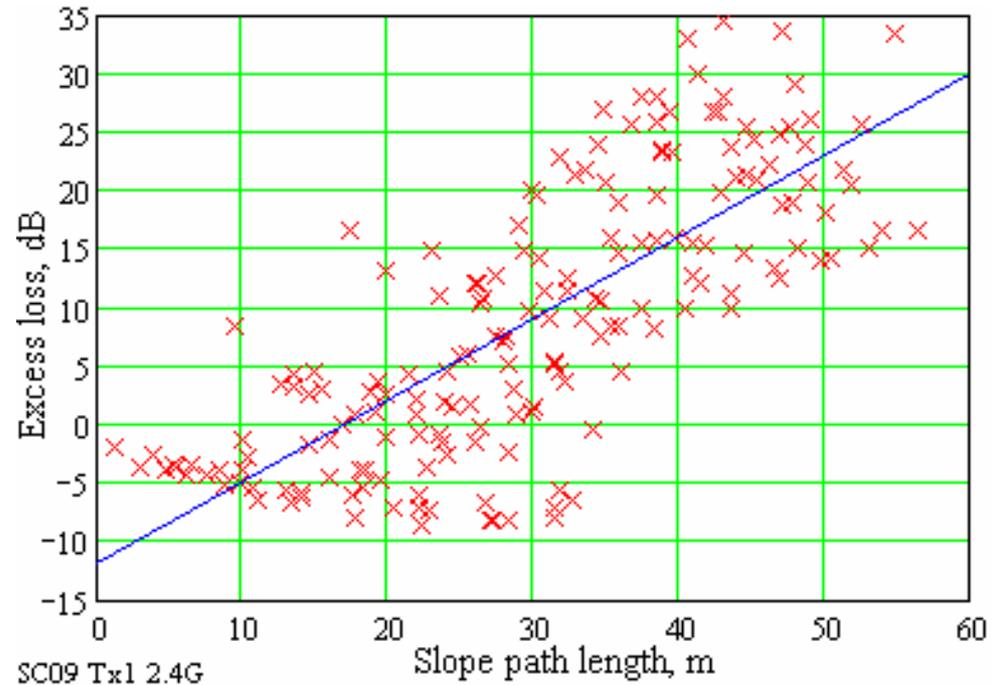
**A linear-regression fit to excess losses plotted against slope path length shows a negative intercept on the excess-loss axis: -11.8 dB.**
