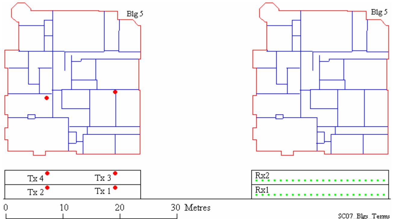
To test the effect of openings, i.e., doors, windows, etc, are "exploited" by rays, losses from Txs 1 and 3 were ray-traced for 2.4 GHz and 5.8 GHz both normally, and with all openings closed by the surrounding surface properties, i.e. wall, etc.
