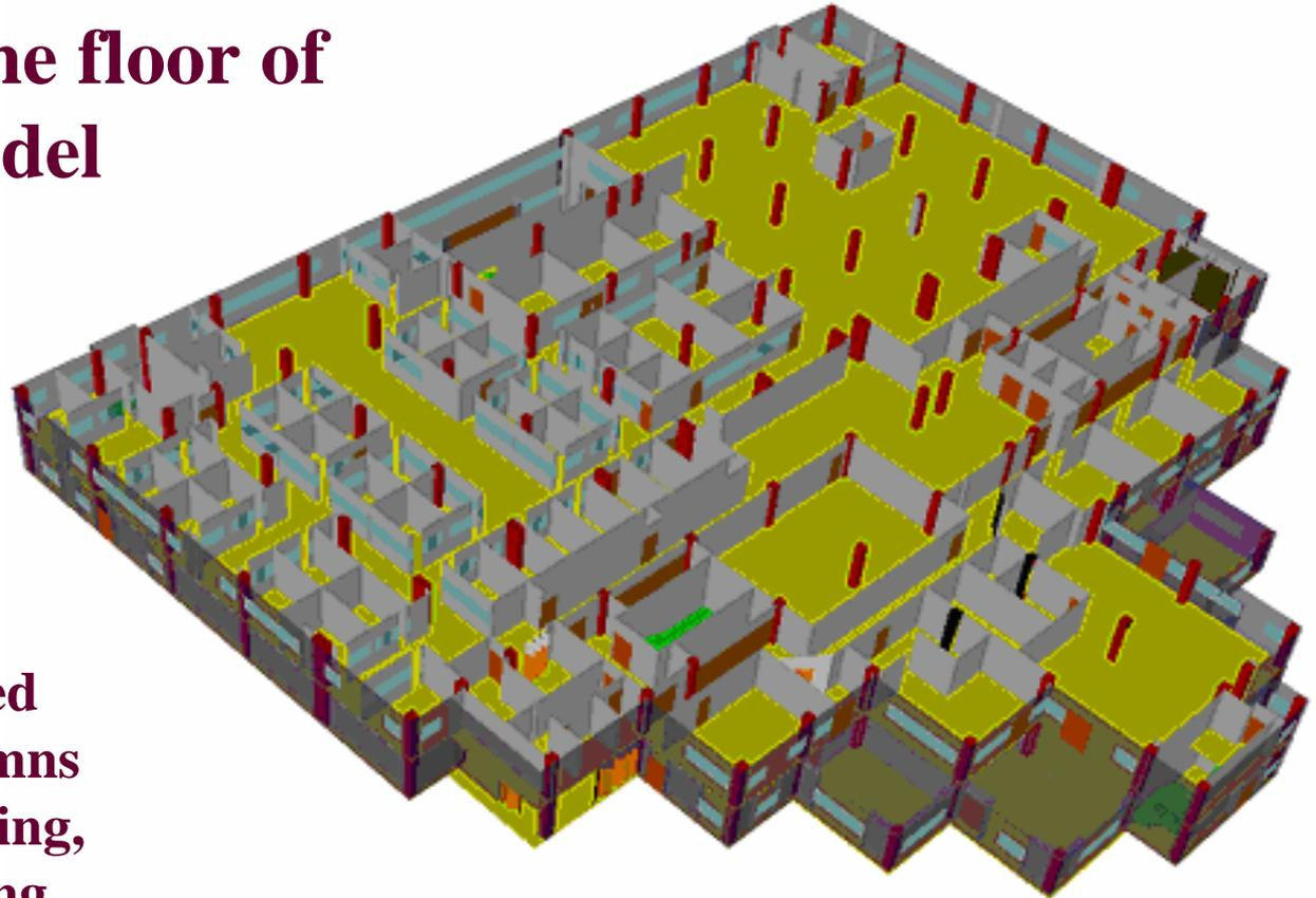
Floors supported mainly by columns inside the building, plus load-bearing external walls.
