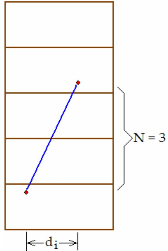
Note that  $d_i$  is zero for a vertical path between floors
