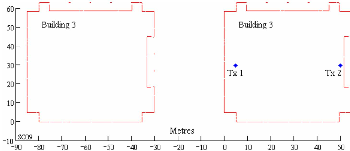
**Two transmitter locations on floor 1 of right-hand building to compare the effect of an adjacent building on the left.**
