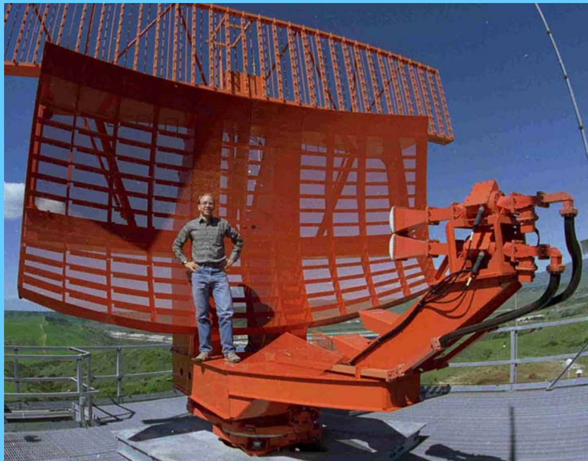
An example of a fixed, ground-based 3-GHz airport surveillance radar antenna.
