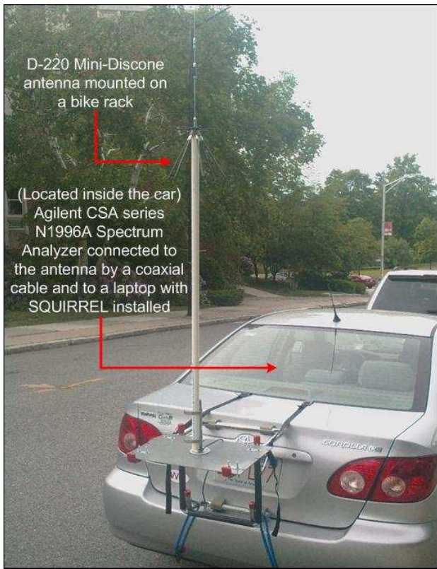
Fig. 5. A photograph of the employed mobile wireless spectrum measurement testbed, which includes a mini-discone/ridged-horn antenna, a spectrum analyzer and a laptop with SQUIRREL installed (from [12]).
