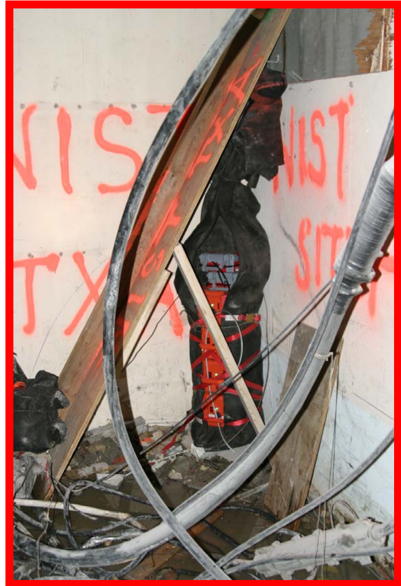
Transmitters are secured to the wall and protected from falling debris by a board
