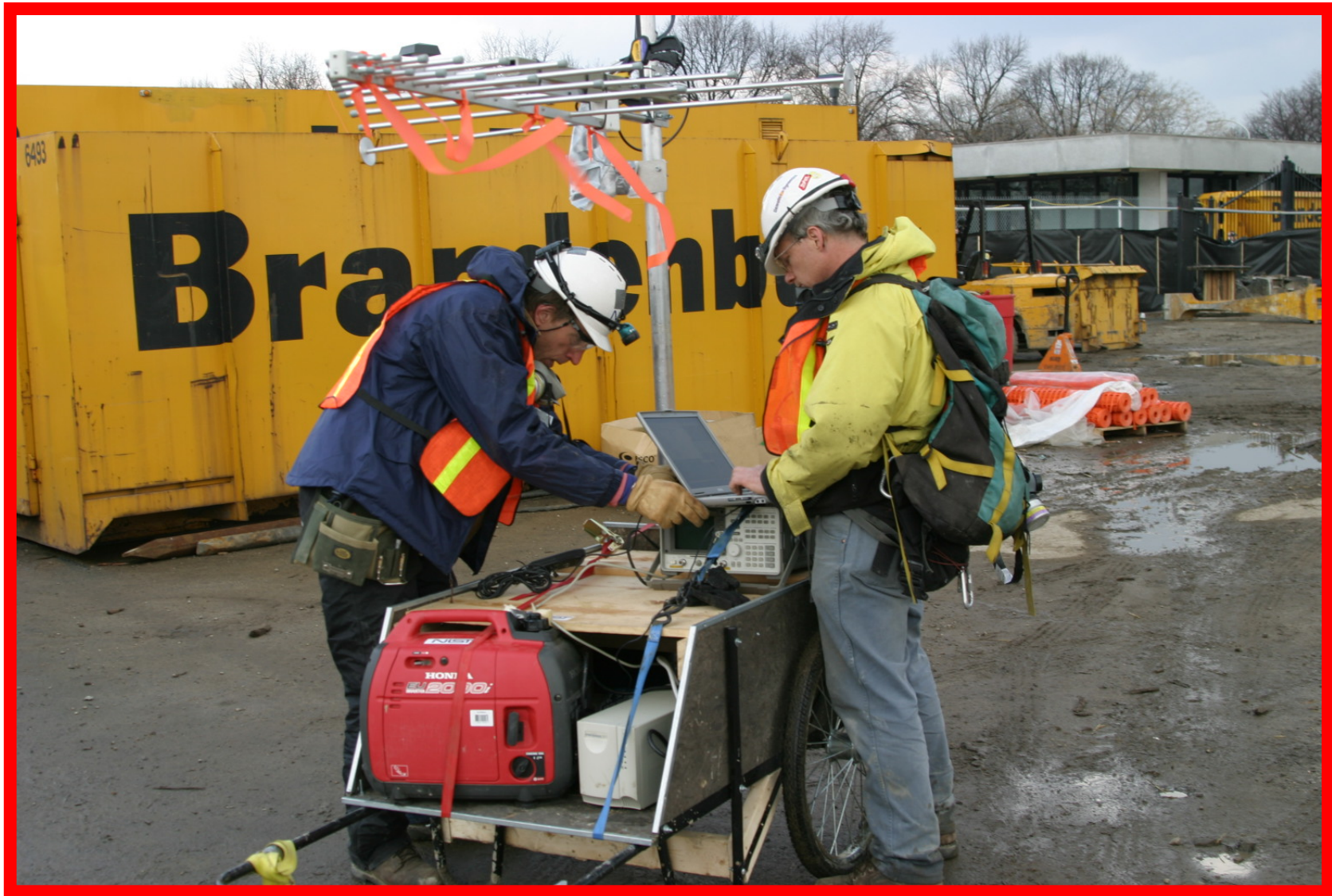
Mobile cart: antenna, generator, UPS, laptop & spectrum analyzer
