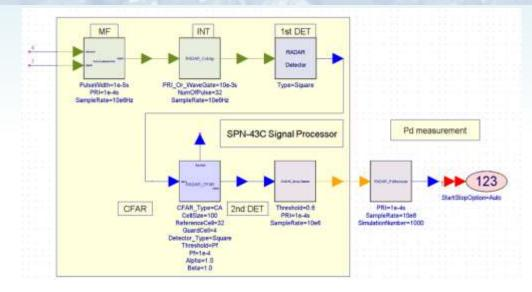
Navy radar signal processing simulation block diagram with:
