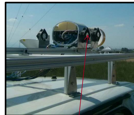
External fan bank to emulate airflow from flight
