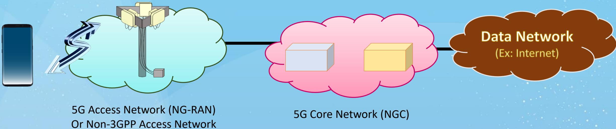
$$\text{UE} + \text{5G Access Network} + \text{5G Core Network} = \text{5G System}$$
