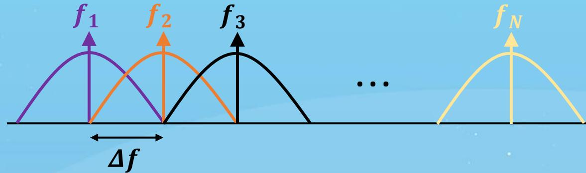
$\Delta f$ : 15 kHz (LTE);  $15 \times 2 = 30$  kHz;  $30 \times 2 = 60$  kHz;  $60 \times 2 = 120$  kHz
