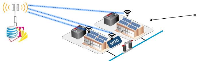
State 1 – Normal: MicroGrid controlling devices in communication with commercial cellular infrastructure
