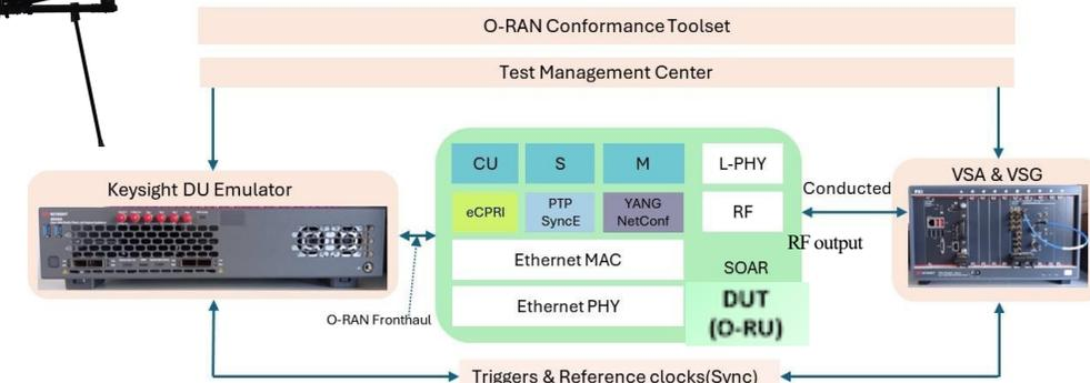
Fig. 2 AERPAW OTIC O-RU Conformance Test setup
