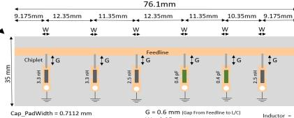
Cap\_PadWidth = 0.7112 mm Cap\_PadLength = 0.894 mm // 0.694 mm Ind\_PadWidth = 0.5004 mm Ind\_PadLength = 0.95 mm // 0.75 mm
