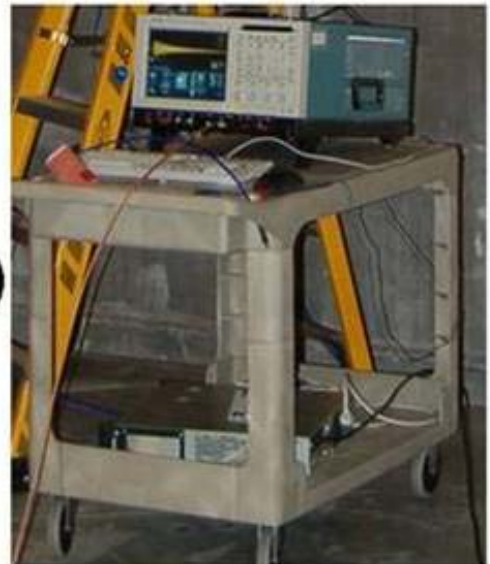
Figure 4. (a) Setup for horizontal scans. (b) Pulse generator inside a shielded box. (c) Oscilloscope mounted on receiving cart.
