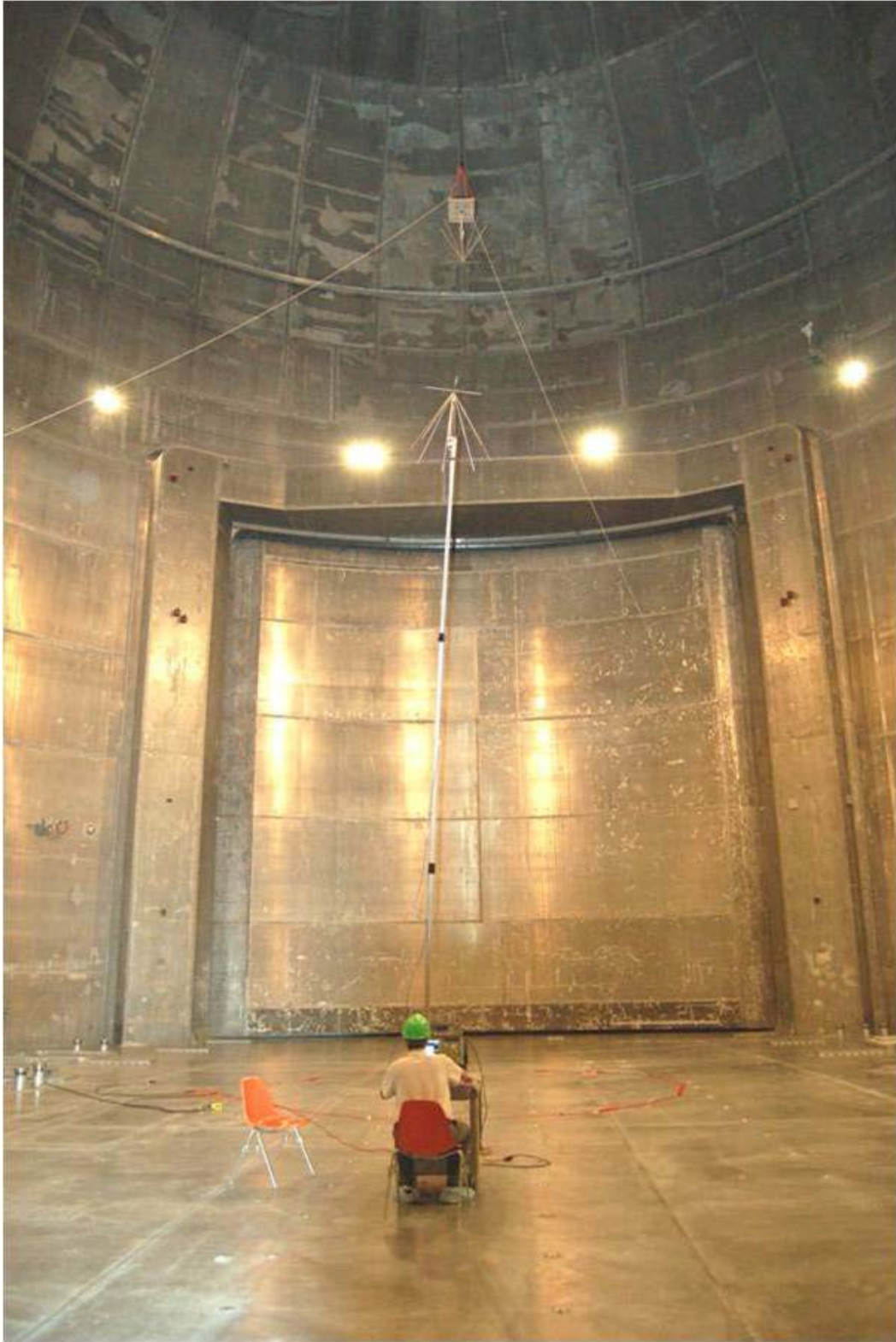
Figure 6. The vertical scan test setup with operator at the receiving cart. The transmitter is supported by nylon rope from above.
