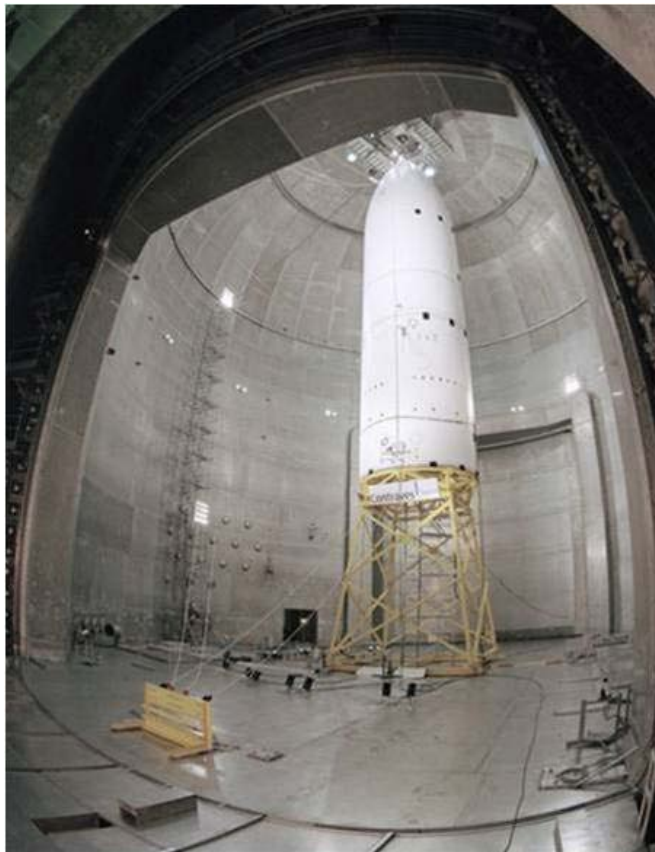
Figure 1. The SPF vacuum chamber with typical test article. Note the large access doors and buttresses in front of and behind the rocket.
