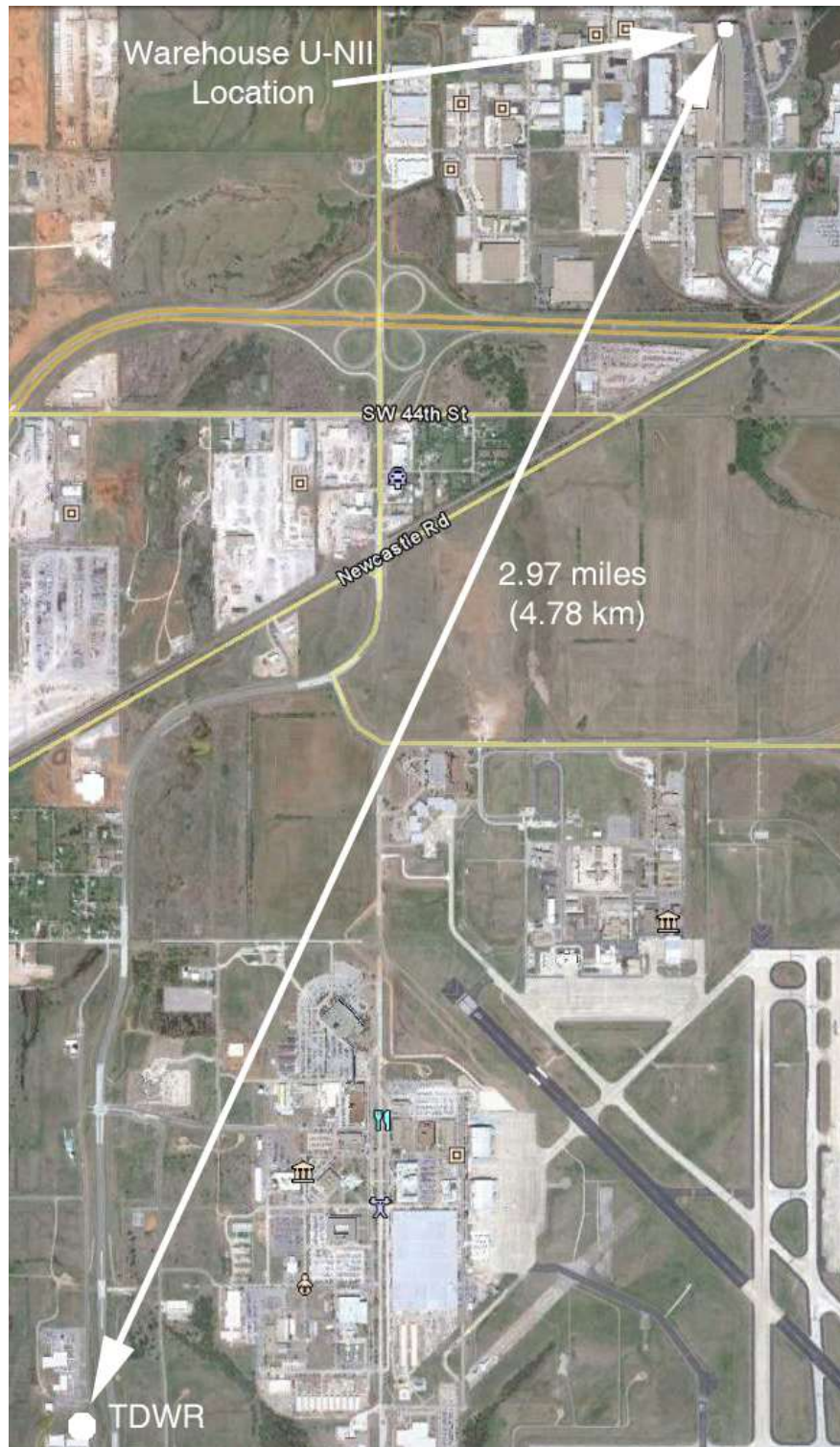
Figure 4. Geometry of the PSF TDWR and the FAA warehouse facility where the U-NII master devices were located. 20
