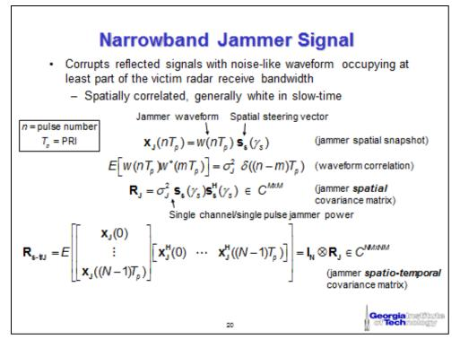
Figure 17. Formulation of the single narrowband jammer incident on a radar array antenna.
