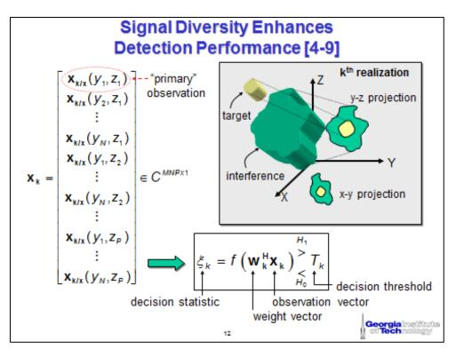
Figure 15. Signal diversity enhancements to detection performance—references in slide refer to [12], [13], [14], [15], [16], and [17].
