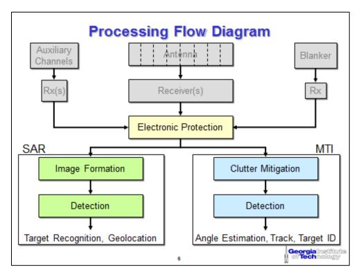
Figure 13. Processing flow diagram for a generalized radar receiver.
