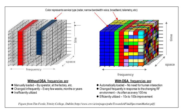
Figure 2. The "Spectrum Cube" vision is for a dense use spectrum use with diverse services sharing with minimal frequency, space and time spaces.
