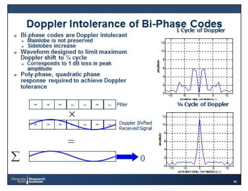
Figure 9. Doppler intolerance of bi-phase codes.
