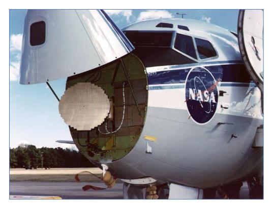
Figure 51. Airborne weather radar used in airliners.
