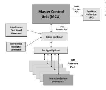
Figure 7. Test Set-Up.
