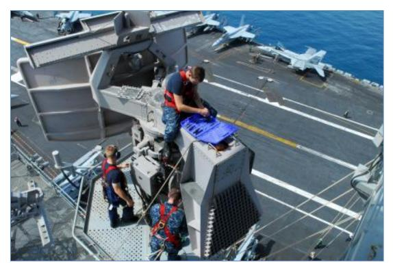
Figure 47. SPN-43C naval ATC (navigation) radar (courtesy: Defense video and imagery).
