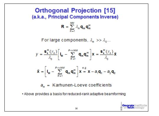
Figure 22. Interference mitigation via eigenvector cancellation—reference in slide refers to [23].
