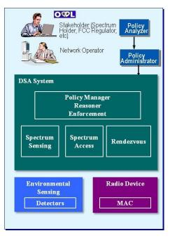
Figure 5. Shared Spectrum Company's DSA 2100 radio system is policy language controlled, which enables it to accomidate most of the incumbant DSA concerns.
