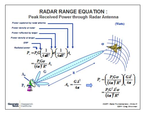
Figure 3. Radar range equation.
