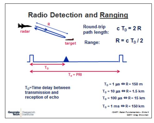
Figure 2. Estimating range with a pulsed radar system.
