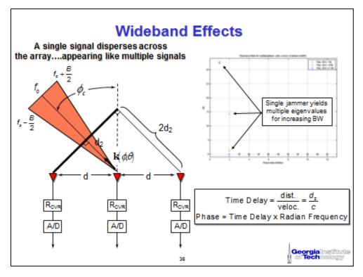
Figure 26. Interference effects on a wideband receive array.
