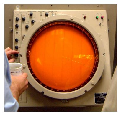
Figure 45. ASR plan position indicator display.
