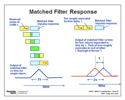
Figure 4. Radar matched filter response of one and two targets.
