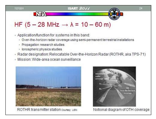
Figure 38. HF over the horizon radar.
