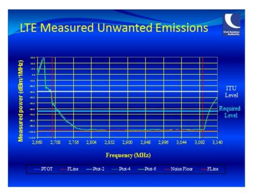
Figure 60. Measured WiMAX/LTE emissions with current ITU and CAA required OOB limits.
