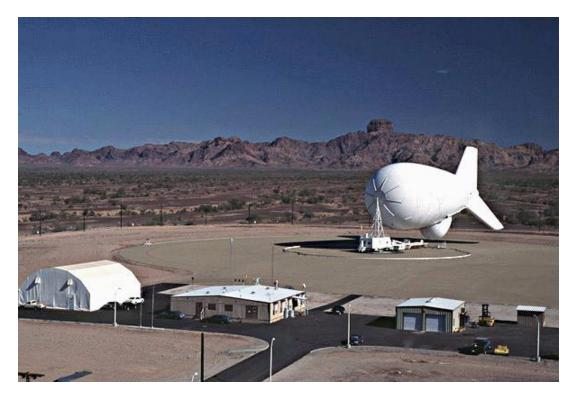
Figure 41. Balloon-mounted Aerostat L-band long-range radar.
