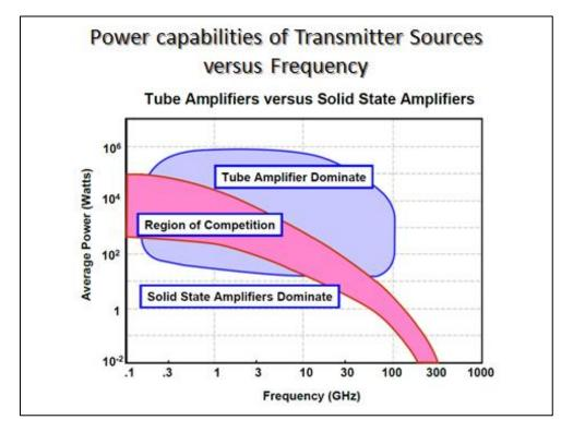
Figure 29. Tube versus solid state amplifier regions in terms of power and frequency.
