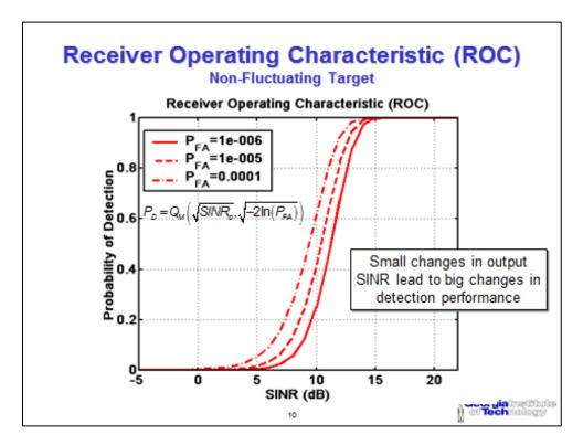
Figure 14.  $P_d$  versus SINR for a non-fluctuating target.
