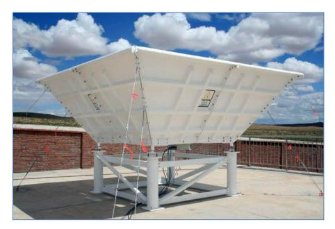
Figure 40. Lower L-band wind profiler radar.
