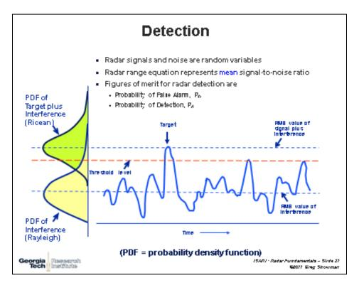
Figure 5. Illustration of radar amplitude detection.
