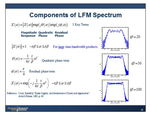
Figure 7. Frequency characteristics of LFM waveforms.
