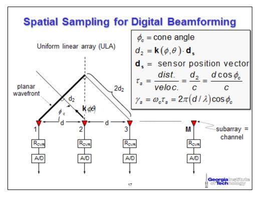
Figure 16. Spatial sampling for digital beamforming.
