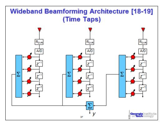
Figure 27. Wideband beamforming architecture used for STAP.
