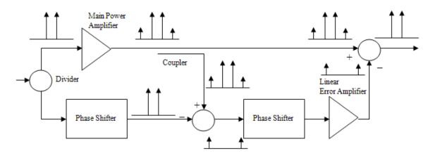
Figure 31. Feedforward approach to subtracting out IMPs.
