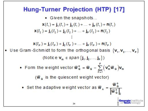
Figure 24. Array weights via Hung-Turner Projection—reference in slide refers to [25].
