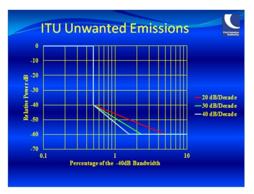
Figure 57. ITU radar emission limits.
