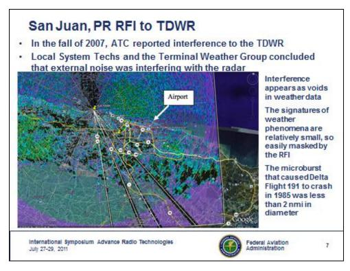
Figure 61. Example of RFI interference to TDWR from U-NII DFS devices.
