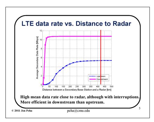
Figure 72. LTE performance versus radar-LTE separation.
