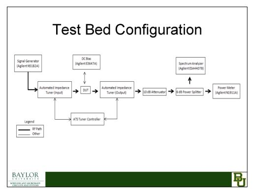
Figure 65. Waveform/Impedance optimization test bed configuration.
