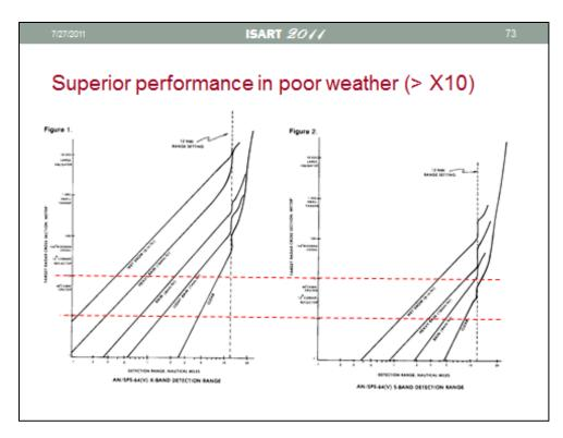
Figure 49. Performance comparison of X- to S-band maritime radar systems operating in different weather conditions.
