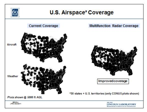
Figure 66. Improved overall coverage if MPAR replaced weather and aircraft surveillance radars.
