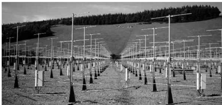
Figure 5-14. 46.5 MHz Wind Profile Radar in UK
