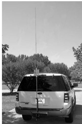
Figure 3-4. Vehicle-Mounted Whip Antenna
