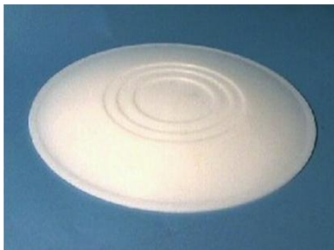
(a) Fresnel Lens (Showing Four Superimposed Lenses)
