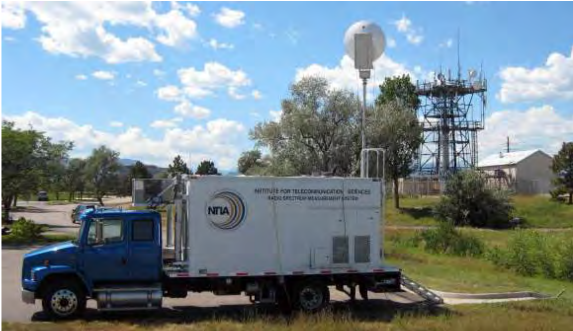
Figure 19. NTIA RSMS during in situ BRS WiMAX measurements at Broomfield, Colorado. Photo by author Sanders.
