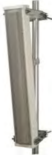
Figure 16. A 2.6 GHz WiMAX base station sector-coverage antenna with +16 dBi gain and 90-degree azimuth coverage. Note mechanical down-tilt feature.
