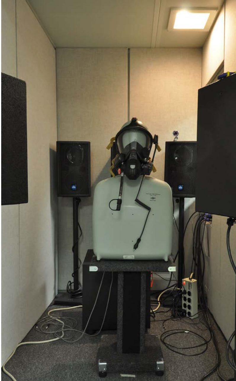
Figure 1. HATS set up in a sound-isolated booth.
