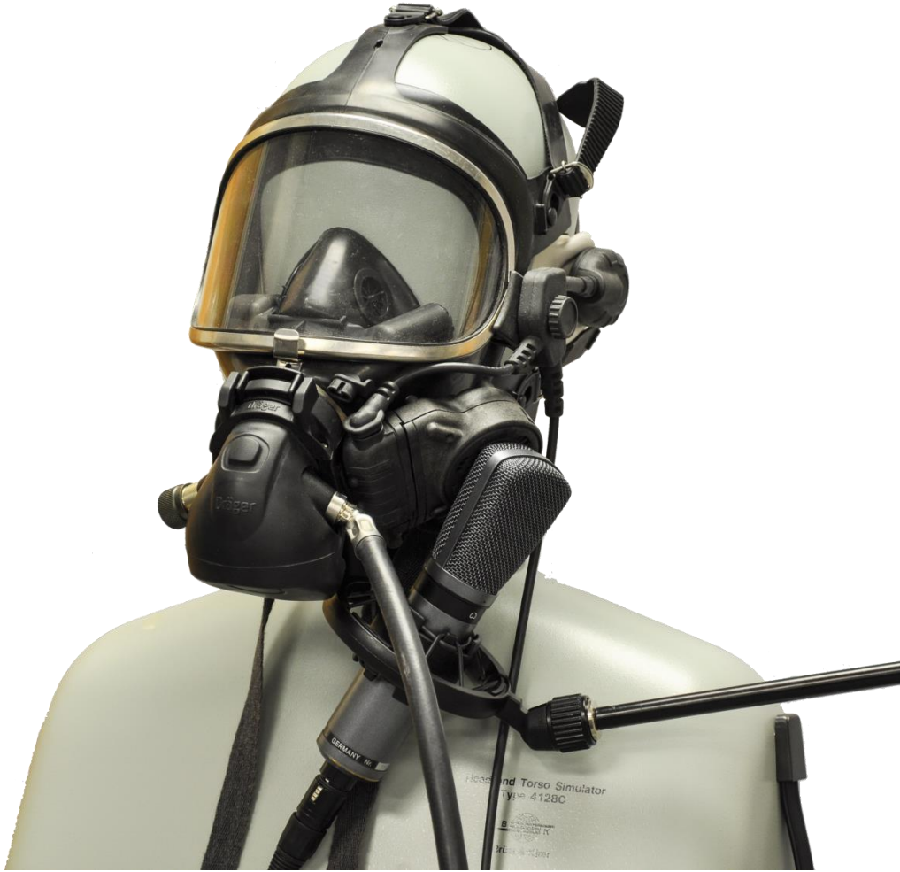
Figure 3. Photograph depicting a HATS set up to speak through the vox port of an example SCBA mask to a microphone.
