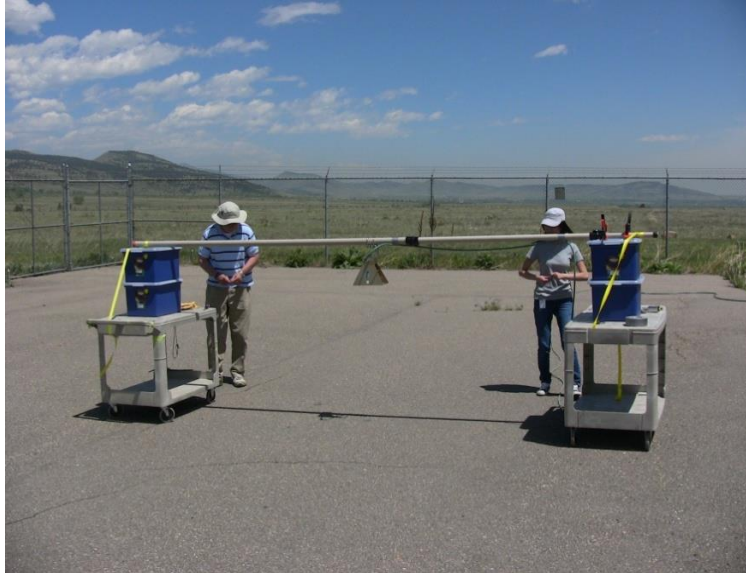
Figure 2. Setup for Building A4 parking lot for measurement of ground constants.
