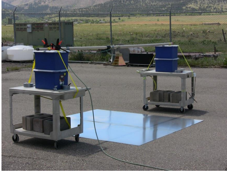
Figure 3. Setup for Building A4 parking lot for calibration measurement reference over aluminum sheet.
