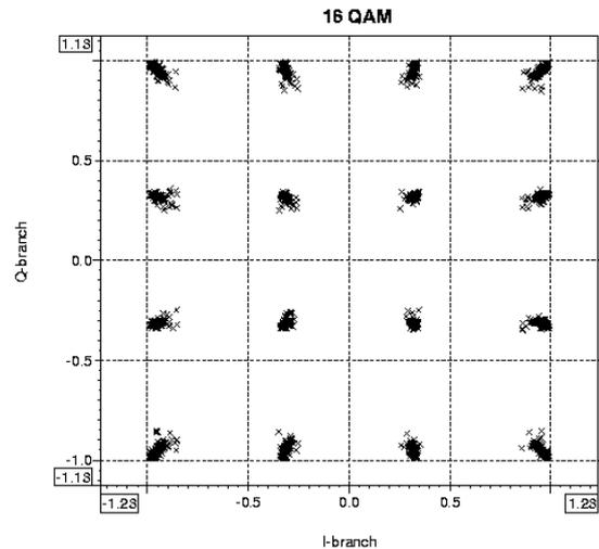
Figure V-3 3-coefficients pre-equalizer
