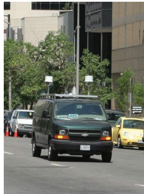
The ITS receiver van performing propagation measurements in the downtown Denver dense urban high-rise city environment. Photo by Robert Johnk.
