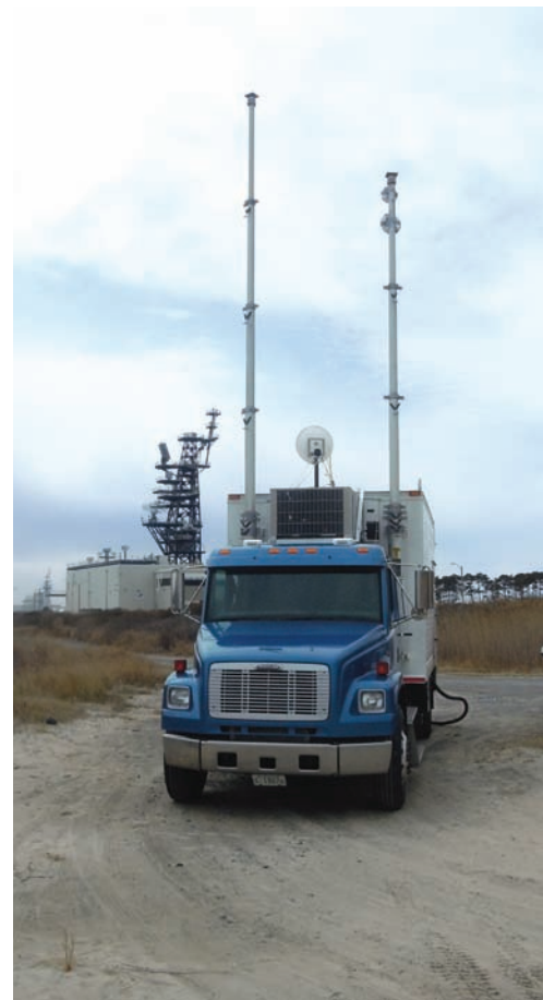
Figure 1. The RSMS truck collecting emission measurement data from Navy radar systems. Photo by John E. Carroll.
