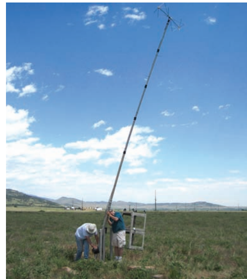
Figure 1. ITS engineers set up equipment for measuring the dielectric properties of soil. Photo by Wayde Allen.
