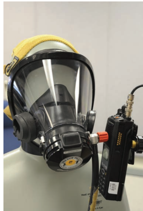
Figure 1. An ITU standard Head and Torso Simulator (HATS) outfitted with a firefighter's mask and set up to talk into a radio. Photo by Ken Tilley.
