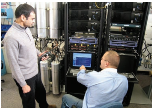
ITS staff examine the operational configuration characteristics of a Project 25 trunked LMR system in the ITS Public Safety RF lab. Photo by Ken Tilley.
