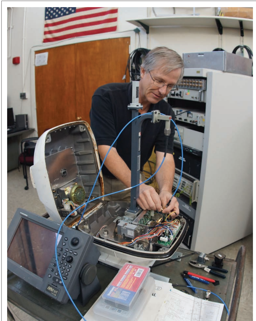
Dr. Robert Johnk of the ITS Theory Division prepares a maritime radar receiver for interference-effects testing for an other-agency sponsor. Such work is critically important in spectrum-sharing studies performed by the Institute. Photo by Frank Sanders.
