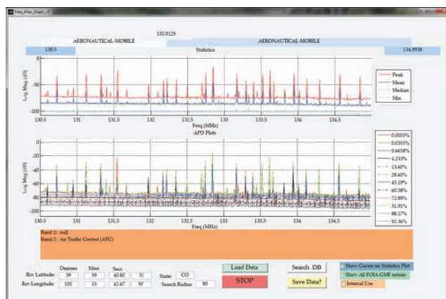
Frequency Allocation Forensics software screen capture: Statistical representations of real radio traffic in the aeronautical mobile band.
