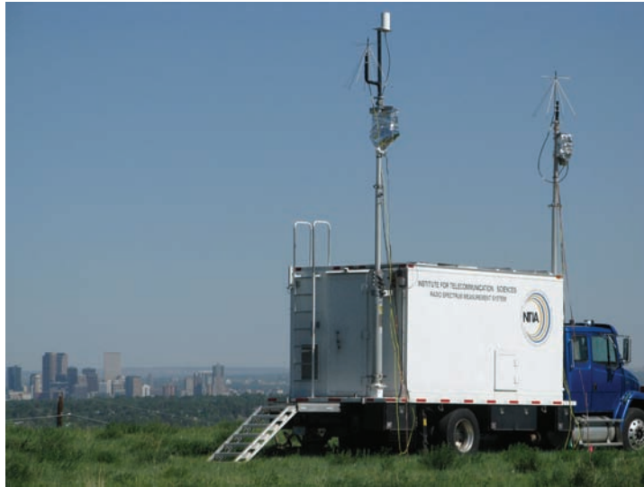
Figure 1. RSMS-4 measurement vehicle in Arvada, CO, while performing a spectrum survey.
