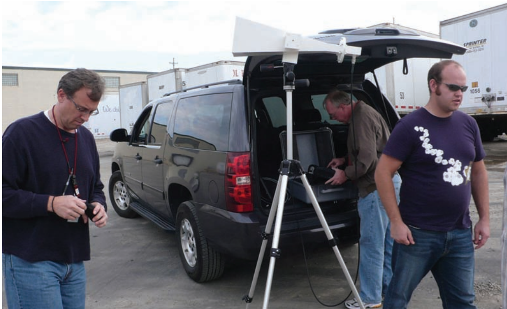
Above: ITS and other Government engineers performing field measurements to identify interference sources. Below: An ITS engineer performs electromagnetic compatibility measurements inside a weather radar bubble 24.4 meters (80 feet) above the ground while observers from the FCC, FAA, and NWS observe. Photos by Frank Sanders
