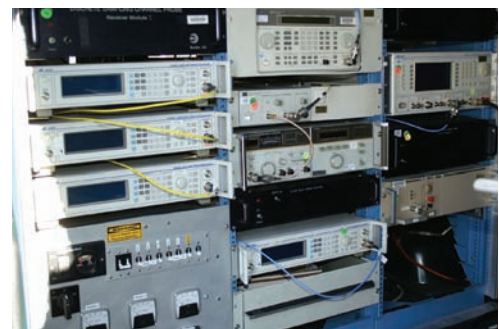
Radio propagation measurement equipment racked in the receiver van.
