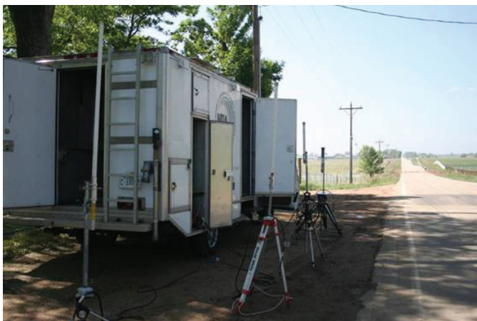
Figure 2. Open rural areas and long distances present different challenges for accurate modeling. In this photo, the ITS Radio Spectrum Measurement Science (RSMS) truck has been deployed to take measurements in a rural location.
