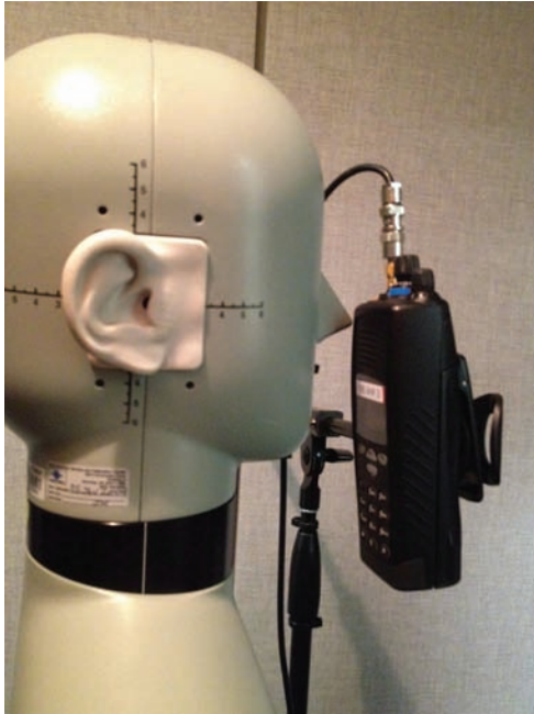
Figure 1. Recordings of phonetically balanced English speech are captured using a reference LMR for later playback in field tests. Photo by Eric Nelson.
