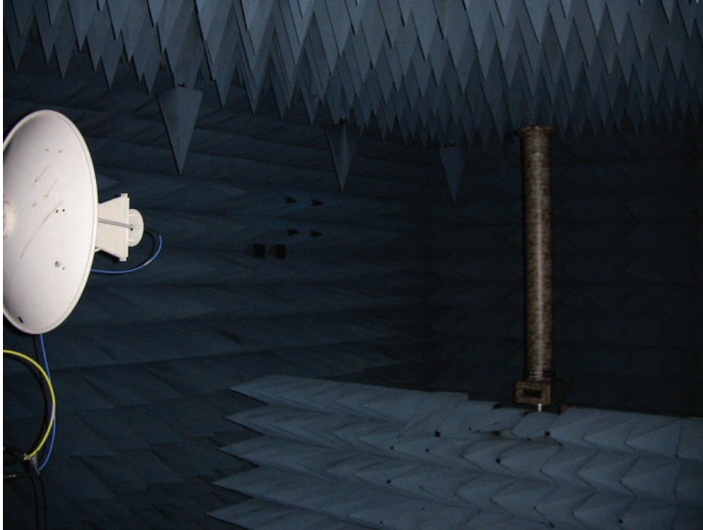
A "short pole" mounted Shore-Line Intrusion Monitoring System (SLiMS) autonomous transmit module is set up in an anechoic chamber at the Department of Commerce Boulder Laboratories, with a receive antenna to capture and measure its emissions. Photo by Robert Achatz.
