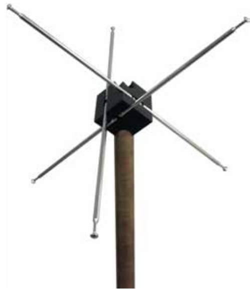
Prototype 3-axis antenna design under development at ITS. Photo by Wayde Allen.
