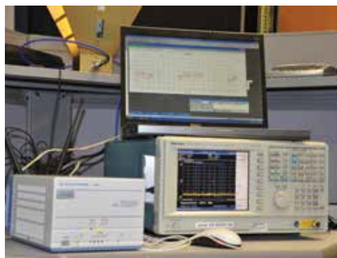
Figure 1 (top). A dual polarized antenna used to receive broadband LTE signals in the 700 MHz spectral range. Figure 2 (bottom). A synchronized dual sampling receiver scanning system that allows examination of the cross-correlation properties of two radiated MIMO signals. Photos by R. Stafford.
