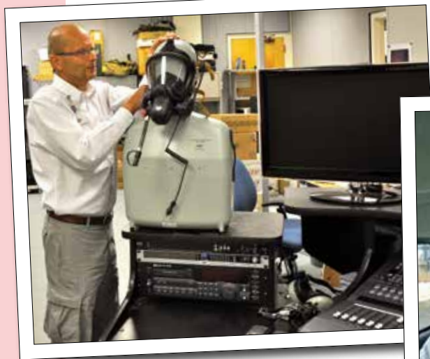
Right: ITS technician Ron Carey configures a transportable public safety LTE base station for interference testing at a public safety land mobile radio transmitter site. Photo by John Vanderau. Below left: ITS engineer John Vanderau configures a head and torso simulator (HATS) to make recordings for audio intelligibility testing experiments. Below right: PSCR technician Sam Gomez and ITS engineer Chris Redding in the PSCR van conducting network drive testing in the field to evaluate an LTE system under test (infrastructure and user equipment) in an operational environment. Photos by Ken Tilley.
