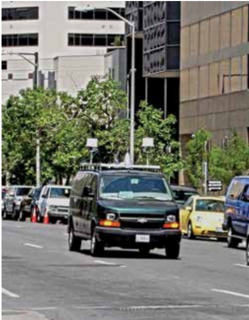
The ITS receiver van performing propagation measurements in the downtown Denver dense urban high-rise city environment. Photo by Robert Johnk.
