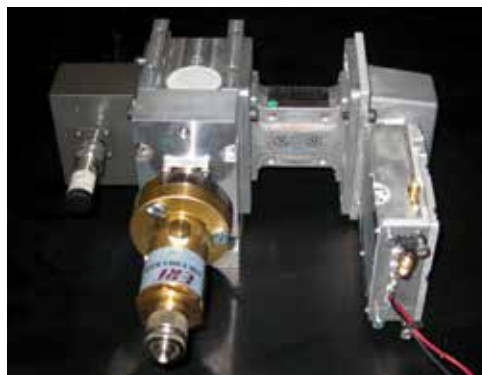
Figure 3 (lower right). Magnetron front end assembly. Components (from left to right) are waveguide terminator, circulator, limiter, and low noise front end. Photo by R. Achatz.
