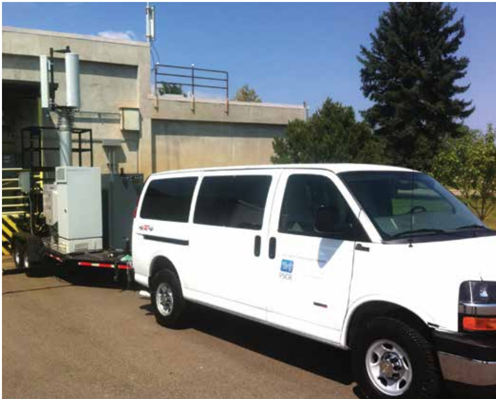
The PSCR drive-test van and the Cell on Wheels (COW) ready for testing. Photo by Ken Tilley.
