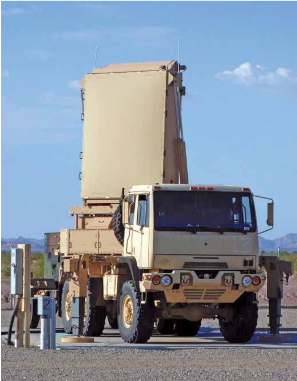
A TPQ-53 counter-fire radar during RSEC compliance measurements at the Yuma Proving Ground. Photo by Frank Sanders, courtesy LMCO and U.S. Army release.
