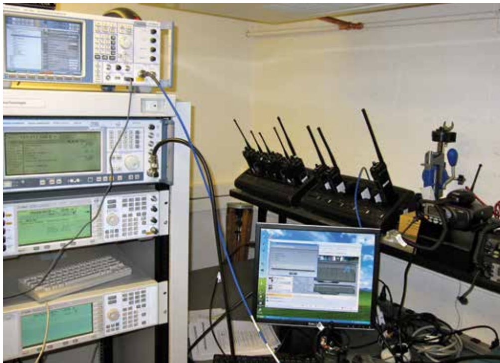
Racks of commercial off-the shelf public safety communications equipment used for testing in the Public Safety Audio Quality Research Laboratory. Photo by Ken Tilley.
