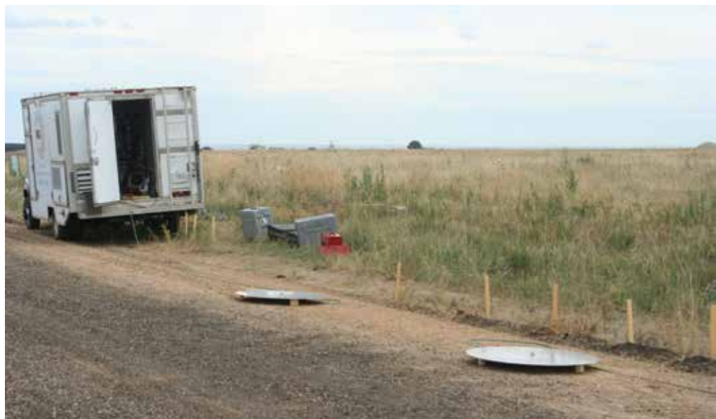
Two monopole-on-a-ground-plane antennas set up for near-Earth propagation measurements at Table Mountain. Photo by S. Carroll.
