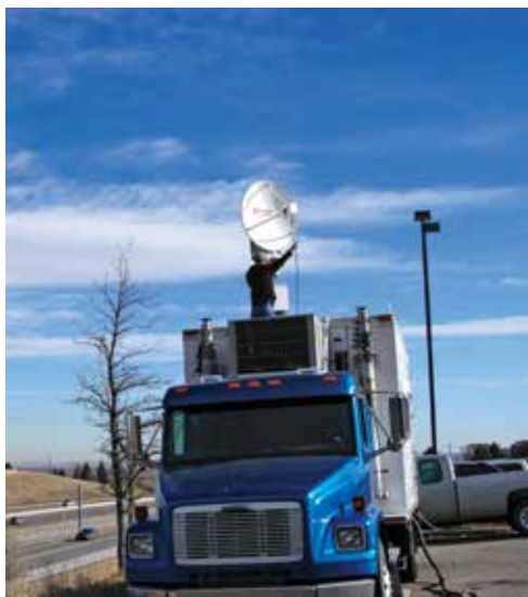
Setting up the RSMS measurement truck in preparation for taking spectrum occupancy measurements as part of ongoing support to OSM, Photo by Chriss Hammerschmidt.
