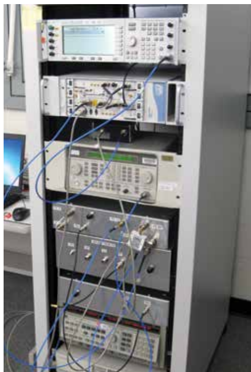
vector signal generator, vector signal analyzer, bandpass filter, signal generator to emulate the radar signal, reference front end and IF, magnetron front end, power supplies, and local oscillator signal generator. Photo by R. Achatz.
