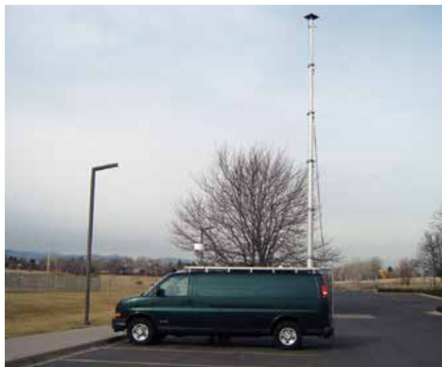
Figure 2 (right). Test van with pneumatic mast deployed for Phase II field measurement of DSA sensor performance.
