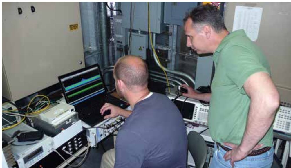
Figure 1 (top). Air Force aircraft (masked in photo) in DOD anechoic chamber during emission measurements. Figure 2. ITS engineer John Carroll and OSM engineer Robert Sole make time-domain recordings of TDWR emissions. Photos by Frank Sanders.
