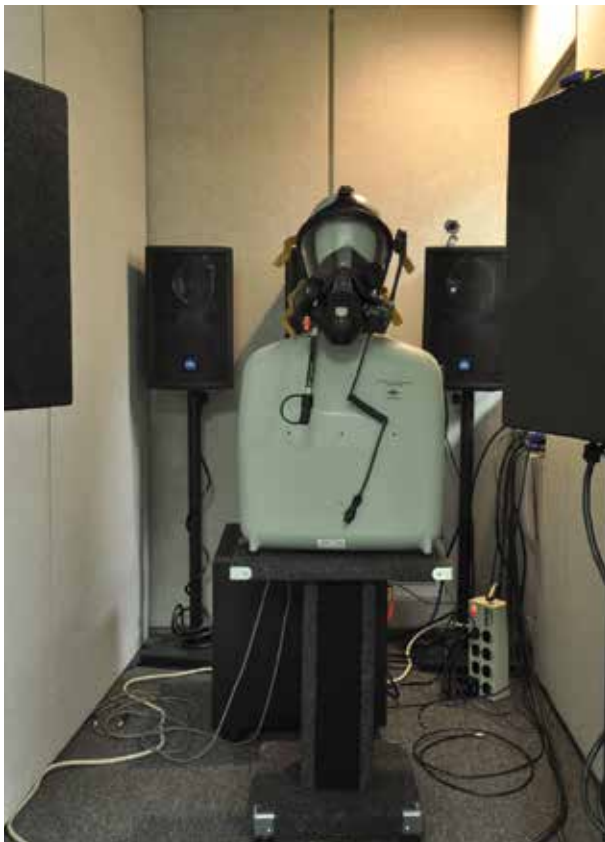
An ITU-Standard Head and Torso Simulator (HATS) is set up in a sound-isolated booth in the Public Safety Audio Laboratory. Loudspeakers behind the HATS are used to reproduce a desired background noise field. Researchers use this set up in a controlled acoustic environment to prepare speech samples for subjective testing. In this way, audio samples used for a subjective audio quality test are identical except for the variables under test. Photo by Andrew Catellier.
