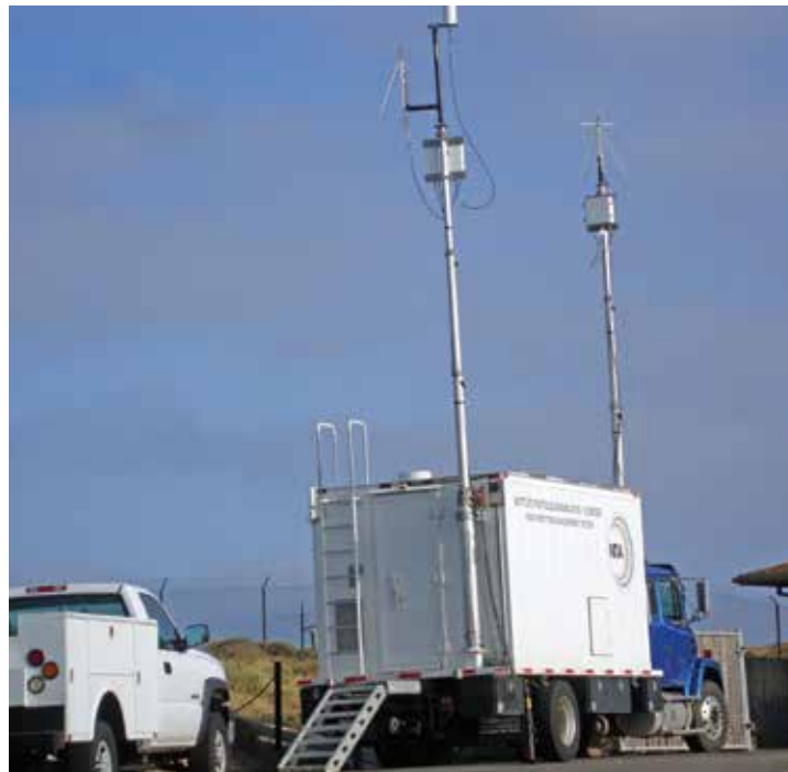
Figure 1 (right). The RSMS-4G vehicle set up to conduct spectrum usage measurements in San Diego, CA. Photo by Chris Hammerschmidt.
