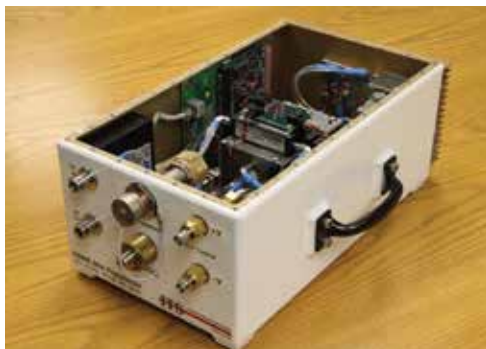
This mini preselector is one of several custom components of the RSMS measurement system designed and built by ITS. Photo by Steve Engelking.
