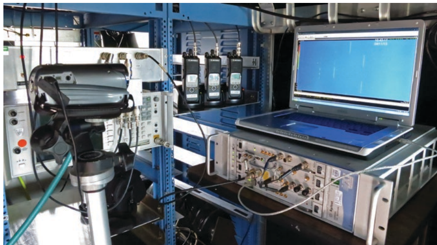
Spectrum monitoring and land mobile radio receiver systems deployed in a test van during Phase III field measurements. Photo by Eric Nelson.
