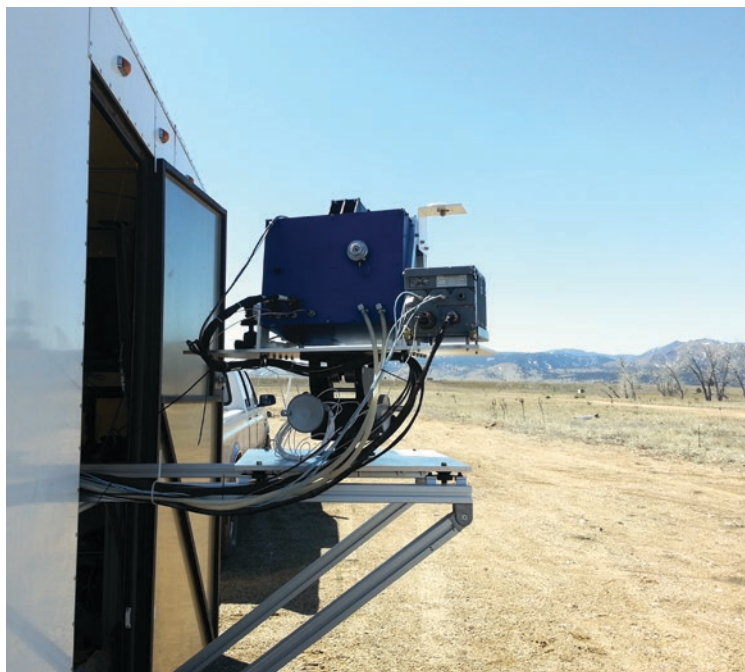
Areté LADAR equipment under development being tested at Table Mountain. Photo courtesy Arété Associates.
