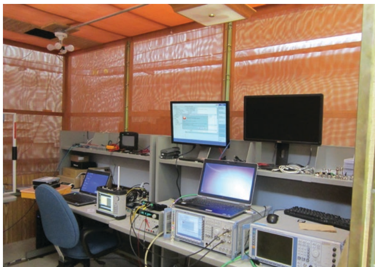
PSCR broadband research laboratory. Upper left: User equipment (UE) from multiple manufacturers in a variety of formats is tested for performance characteristics and interoperability; measurement instruments are on the middle shelf. In the secure area behind the door to the left are eNodeBs from multiple manufacturers for interoperability testing over the air. Above: A bidirectional radio channel emulator is used to develop repeatable air interface testing experiments with different simulation scenarios. Left: A test bench in a screen room for conducting tests in a shielded environment. Photos by Lilli Segre.
