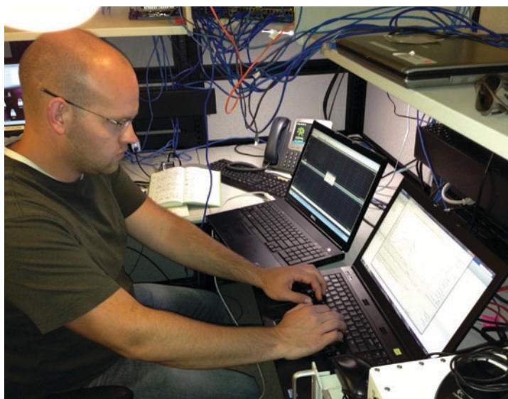
NTIA/ITS engineer John Carroll using a computer-controlled measurement system to gather data on radar-to-LTE interference effects. Photo by Frank Sanders.
