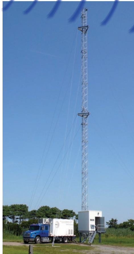
The RSMS mobile measurement laboratory deployed in the field to take radar emission measurements. Photo by Frank Sanders.
