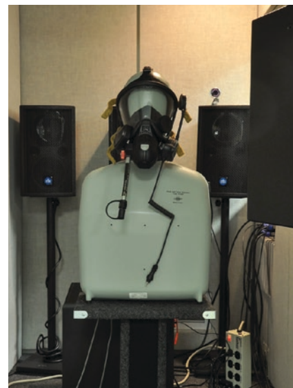
An ITU-Standard Head and Torso Simulator (HATS) set up in a sound-isolated booth for testing in the PSAL. Photo by Andrew Catellier.
