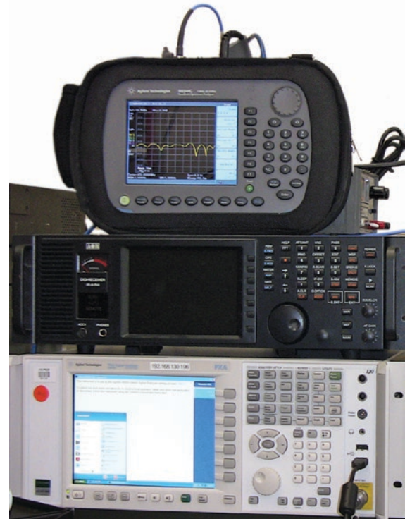
The high precision propagation measurement system in the receiver van was developed by ITS using commercial-off-the-shelf components. Photo by R. Johnk.
