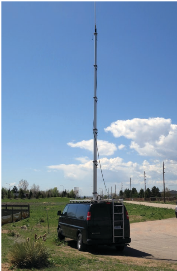
Test van with elevated land mobile radio base station antenna for Phase III field tests of DSA transceivers. Photo by Eric Nelson.
