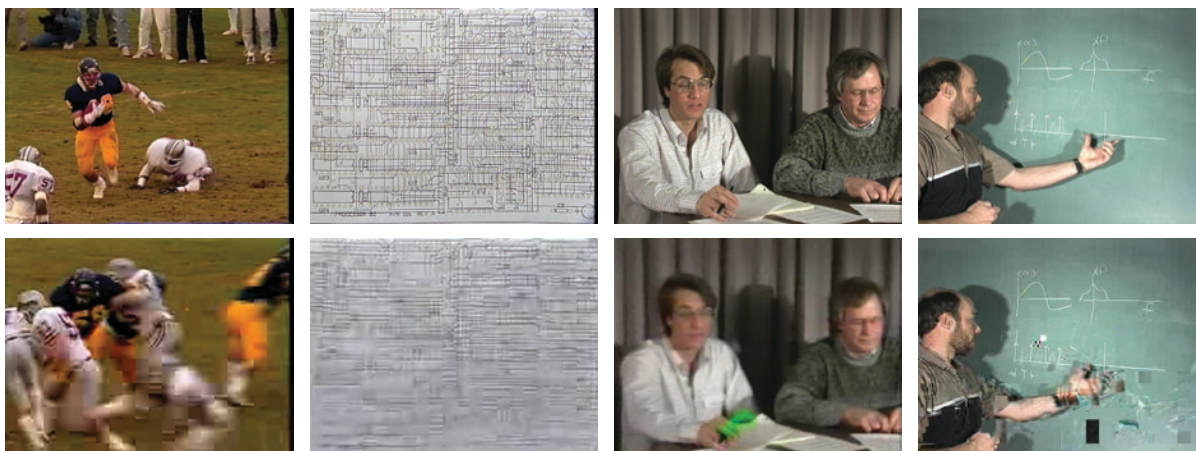
Sample frames from the 1994 ATIS dataset of 25 source video sequences (SRC), all in the public domain, made available on CDVL. Original (top row) and impaired (bottom row) clips include content with high object/camera motion, graphics, more than one person, one person with graphics, and more. Stills courtesy CDVL.
