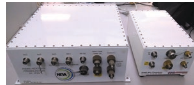
Customized preselectors built by ITS. Photo by John Carroll.
