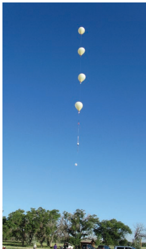
A balloon-borne LTE repeater is deployed to test the feasibility of this technology for emergency communications. Photo by Ken Tilley.
