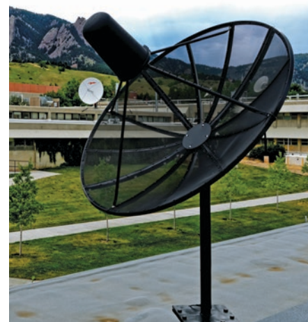
The black satellite base station receiver antenna in the foreground was mounted on the roof of the ITS laboratory for validation testing. Photo by Tim Riley.
