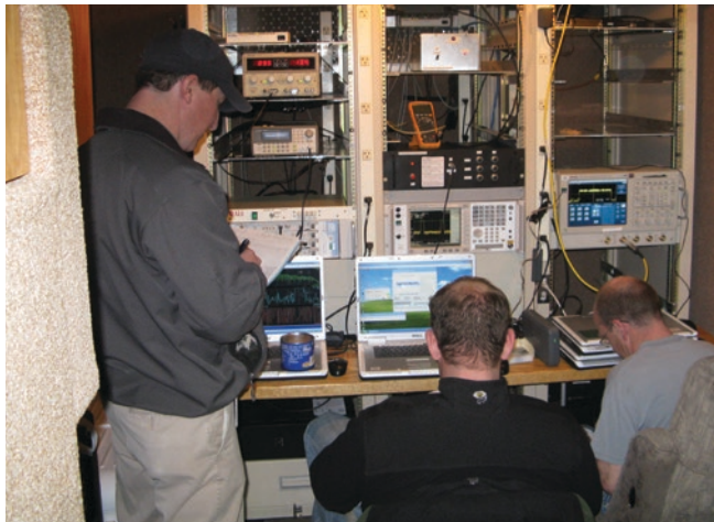
ITS engineers inside the RSMS-4 mobile spectrum measurement laboratory performing and documenting a measurement. Photo by J.R. Hoffman.
