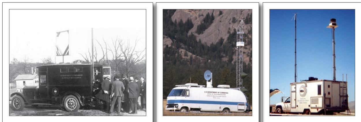
RSMS mobile measurement laboratories through the years. Left, the 1927 Bureau of Standards RF truck; center, RSMS-1 on the Boulder labs grounds in 1970; right, RSMS-3 taking measurements at Fort Irwin, c. 1998 (photo by Frank Sanders).
