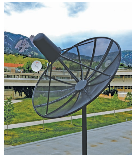
A satellite base station receiver antenna was mounted on the roof of the ITS laboratory for validation testing. Photo by Tim Riley.
