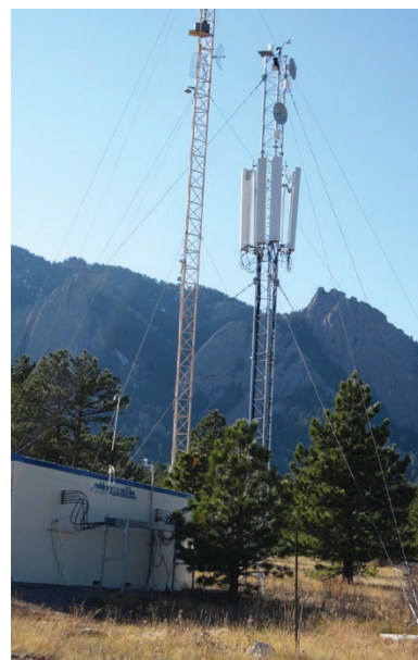
A cluster of antennas used to test different telecommunications technologies at the Green Mountain Mesa Field Site. Photo by Jeff Bratcher.
