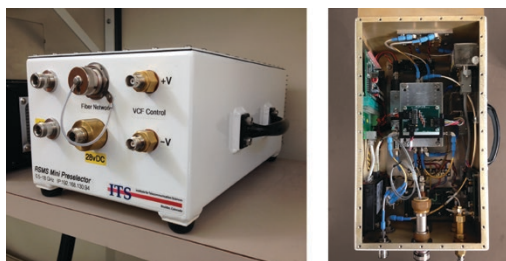
ITS compact RF front end containing noise diode calibration source, wide-range stepped RF attenuator, yttrium iron garnet (YIG) tunable microwave bandpass filter and low-noise amplifiers. Operates at frequencies up to 18 GHz. Photos by Frank Sanders.
