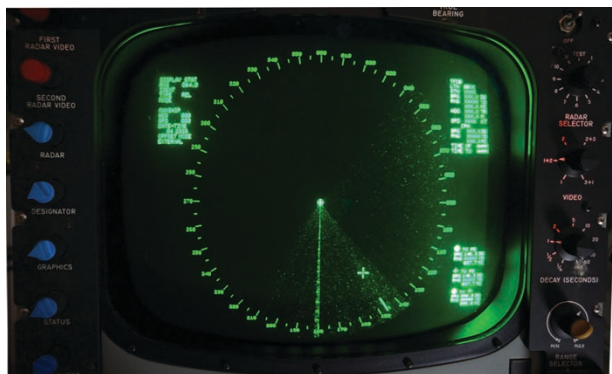
Figure 1. PPI display when Gaussian noise interference is present. The artificially generated targets are visible as regularly spaced bright green tics at 180 degrees bearing.
