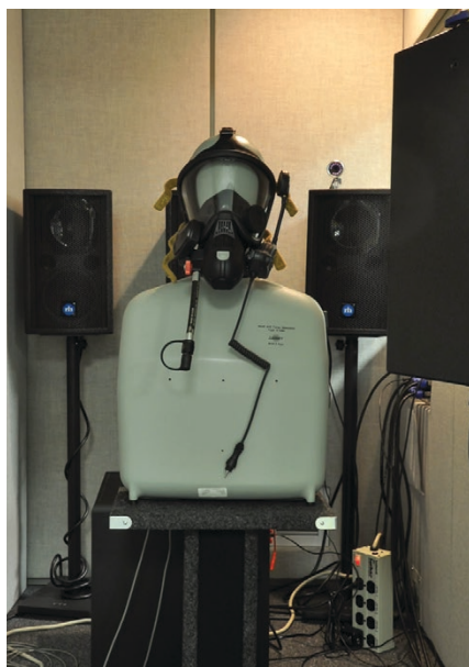
An ITU-Standard head and torso simulator (HATS) set up in a sound-isolated booth for testing in the PSAL. Photo by Andrew Catellier.
