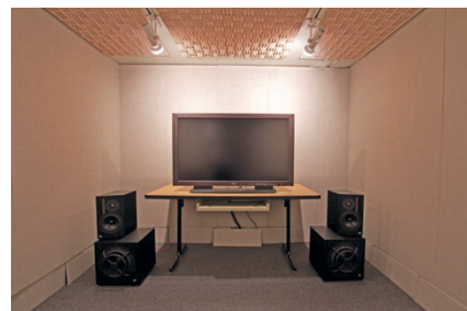
Audio Visual Laboratory facilities at ITS. Top: The video workstation includes a broadcast quality television, studio quality speakers, and uncompressed capture of HDTV. Acoustical foam reduces background noise, so that subtle audio impairments can be heard. Middle: Subjective test room set up as a real world living room. Bottom: Sound isolation booth set up for an audiovisual subjective test, with a broadcast quality television and studio quality speakers. Photos by Andrew Catellier.
