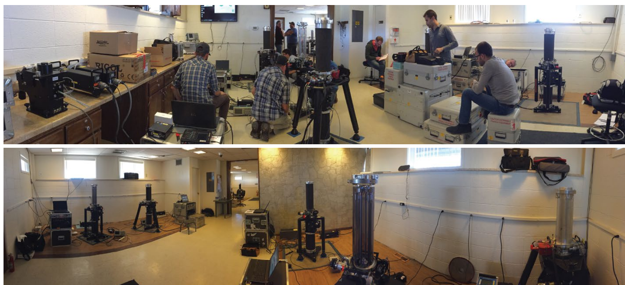
Top: Researchers from Germany, Brazil, Italy, Canada, the Netherlands, Saint Lucia, Luxembourg, and elsewhere brought equipment to set up for the annual “North American Comparison of Absolute Gravity Meters” at the Table Mountain Gravity Observatory. Bottom: The gravimeters in place during testing. Photos by Derek vanWestrum, NOAA.
