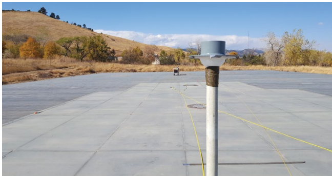
Figure 3. ITS VNA/optical link system deployed on the NIST OATS for propagation measurements. Photo by Bob Johnk.
