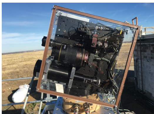
Telescope and gimbal control for a dual-comb laser spectrometer instrument being tested at the Table Mountain Field site by the Applied Physics Division of NIST and University of Colorado to locate and size methane leaks from oil and gas production sites with high precision. Photo by Sean Coburn.
