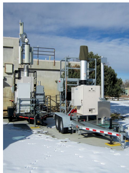
Two cell-on-wheels (COW) units extend the reach of the fixed nodes on the Public Safety Broadband Demonstration Network. Photo by Jaydee Griffith.
