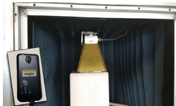
To develop test plans for the widest possible variety of instruments, the first NASCTN project took measurements with a UE hardline connected to the test instrumentation (inset) as well as with the UE placed immediately in front of the aperture of a dual-ridged horn antenna inside a small anechoic chamber. The UE is barely visible as a thick silver line immediately underneath the horn antenna.
