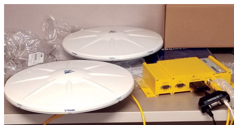
Figure 1. Dual-antenna, multi-constellation GPS receiving system.
