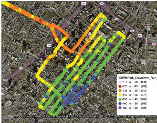
Figure 1. Basic transmission gain along streets in downtown Los Angeles with a transmitting antenna in Griffith Park. Violet dots represent greatest attenuation, pink least attenuation. Satellite imagery courtesy USGS, LAR-IAC Earthstar Geographics SIO © 2016 Microsoft Corporation © 2010 NAVTEQ.
