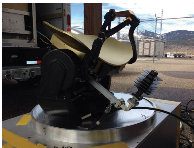
Top: ITS engineer Geoff Sanders measures emissions of a new Ku band airborne radar system at the Table Mountain Field Site. Bottom, the device under test. Photos by Frank Sanders.
