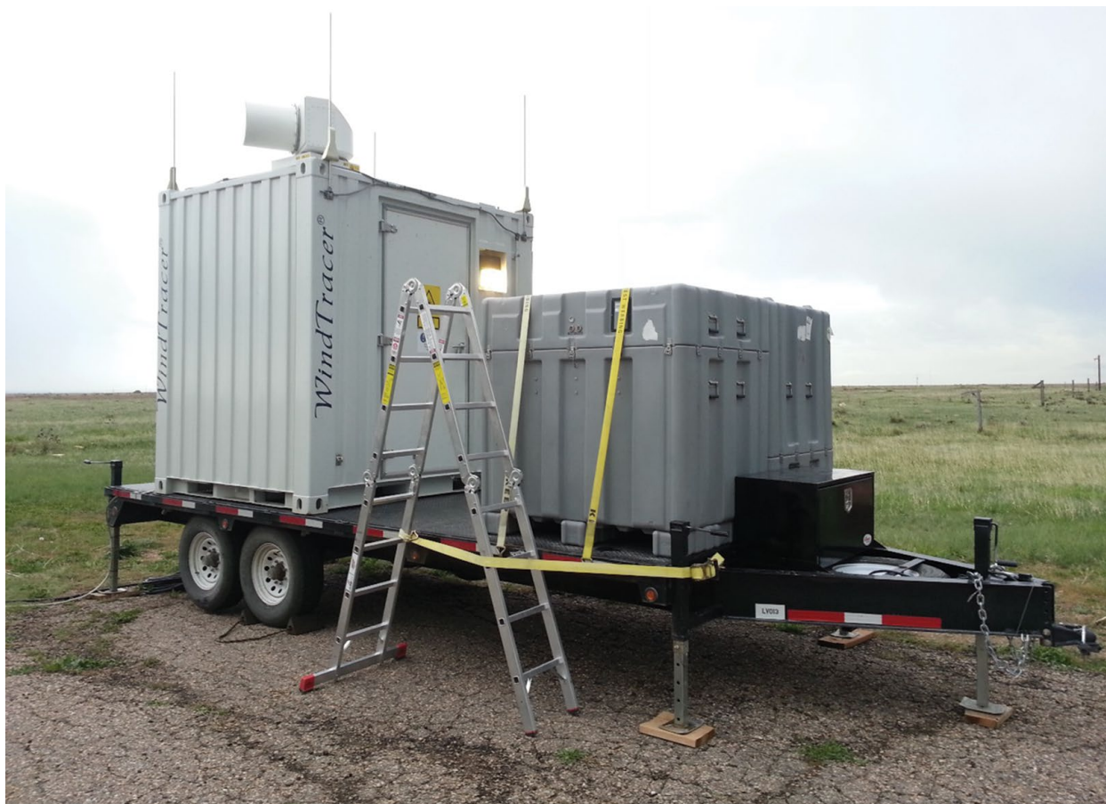
WindTracer® Doppler lidar system being readied for testing at the TMFS. Photo courtesy Lockheed Martin.
