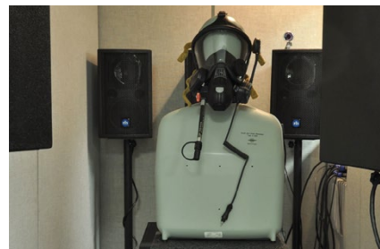
An ITU-Standard head and torso simulator (HATS) set up in a sound-isolated booth for testing public safety communications. Photo by Andrew Catellier.
