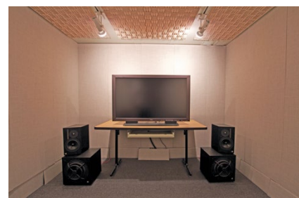
Top: ITS subjective test room set up as a real world living room. Bottom: Sound isolation booth set up for an audiovisual subjective test. Photos by A. Catellier.
