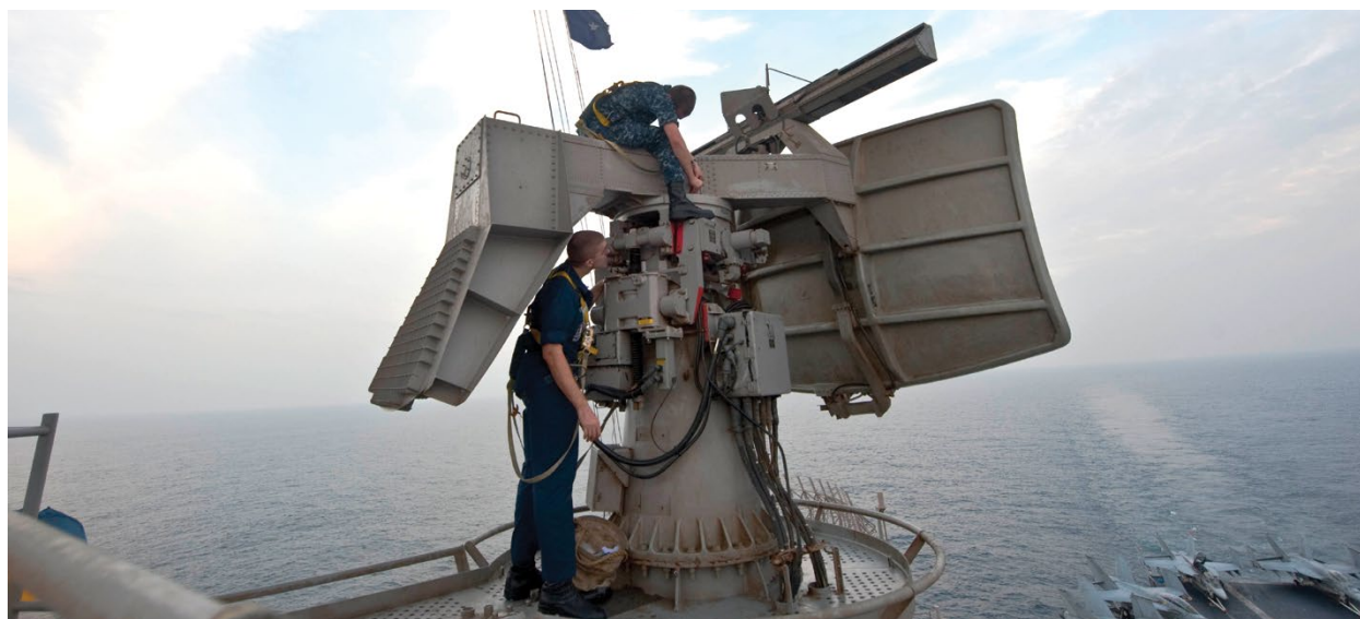
SPN-43 radar aboard the aircraft carrier USS John C. Stennis (CVN 74). Electronics Technician 3rd Class N. Blomgren, top, is performing maintenance (U.S. Navy photo by Mass Communication Specialist 3rd Class W. Tyndall/Released)
