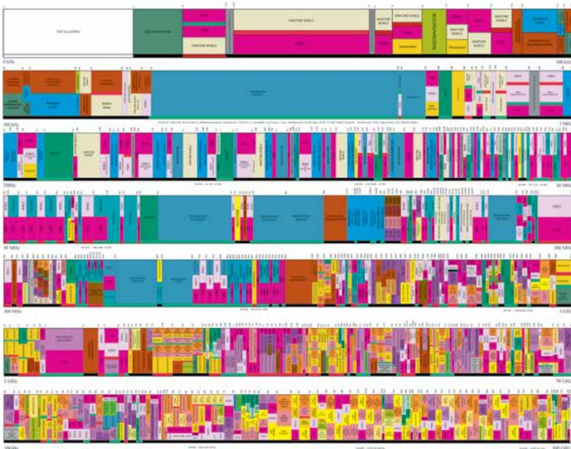
Figure 1 Chart of United States radio spectrum frequency allocations, visually demonstrating the concept of spectrum crowding. The horizontal bands below the allocations show whether frequency bands are reserved for Federal use (red), non-Federal use (green), or shared between Federal and non-Federal users.
