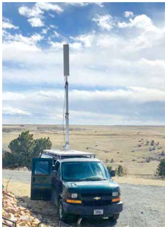
Measurement vehicle with a mast mounted cellular panel antenna collecting aggregate LTE user equipment measurements at a hilltop location near Boulder, CO.
