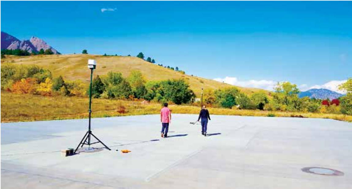
Radiated test setup for channel sounding comparison, located on an open-area test site (OATS) at the U.S. Department of Commerce Boulder Laboratories.
