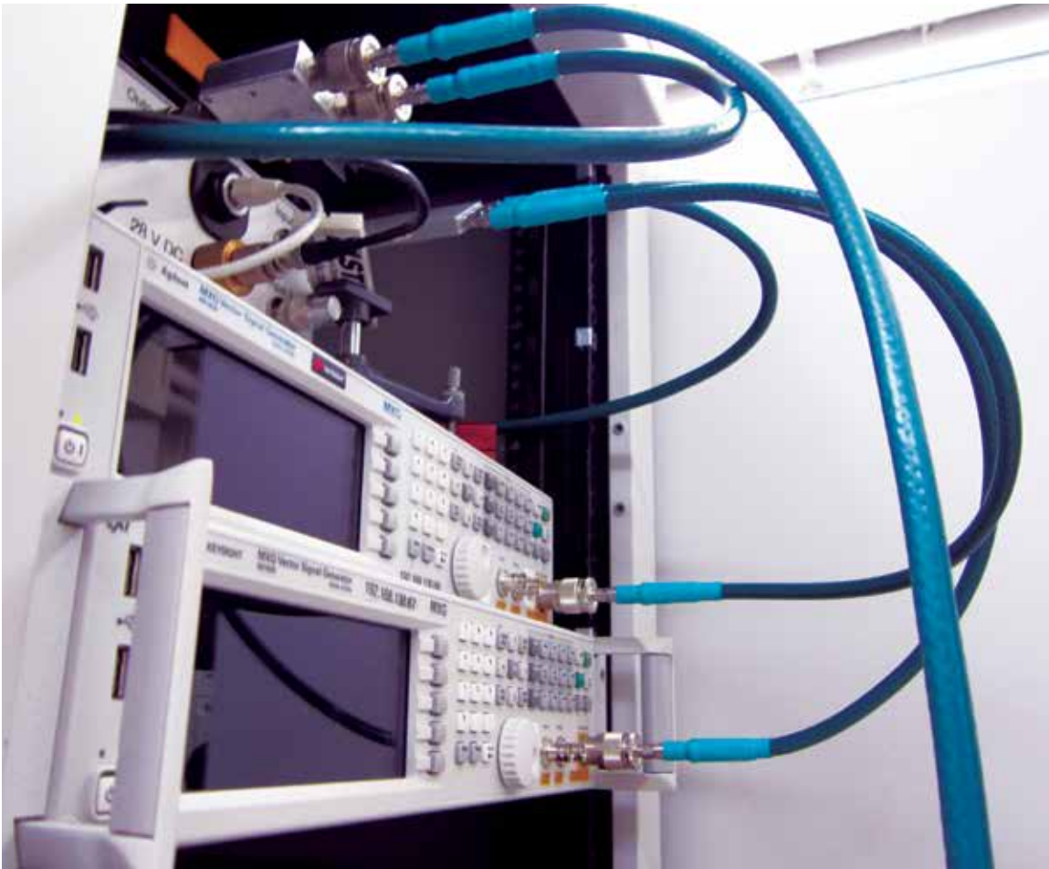
A typical interference protection criteria (IPC) measurement test fixture.
