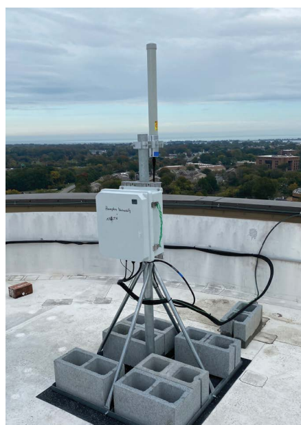
Above left, ITS Principal Investigator Todd Schuman measures antenna S-parameters during installation of a SEA prototype sensor at the Norfolk International Terminal (NIT). Right, top, SEA prototype preselector installed at the top of a NIT tower, with the door open to show internal components; bottom prototype sensor (antenna and preselector) deployed on top of a Hampton University building in Hampton, VA. (Photo credit: Anthony Romaniello)
