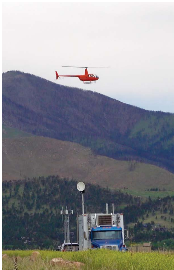
The RSMS-4 measurement vehicle capturing emissions data on a 5G cell on wheels (CoW) while a portable RSMS data-collection system, operated by an ITS engineer, flies in a helicopter at the Table Mountain Federal Advanced Communications Test Site. (Photo credit: Kenneth R. Tilley.)
