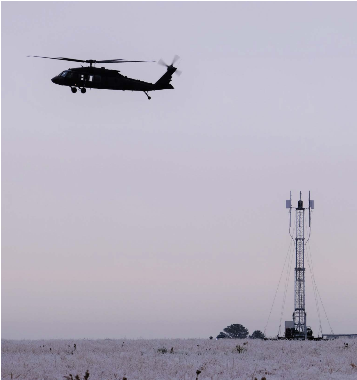
An Army Blackhawk helicopter probes the space surrounding a 5G base station to determine the effects of 5G emissions on an on-board radar altimeter. (Photo credit: Eric Nelson)
