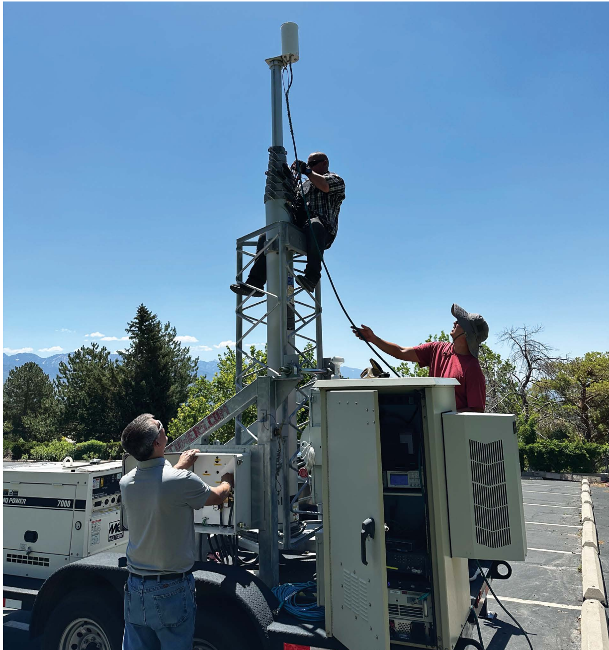
Left to right: ITS engineers James McLean, Kenneth Brewster, and Mike Chang prepare to raise the mast on a CoW to transmit towards downtown Salt Lake City, Utah, in July 2023. This clutter measurement campaign targeting the 3.1–4.2 GHz frequency band supported the 3.5 GHz Propagation Modeling Project. (Photo credit: William Kozma, Jr.)
