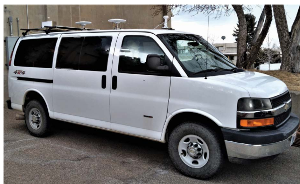
Above top, measurement and data processing equipment racked inside the RSMS-4. Above bottom, measurement van configured as a mobile receiver van for outdoor propagation measurements in the 37–40 GHz band in Boulder, Colorado. Right top, the green van is pictured as configured to transmit a continuous wave 37 GHz signal for the 37–40 GHz band measurement campaign. The fully extended telescoping mast places the transmitting antenna at approximately 10 m above ground level (AGL). Right bottom, CoWs configured for 5G over the air EMC tests at the Table Mountain Radio Quiet Zone.
