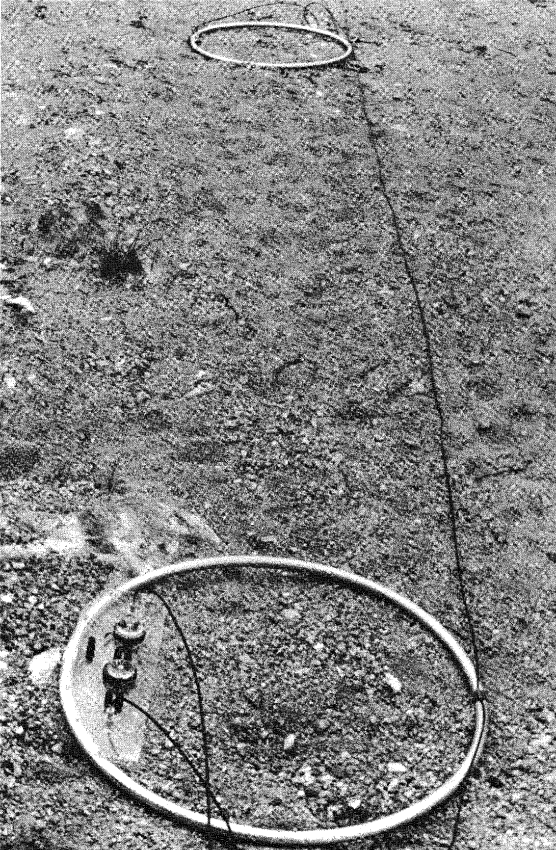
Figure B-2. Conductivity measurement loops in the coplanar orientation on the interface.
