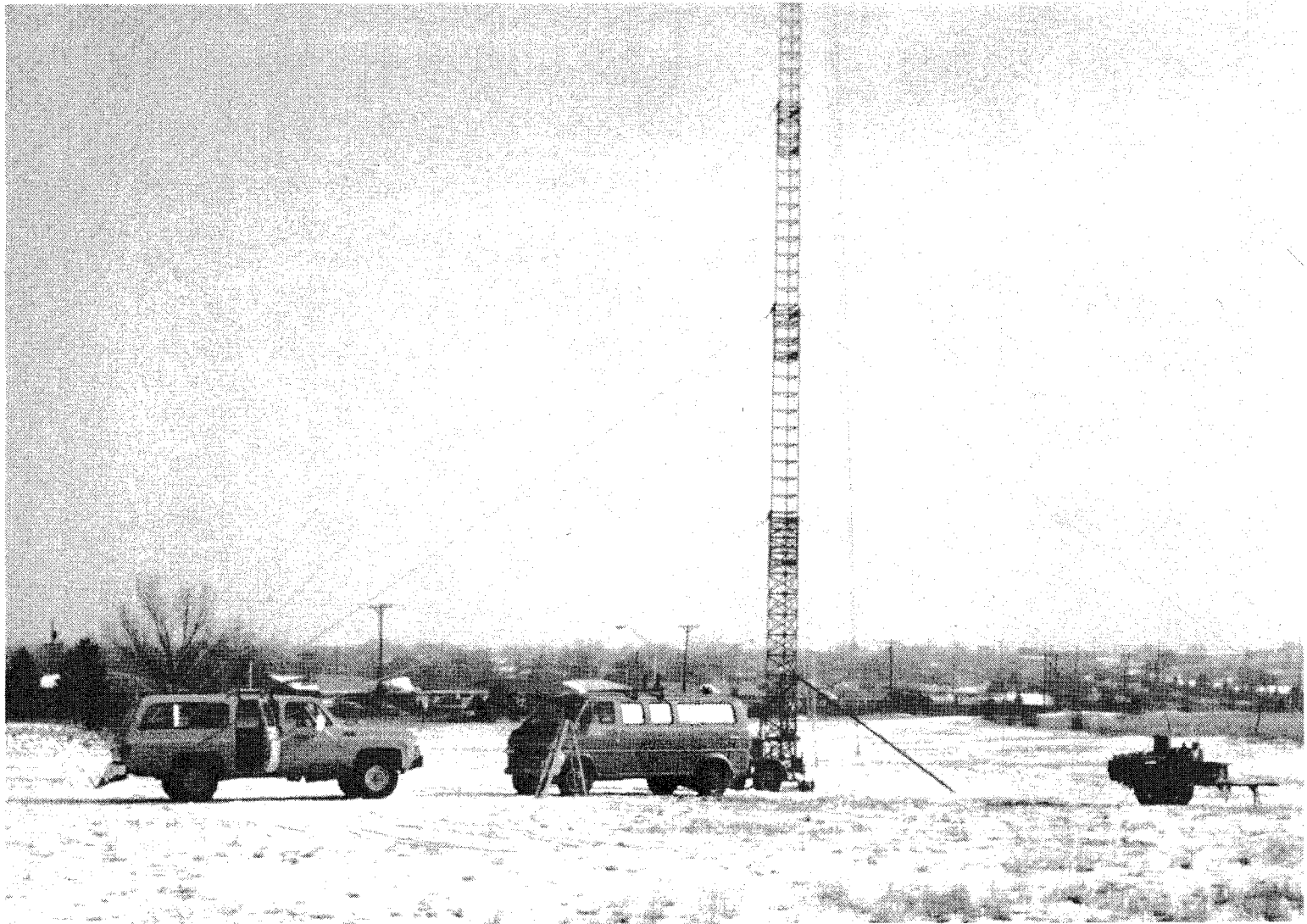
Figure A-1. The receiver and transmitter vans, the erectable tower and diesel generator.
