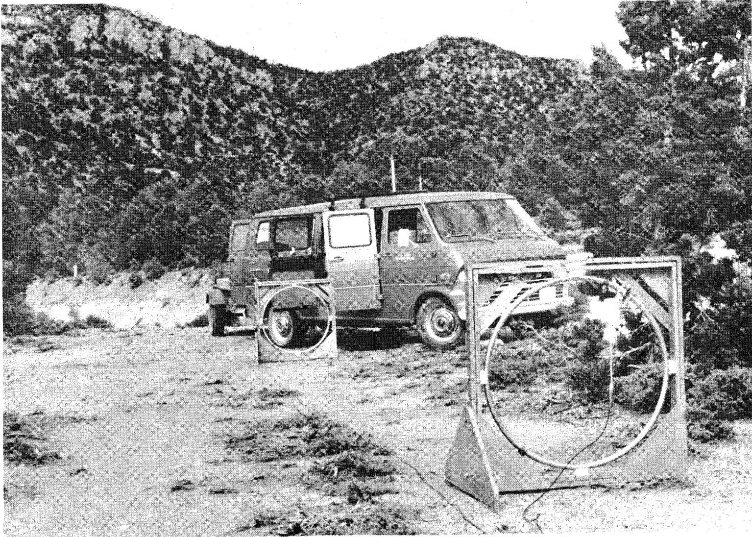
Figure B-3. Conductivity measurement loops in the coaxial orientation.
