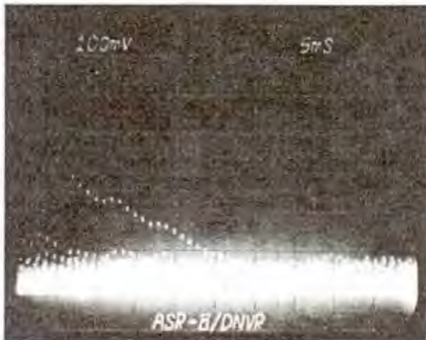
Figure D-27. Measured ASR-8 Integrator Output for Asynchronous MTI Channel Interference
