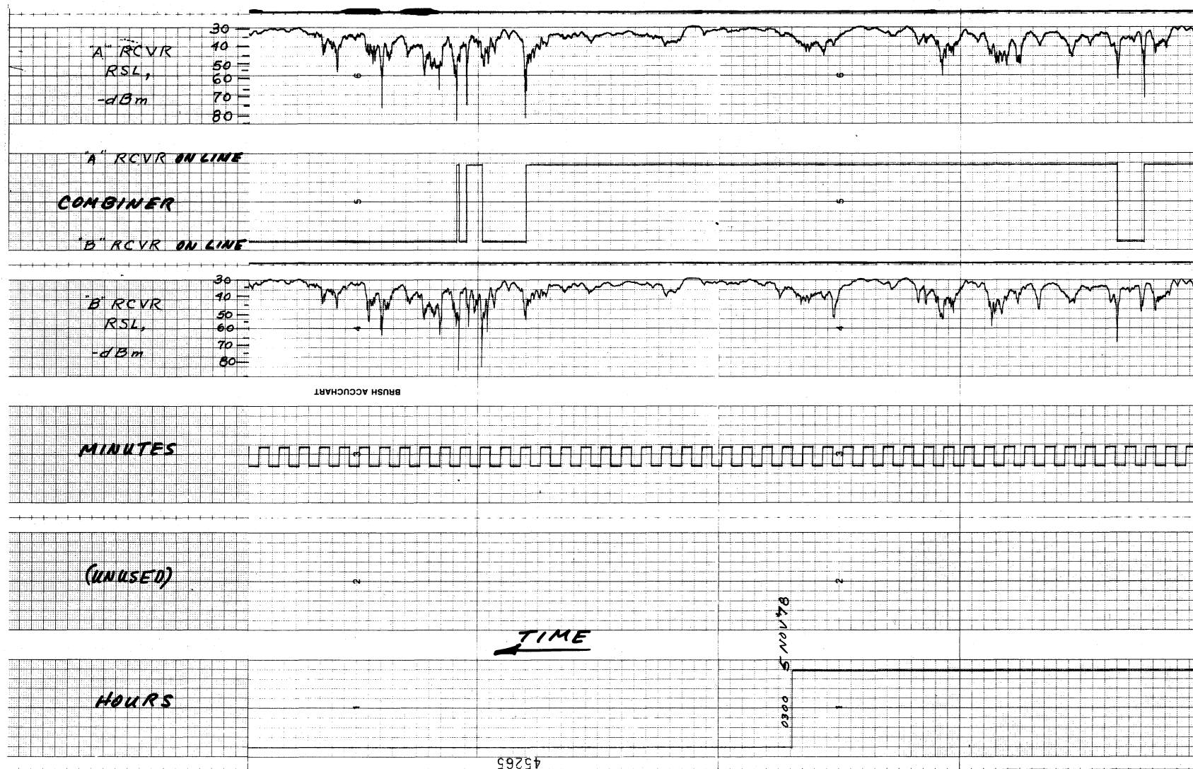
Figure 10. Zugs Spitze recording showing diversity switch activity caused by phase interference fading.
