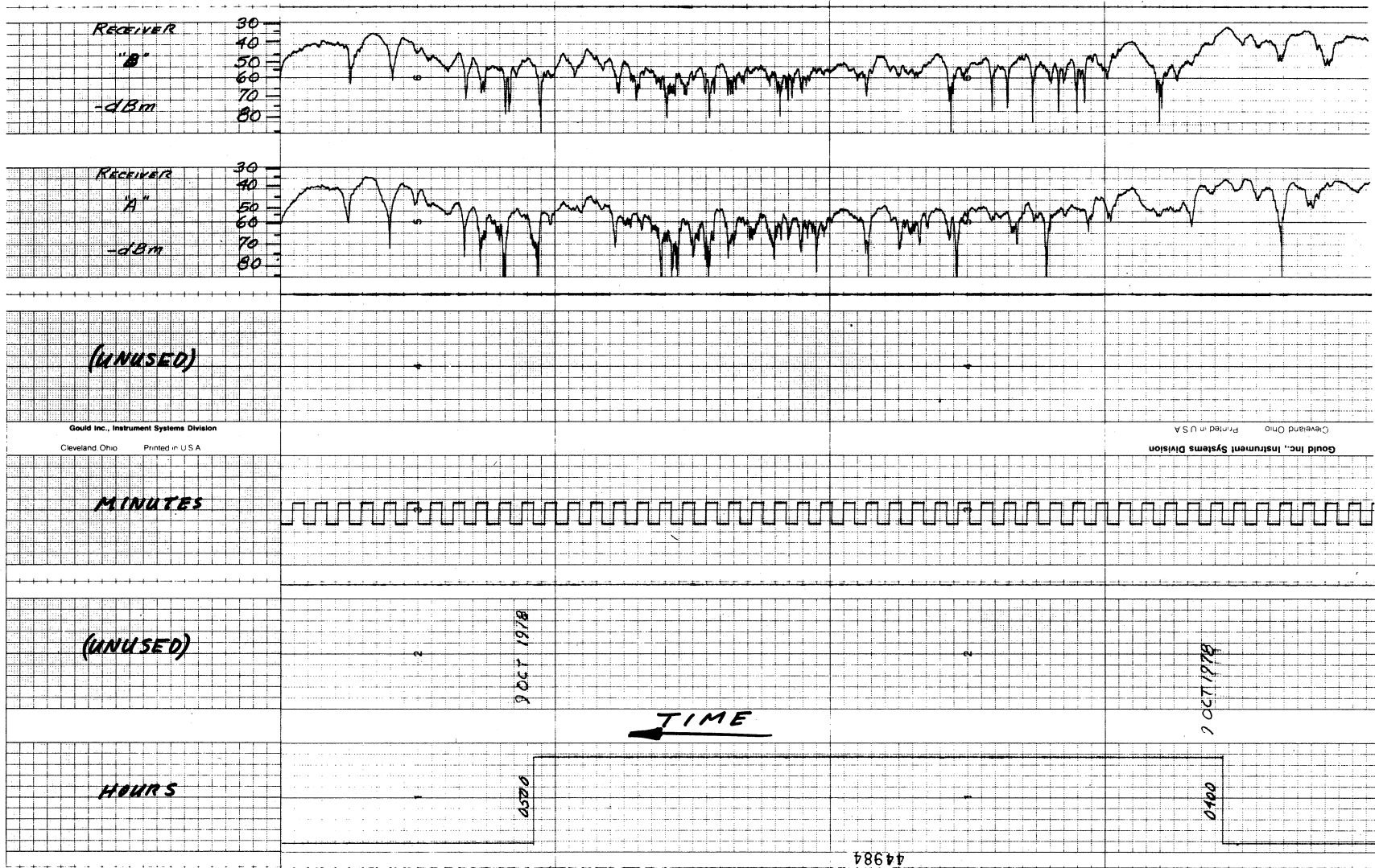
Figure 13. Zugspitze recording showing depressed median signal accompanied by rapid phase interference fading.
