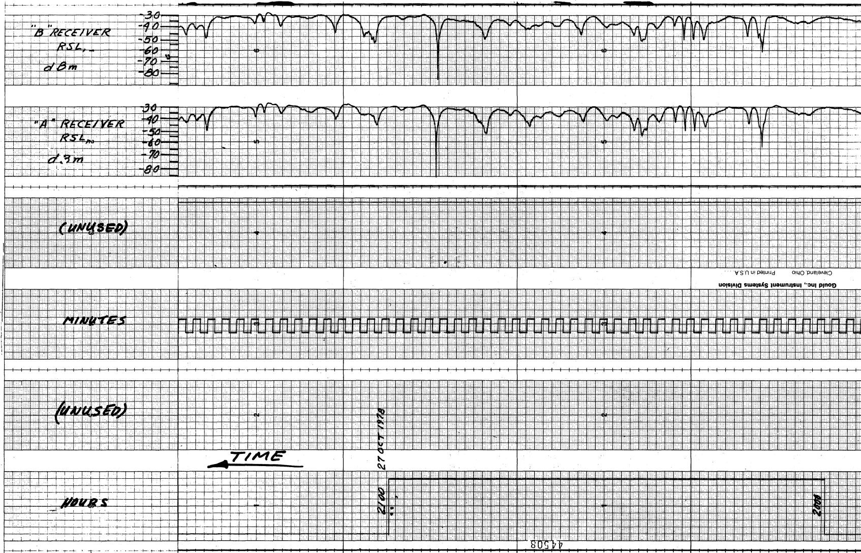
Figure 14. Zugspitze recording showing lack of correlation between very deep fades.
