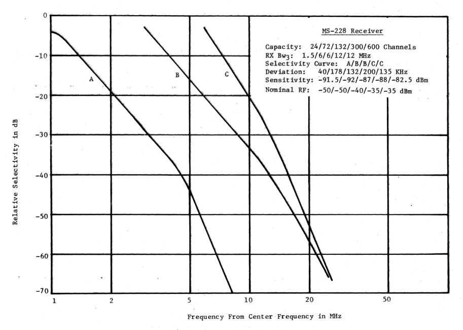
Figure B-3. Parameters for Collins MS-228 Receiver
