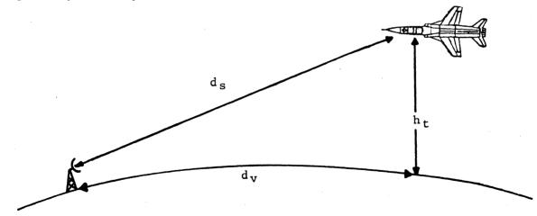
To determine the slant distance,  $d_s$ , at which the interference becomes unacceptable, a criterion will be used that the interference will increase the receiver noise level by not more than 1 dB. For an additive noise-like interfering signal, such as a wideband spread spectrum emission, this point occurs when the power within the receiver passband is approximately 6 dB below the receiver noise level. This can be expressed as follows:
