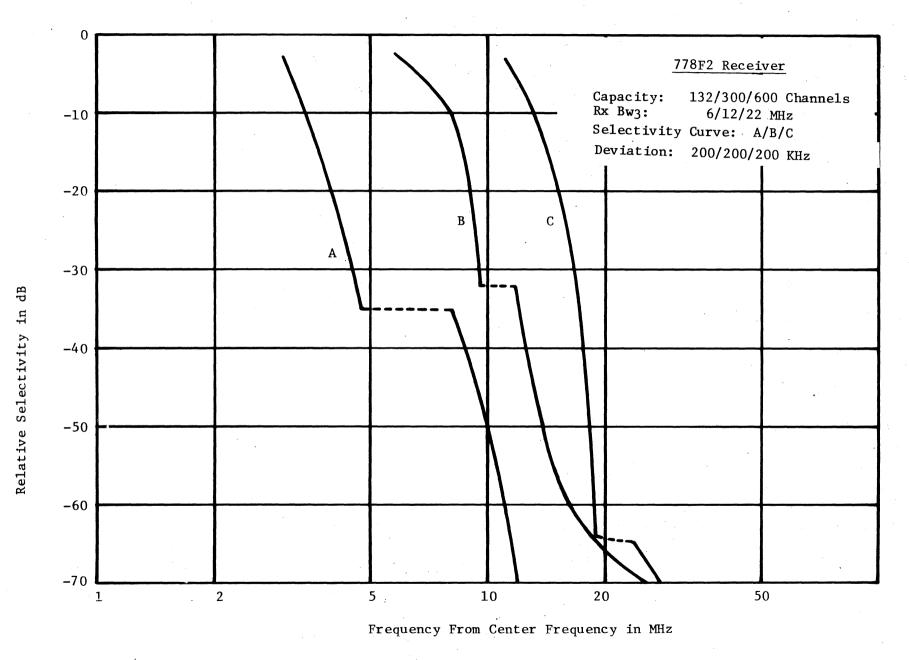
Figure B-4. Parameters for Lenkurt 778F2 Receiver
