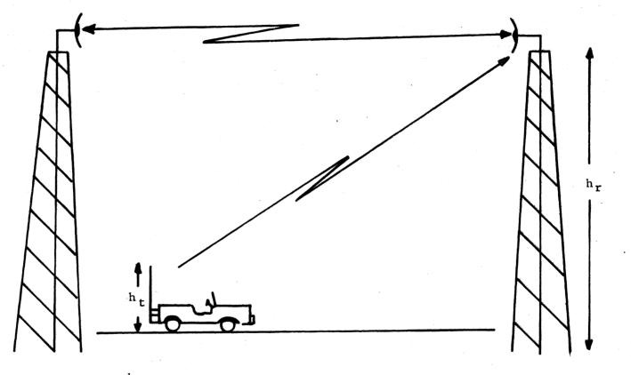
h t = Packet Radio Transmitting Antenna Height
