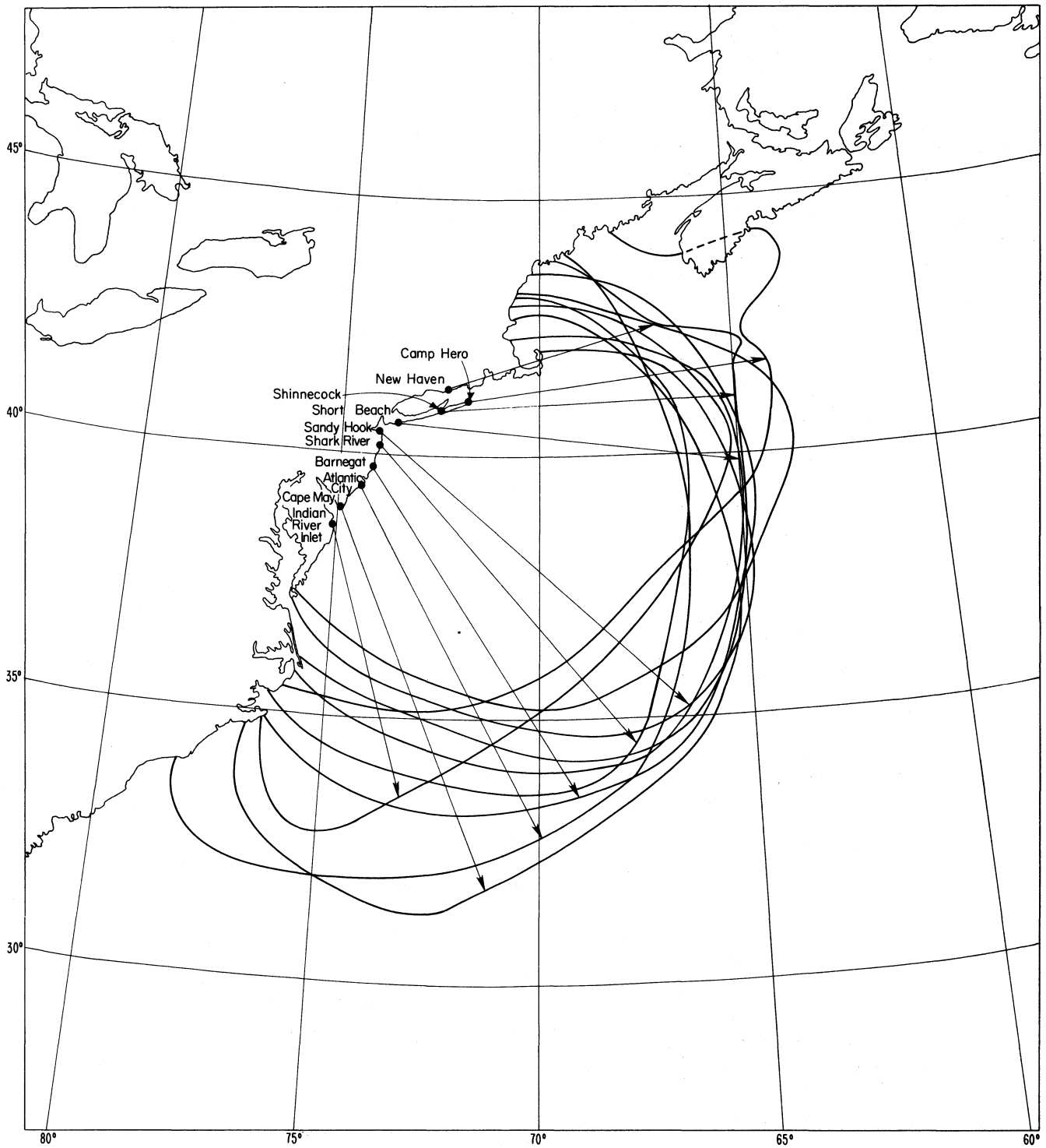
Figure 7. 2182 kHz coverage for District 3, minimum noise.
