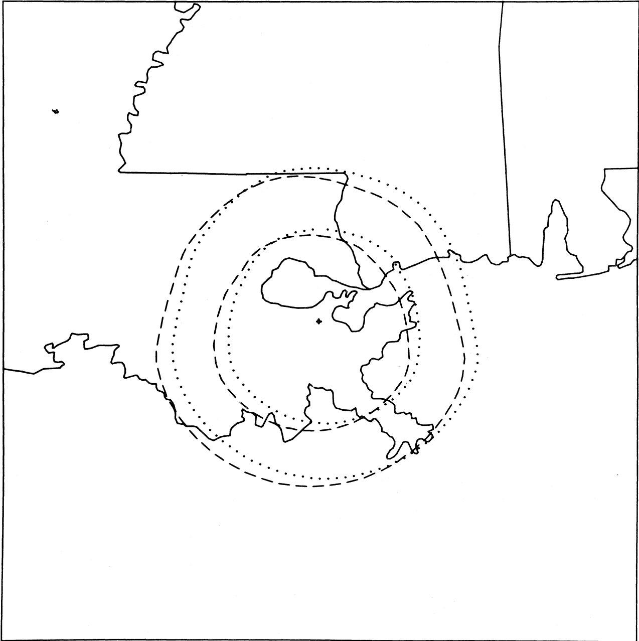
Figure 81. VHF coverage for the District 8 station at Chalmette (60°, dots; 240°, short dashes). Center: 29°57'13"N, 89°57'32"W.
