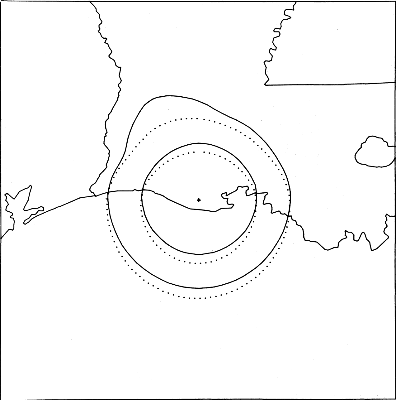
Figure 85. VHF coverage for the District 8 station at Pecan Island (5°, solid; 185°, dots). Center: 29°41'33"N, 92°30'12"W.
