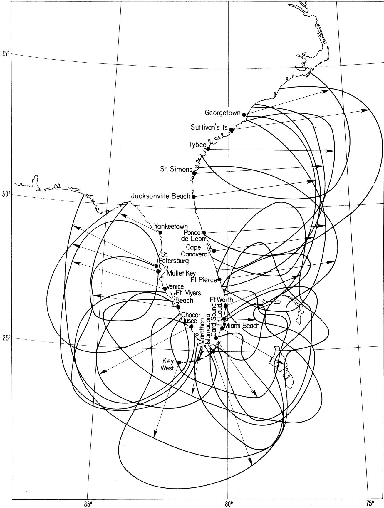
Figure 10. 2182 kHz coverage for District 7, maximum noise.
