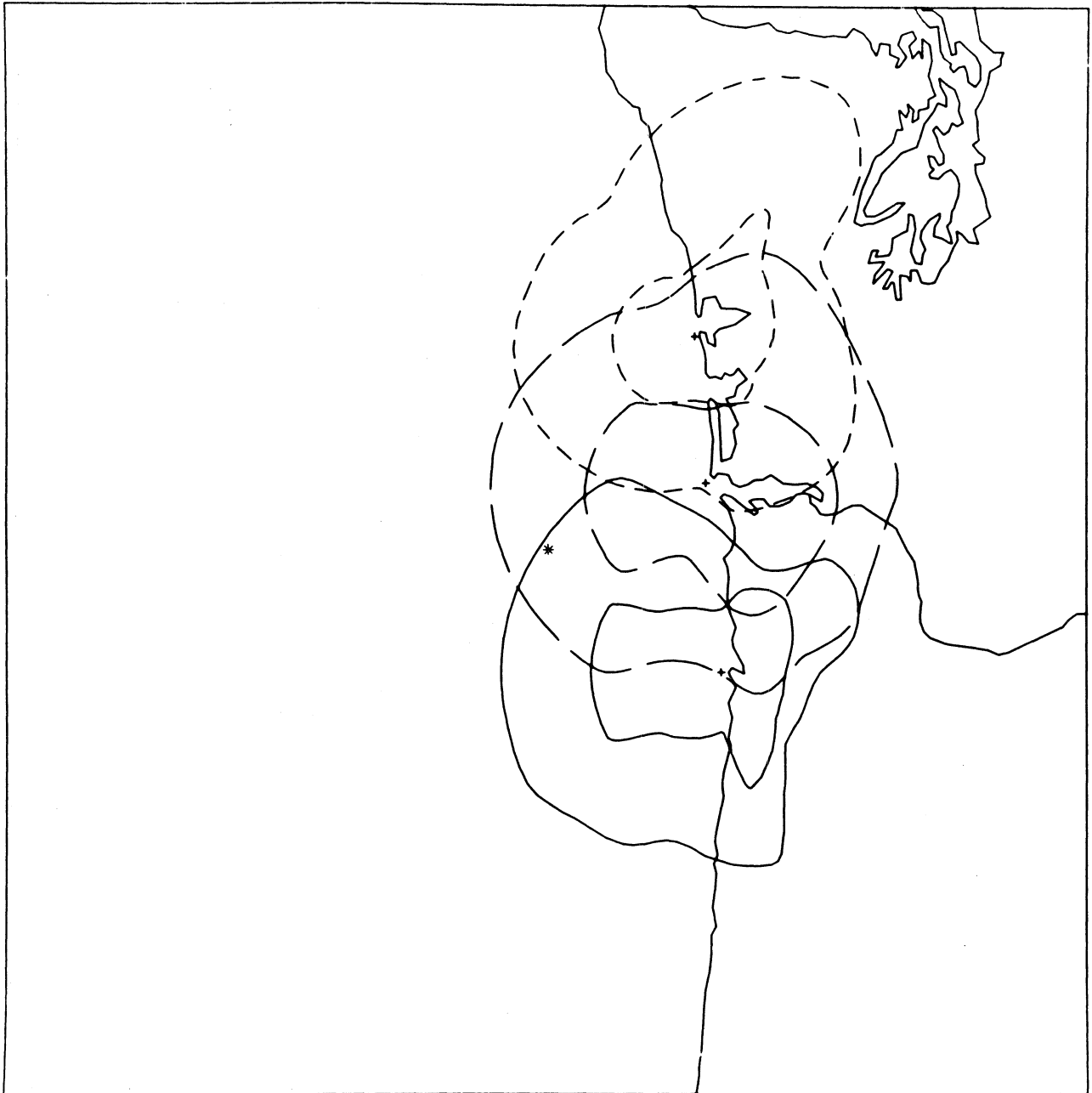
Figure 110. VHF coverage for the District 13 station at Grays Harbor (short dashes), Cape Disappointment (long dashes), and Cape Mears (solid). Center: 46^{\circ}0'0''\text{N} , 125^{\circ}0'0''\text{W} .
