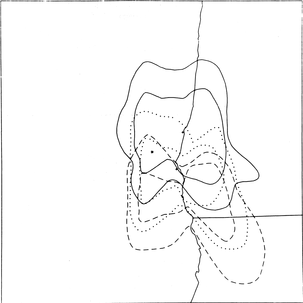
Figure 112. VHF coverage for the District 13 station at Sun Devils (solid), Port Orford (dots), and Cape Sebastian (short dashes). Center: 43^{\circ}0'0''\text{N} , 125^{\circ}0'0''\text{W} .
