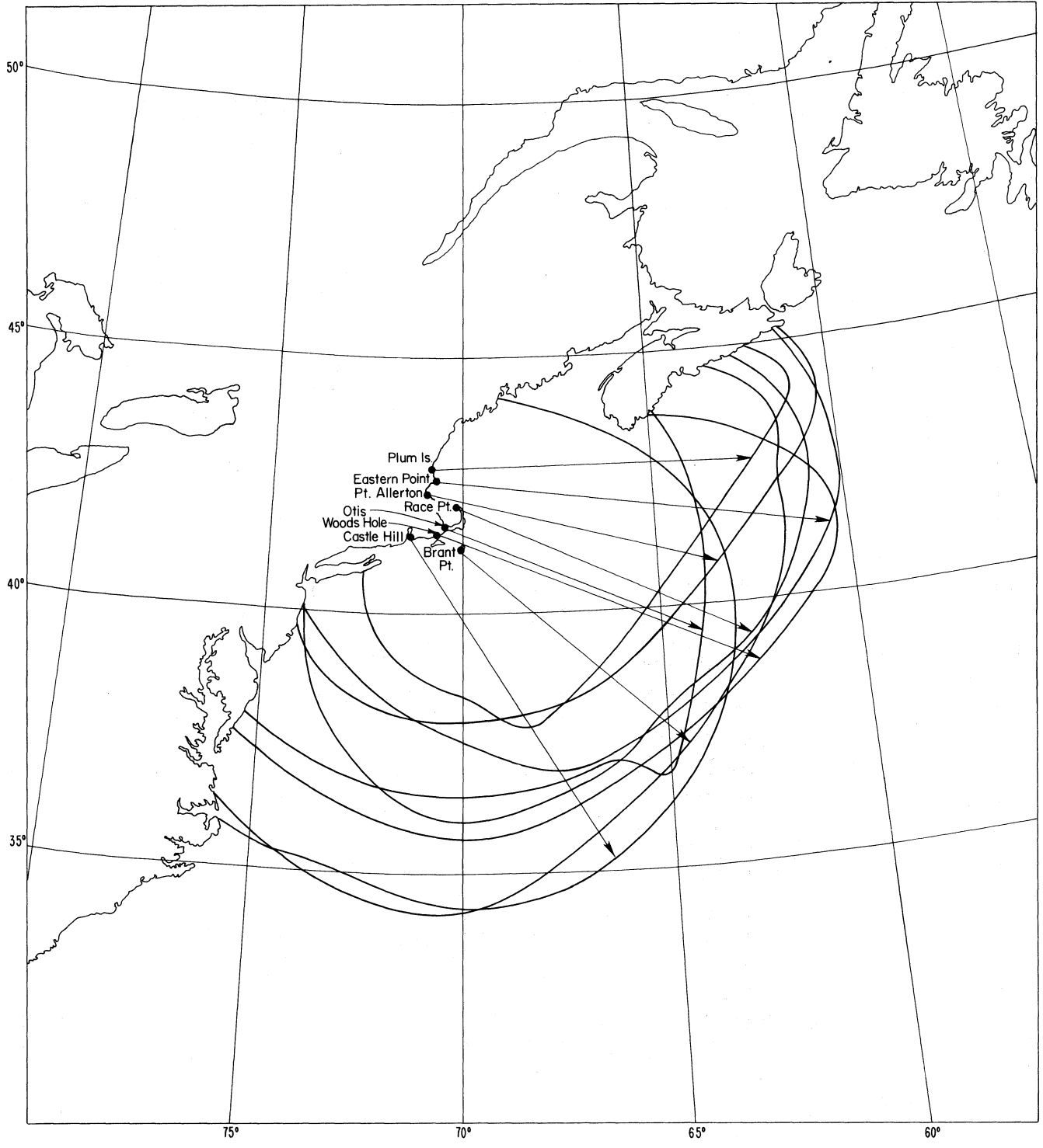
Figure 5. 2182 kHz coverage for the southern portion of District 1, minimum noise.
