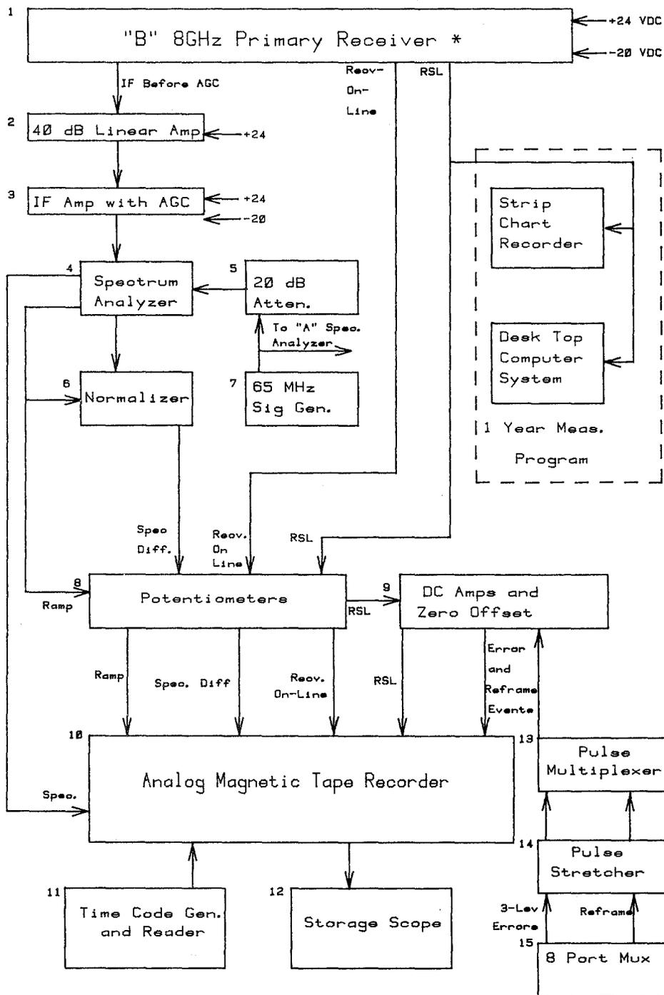
\*This diagram shows the instrumentation for the "B" recv.
