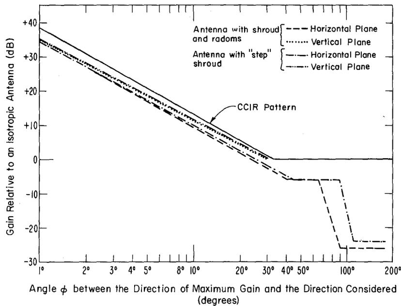
Figure 14. Radiation patterns of two typical parabolic dish antennas in the 7125-7750 MHz frequency range (Colavito and Masone, 1973, p. 11-6).
