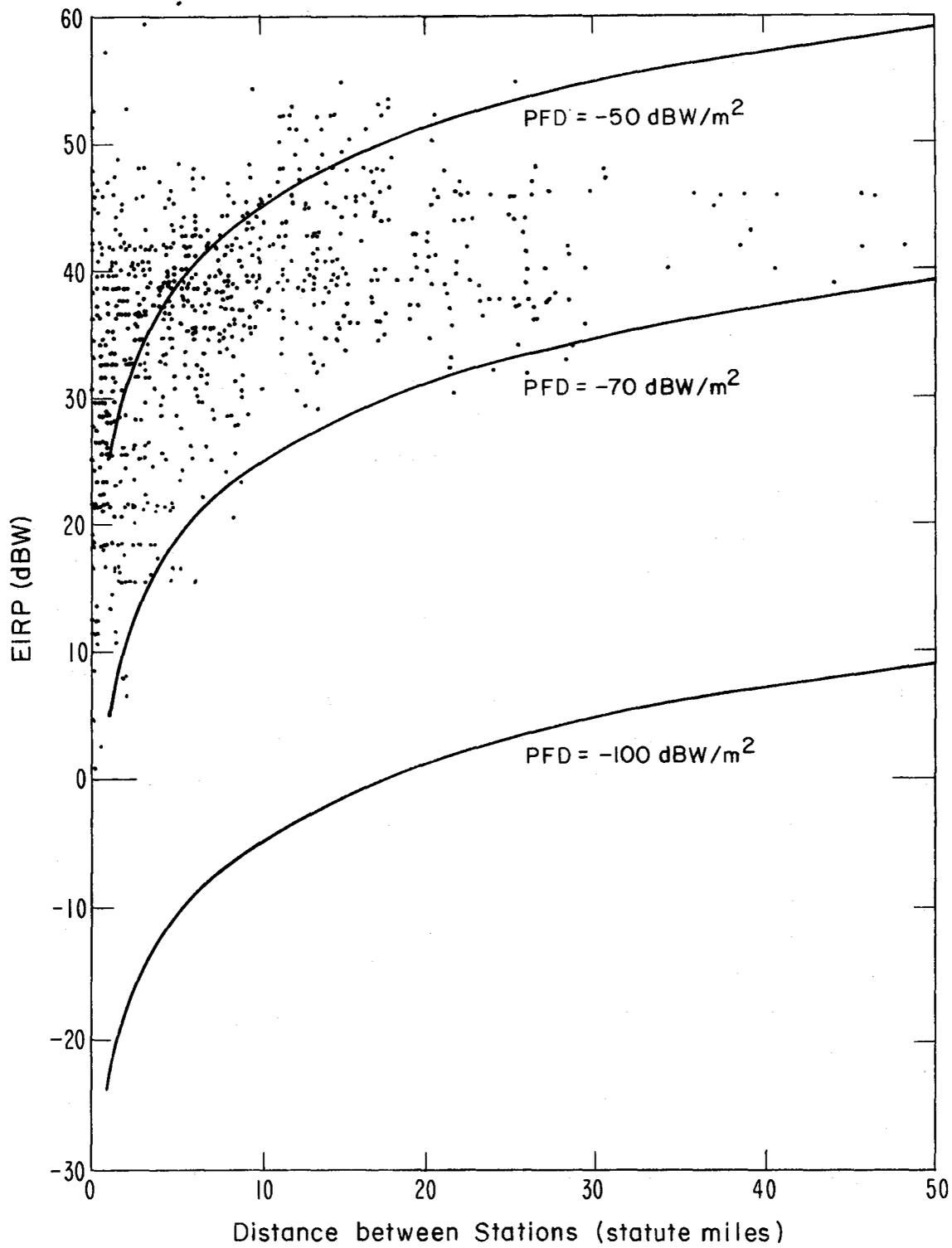
Figure 18. United States FS system operating levels roughly bounded between  $-50$  and  $-70$   $\text{dBW}/\text{m}^2$  PFD compared with the BSS PFD on the surface of the earth at  $-100$   $\text{dBW}/\text{m}^2$ .
