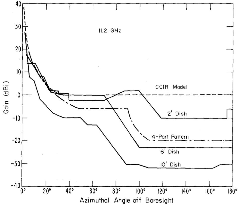
Figure 12. Radiation patterns of typical parabolic dish antenna in the 10.7 to 11.7 GHz range.
