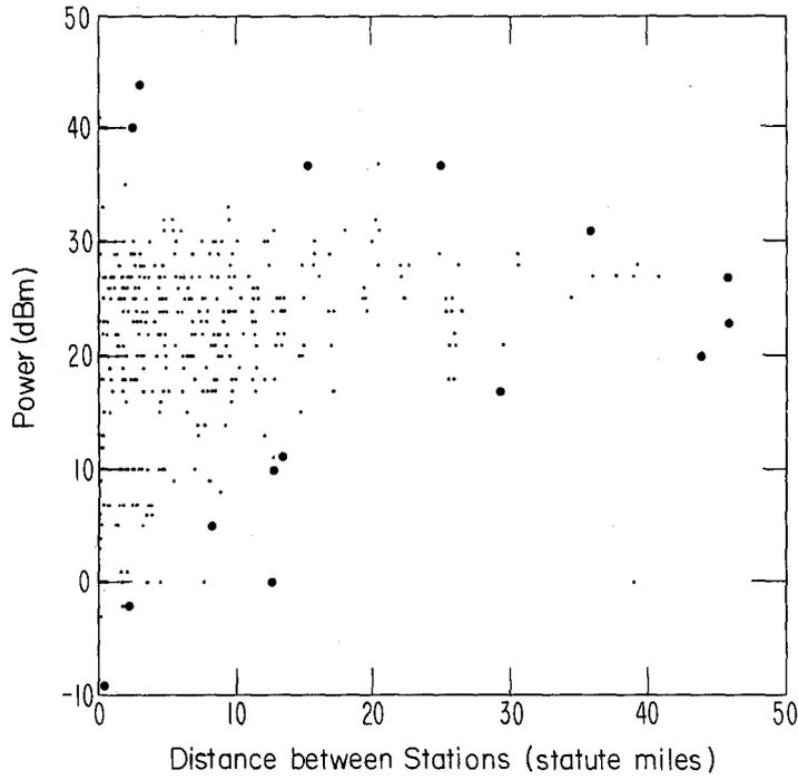
Figure 16. Station distance and transmitter power scatter diagram of 1529 FS transmitters in the United States.
