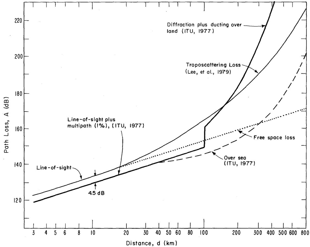
Figure 20. The terrestrial propagation path loss as a function of distance.
