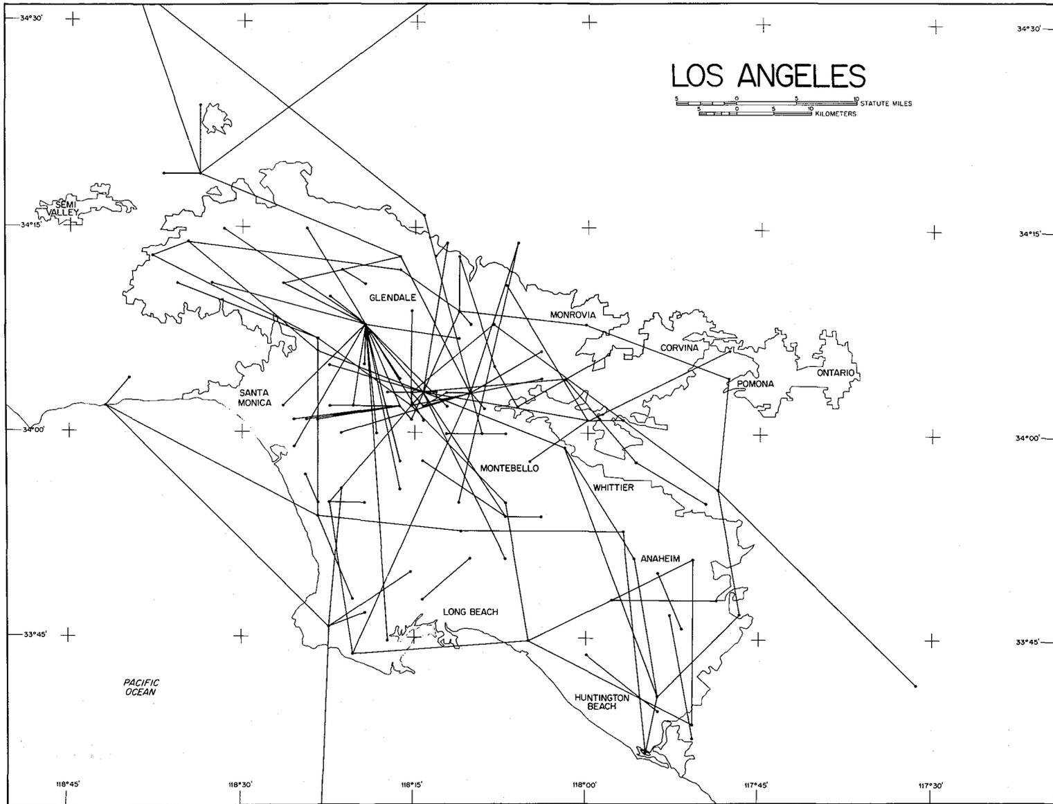
Figure 8. Terrestrial FS user connectivity for the 12.2-12.7 GHz band in the greater Los Angeles Area.
