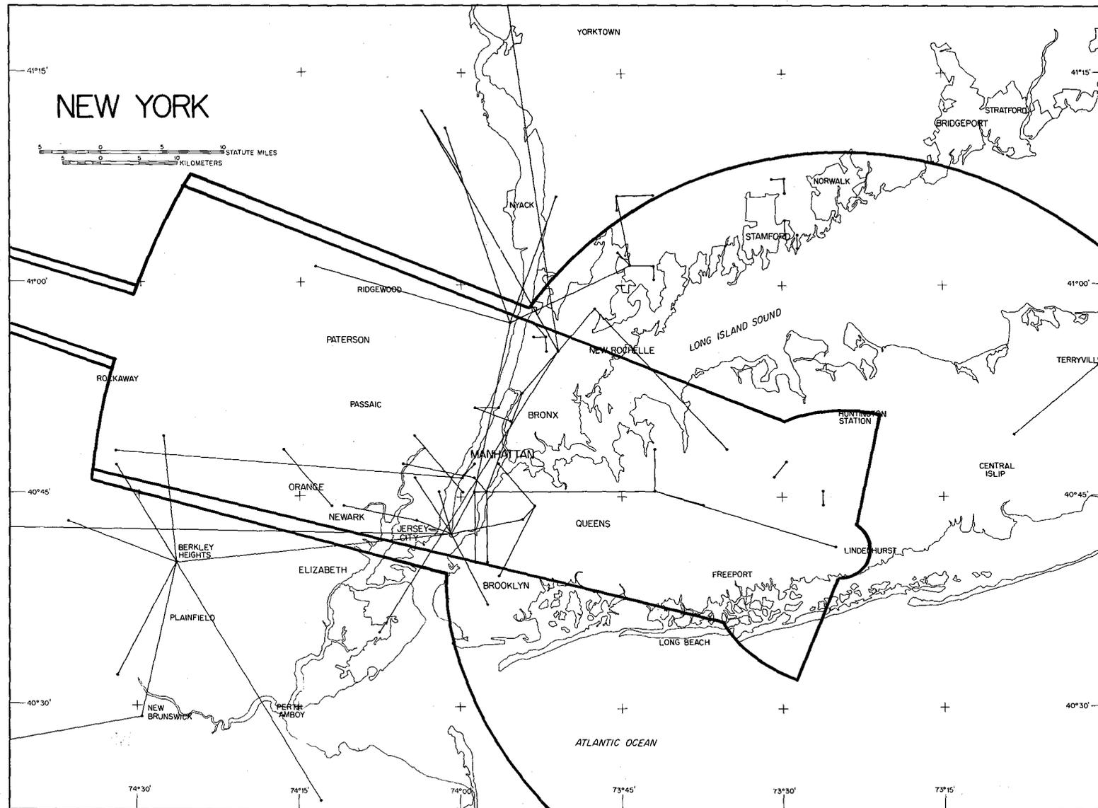
Figure 22. Co-channel interference contours overlaid on New York City. Inside contour derived from four-part pattern, outside contour derived by Akima (1980) using CCIR standards.
