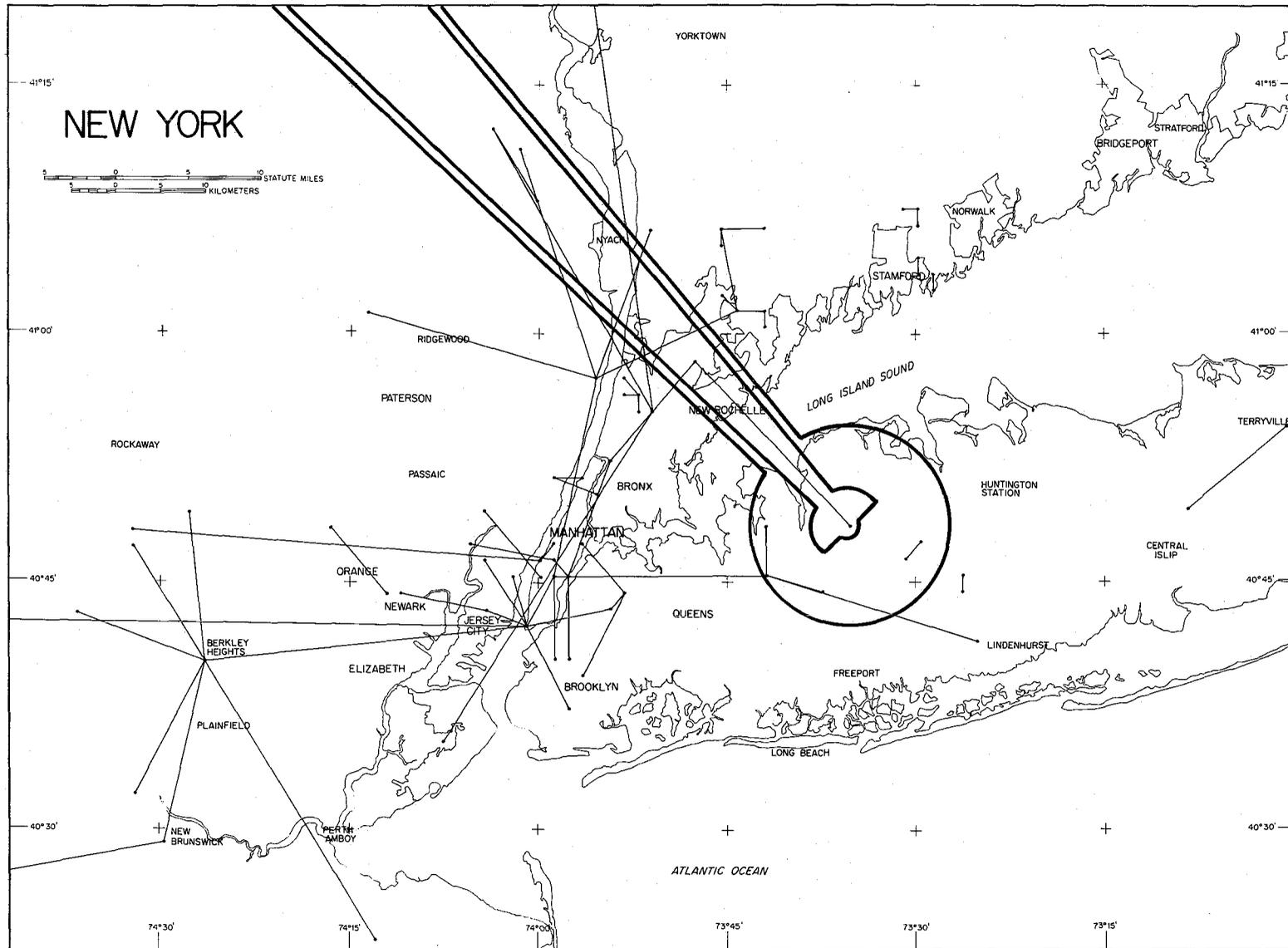
Figure 23. Adjacent-channel interference contours overlaid on New York City. Inside contour derived from four-part pattern, outside contour derived by Akima (1980) using CCIR standards.
