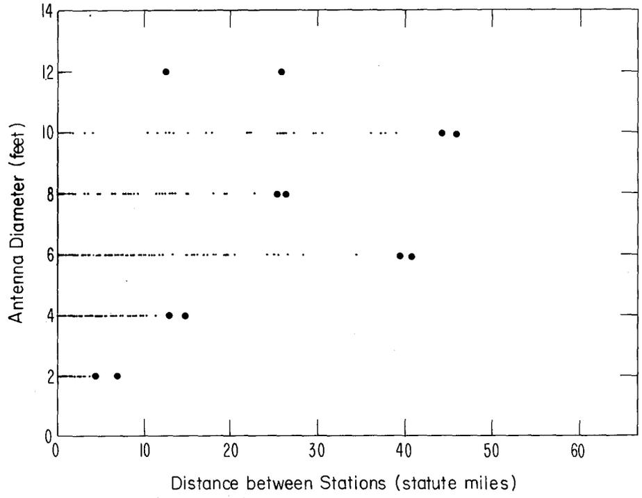
Figure 11. Scatter diagram of United States deployed FS antenna systems as a function of distance between transmitter and receiver versus antenna diameter.
