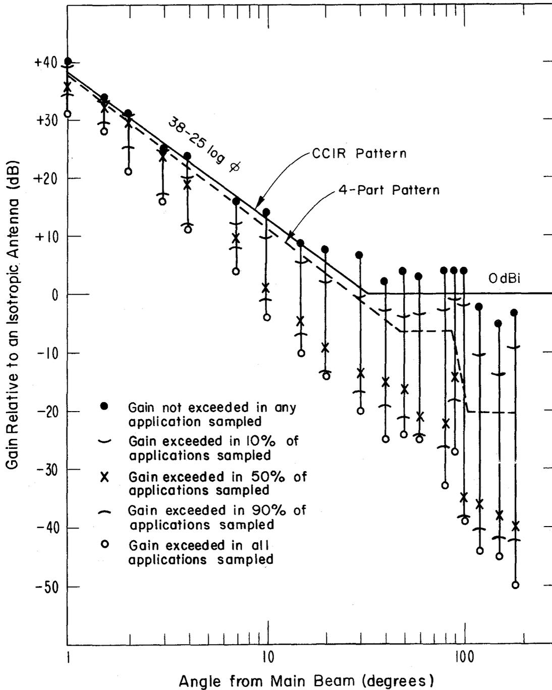
Figure 13. Distribution of horizontal plane gain for line-of-sight radio-relay antenna (CCIR, March 21, 1972, Radiation Diagram of Line-of-sight Radio-Relay antennae For Use In Interference Studies With Communications Satellite Earth Stations, Study Programme 17A/19, Doc. 9/38-E, p. 7).
