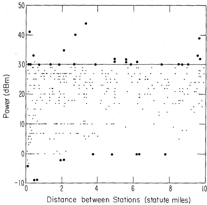
Figure 17. Expanded station distance and transmitter power scatter diagram of 881 FS transmitters in the United States.
