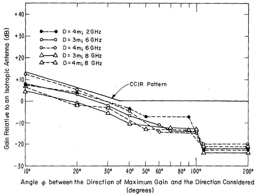
Figure 15. Radiation patterns of some parabolic dish antennas (from 2 GHz to 8 GHz) (Colavito and Masone, 1973, p. 11-6).
