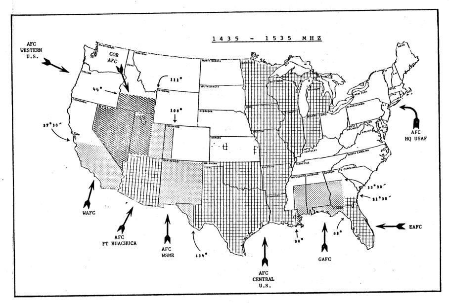
Figure 1. Area Frequency Coordination Responsibility (Extracted from Annex D of the NTIA Manual)
