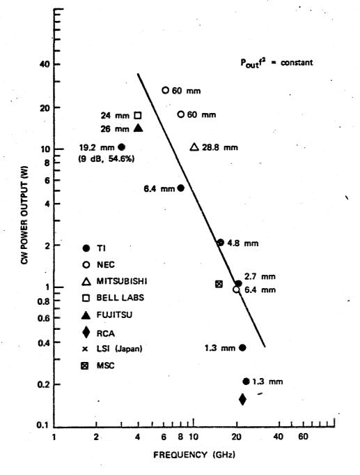
Figure 7. GA FET power output versus frequency. From H.G. Tserng, "Advances in Microwave GA Power FET Devices and Circuit Technology," 1981 European Microwave Conference, London. State of the art as of September 1981.
