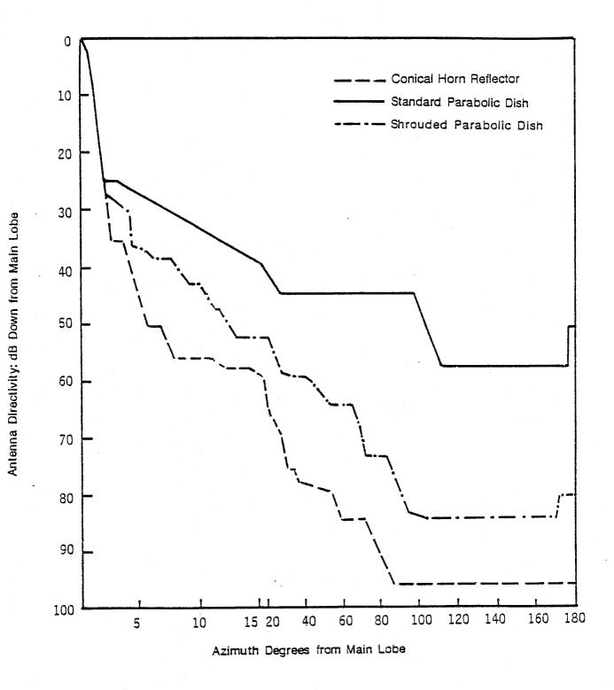
Figure 6-1. Comparison of typical 10 foot (3 m) 4/6 GHz Common Carrier Radio Relay Antennas.
