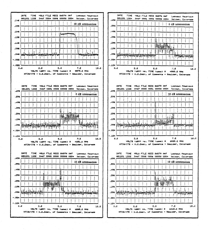
Figure 5-20. Pulse time waveform measurements of a WR100-2 (measured in a 30 MHz bandwidth).
