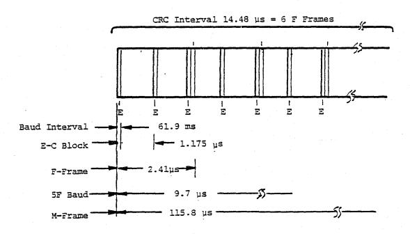
Figure A-5. Two (2) DS-3 IN 20 MHz, Error Correcting 64-QAM.
