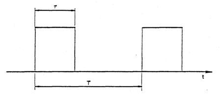
Figure E-1. Input radar pulse time waveform.
