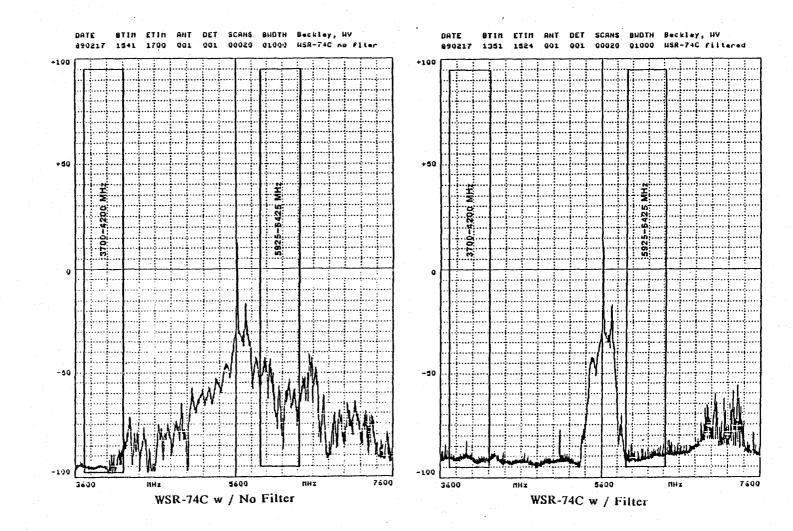
Figure 6-2. Radiated spectrum measurements of the WSR-74C radar at Beckley, WVA without and with an RF Filter.
