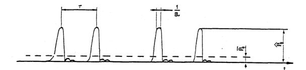
Figure E-2. Output time waveform for condition  $B_r > 1/T$  and large frequency deviation ( $\Delta f$ ) from the tuned frequency.
