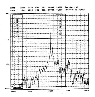
Figure 5-8. Radiated spectrum measurements of the WSR-74C radar at Beckley, WVA (pulsewidth = 3 us).
