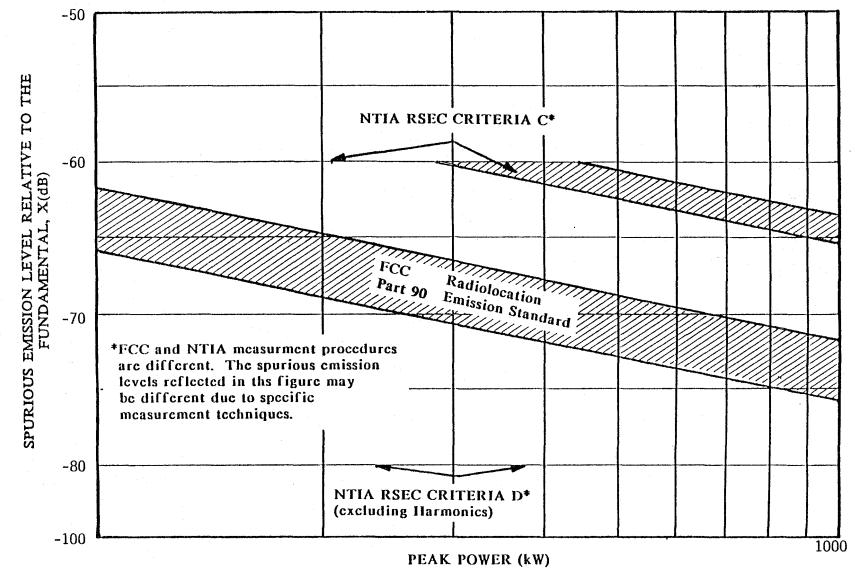
Figure 3-1. Comparison of spurious emission level standards for government and nongovernment meteorological radar stations.
