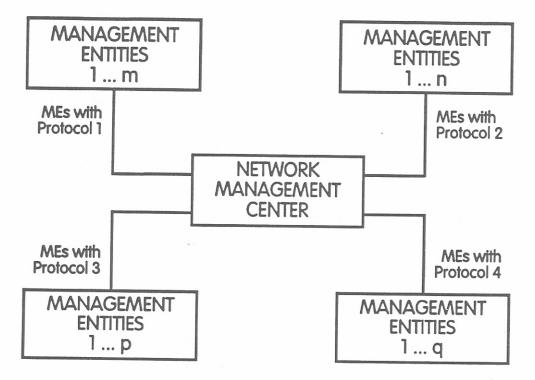
Figure 9. Centralized approach to network management.
