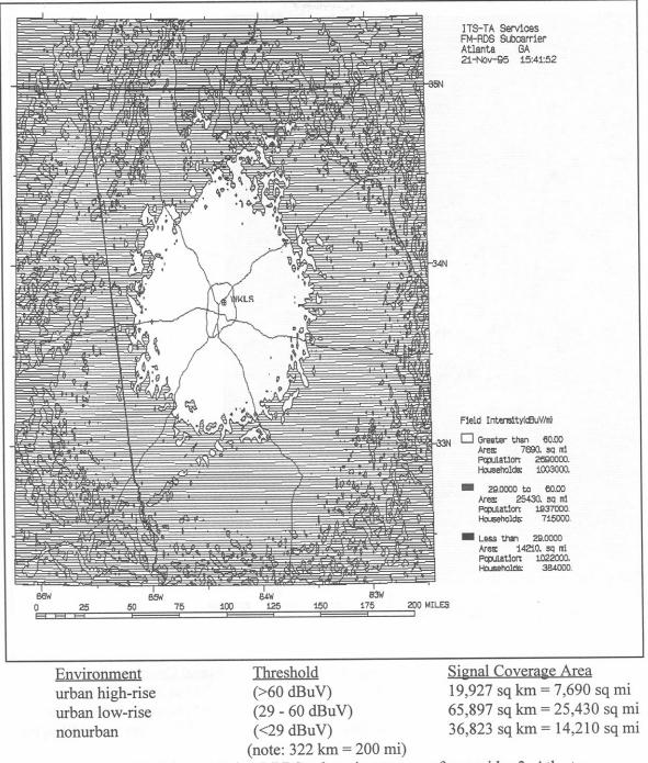
Figure 8. WKLS FM station RBDS subcarrier coverage for corridor 3, Atlanta.
