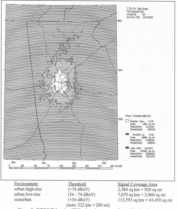
Figure 9. WRFG FM station STIC subcarrier coverage for corridor 3, Atlanta.
