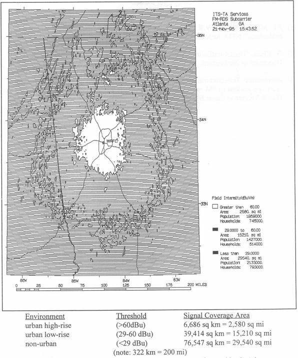
Figure 10. WRFG FM station RBDS subcarrier coverage for corridor 3, Atlanta.
