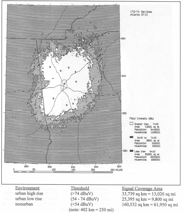
Figure 5. Composite FM station STIC subcarrier coverage for corridor 3, Atlanta.
