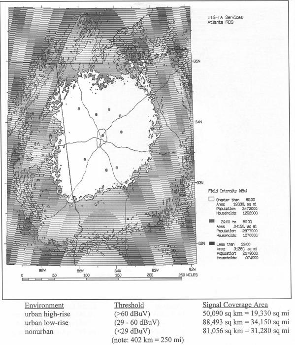
Figure 6. Composite FM station RBDS subcarrier coverage for corridor 3, Atlanta.
