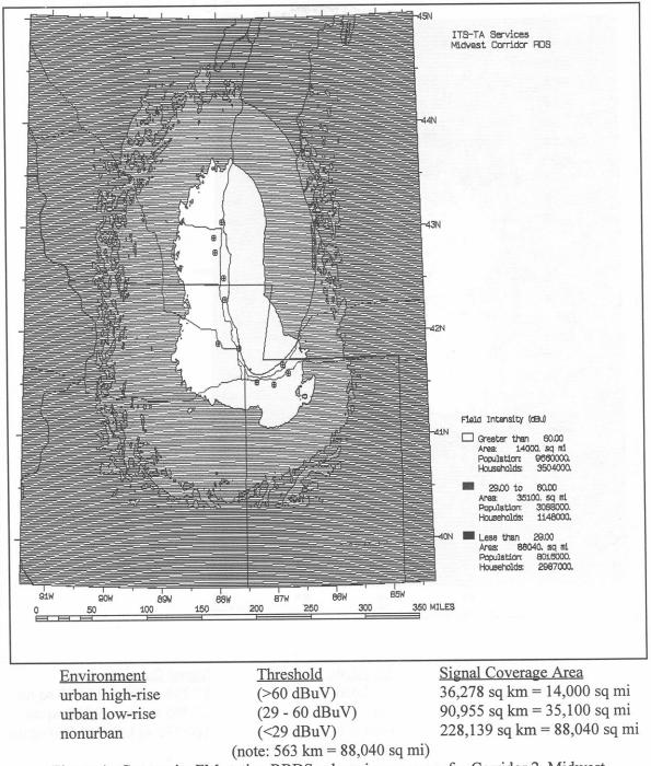
Figure 4. Composite FM station RBDS subcarrier coverage for Corridor 2, Midwest.
