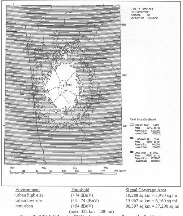
Figure 7. WKLS FM station STIC subcarrier coverage for corridor 3, Atlanta.
