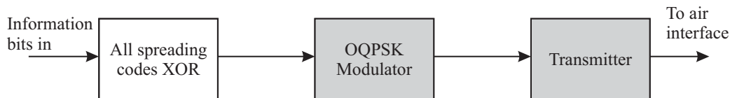
Figure 5.2. Abstracted reverse link block diagram.
