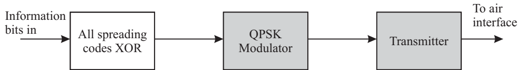
Figure 5.4. Abstracted forward link block diagram.
