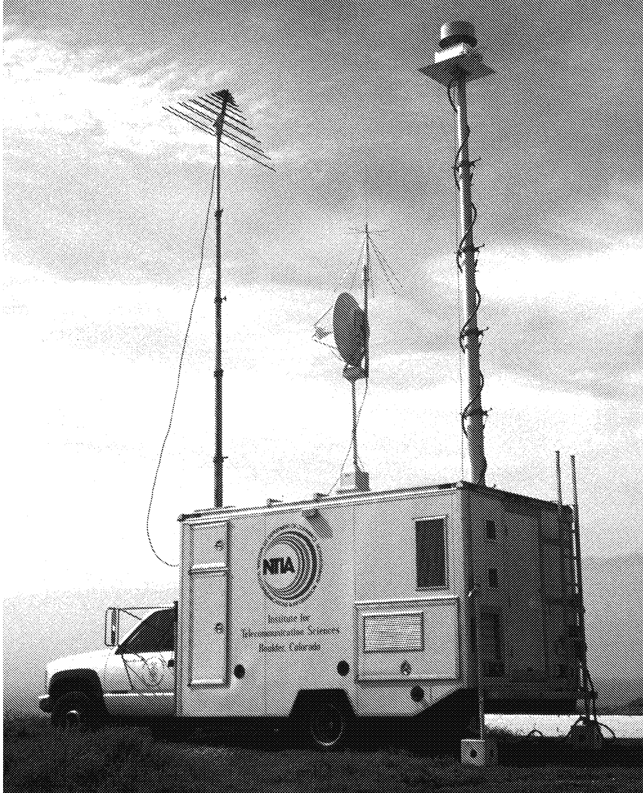
Figure C-1. ITS radio spectrum measurement system with telescoping masts raised and antennas mounted for a broadband spectrum survey at a remote field site.
