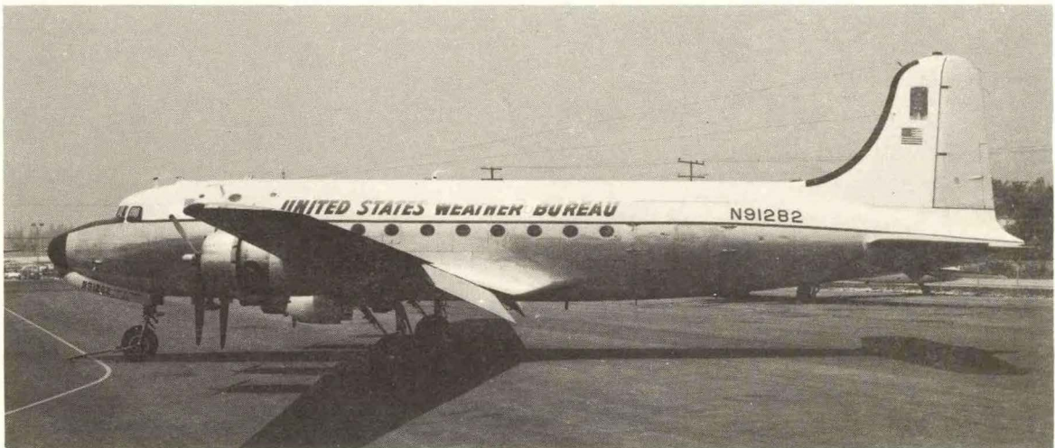
Fig. 22. RFF C-54 (DC-4) aircraft. Long range, unpressurized, four-engine (reciprocating type) land plane capable of flying at altitudes up to 25,000 ft, with a cruise speed of 217 knots (IAS), mission radius of 1350 nmi. In addition to its uses for operational research missions, the aircraft serves as a test-bed for developmental instrumentation and logistical support. The aircraft is equipped with standard and Doppler aids to navigation and a highly flexible communications system.
