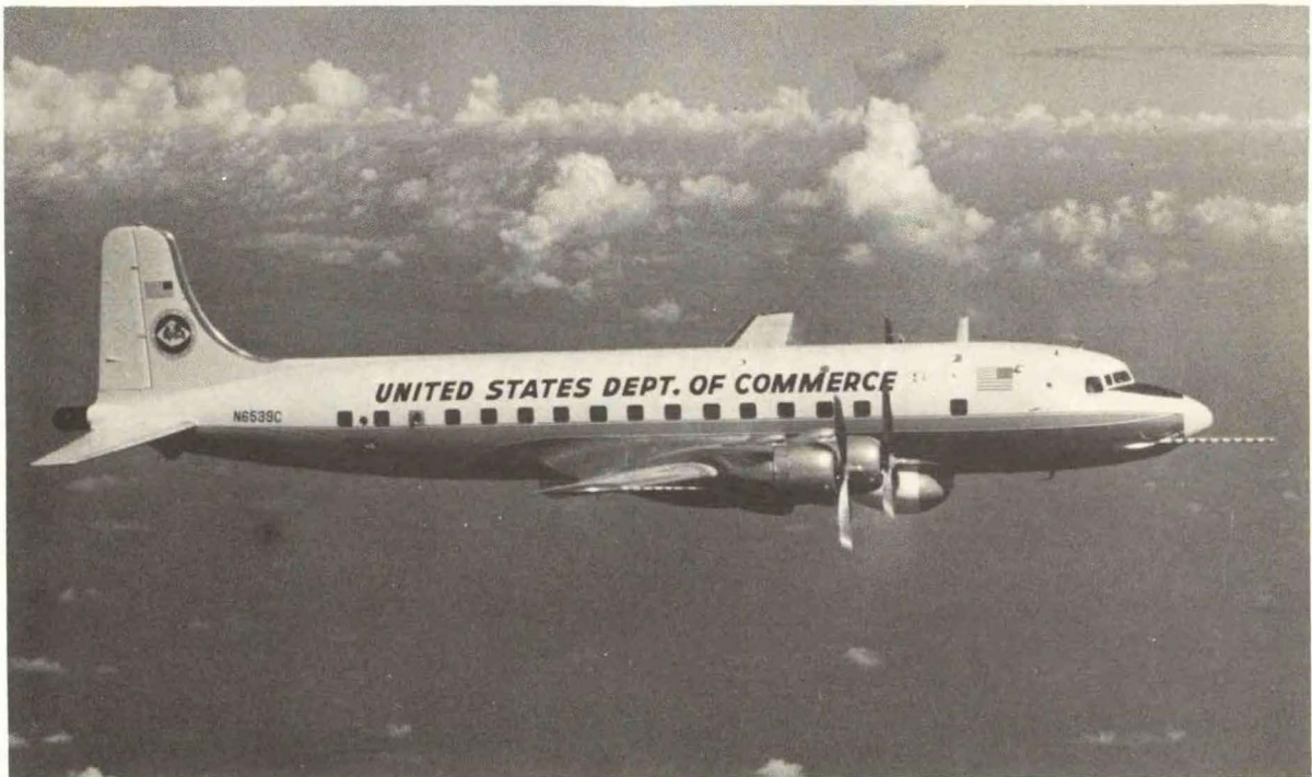
Fig. 20. RFF DC-6A/B aircraft. Long range, pressurized four-engine (reciprocating type) land plane capable of flying at altitudes up to 25,000 ft, with a cruise speed of 220 knots (TAS), mission radius of 1100 nmi and equipped with standard and Doppler aids to navigation with highly flexible communications system.
