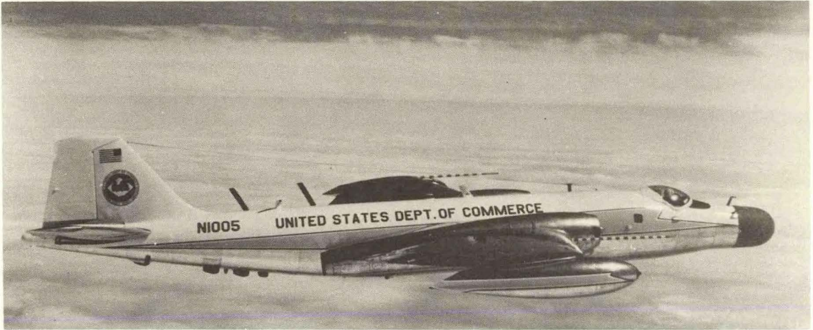
Fig. 21 . RFF B-57A aircraft. High altitude, twin jet research-reconnaissance aircraft, normally operated at altitudes between 30- and 45,000 feet at speed of approximately 430 knots (TAS), with a mission radius of 950 nmi. Standard and Doppler navigational/communications facilities are available on this aircraft.
