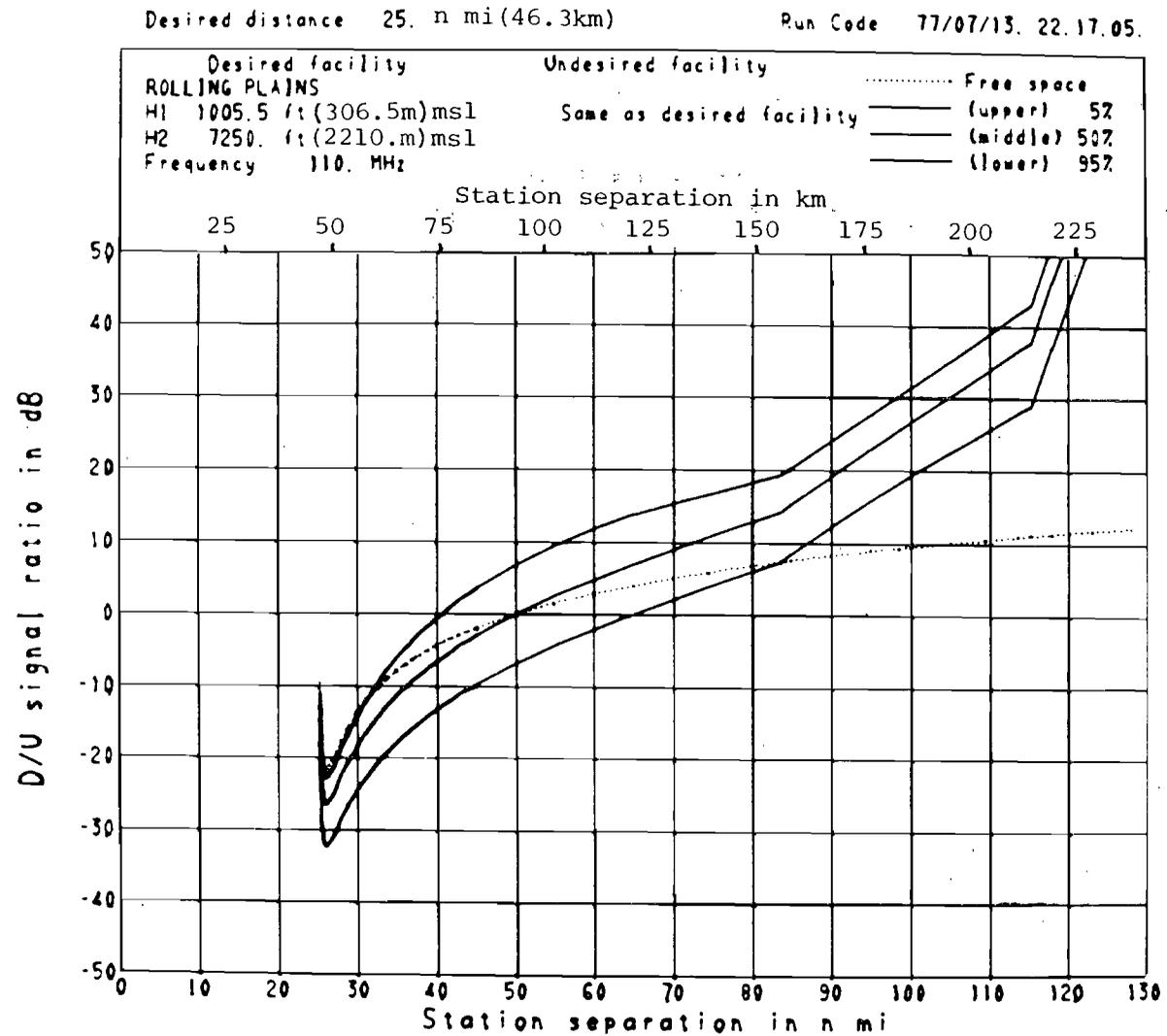
Figure A38. Signal ratio-S, ILS, rolling plains. Calculations were made for the parameters of figure A27 except with a  $\Delta h$  for rolling plains (195 ft, 59 m). Horizon parameters were calculated from  $\Delta h$ .
