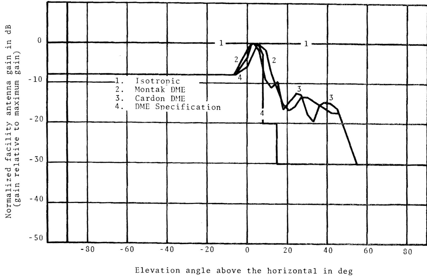
Figure 46. Normalized antenna gain vs. elevation angle, DME
