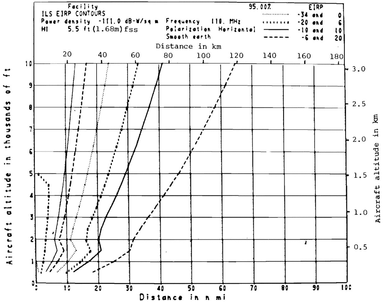
Figure 27. EIRP contours, ILS. EIRP contours are shown in the altitude vs. distance plane for a 95% time availability and the parameters of figure 2.
