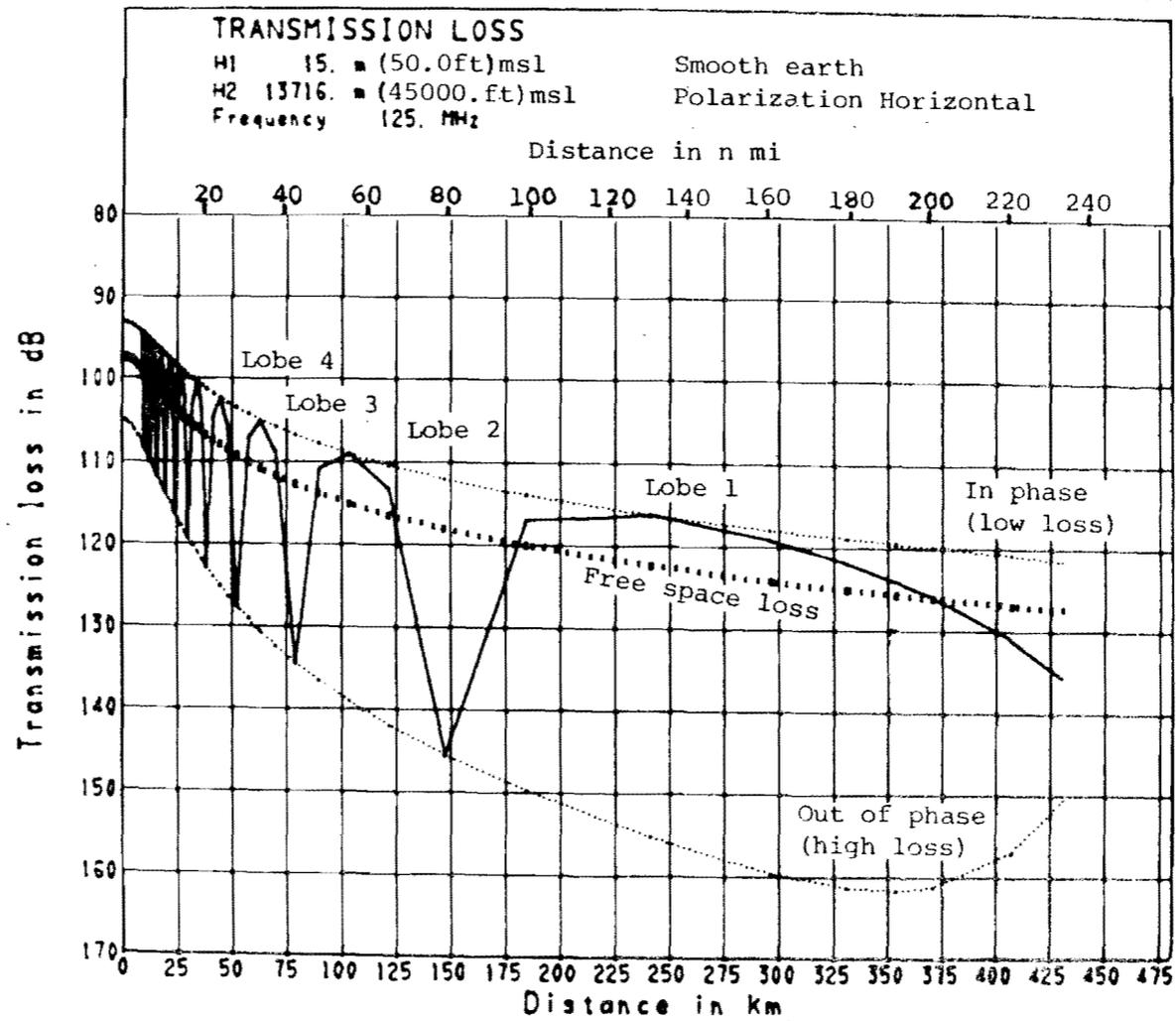
Figure 6. Lobing, ATC. Transmission loss for the first ten lobes inside the radio horizon, limiting values associated with in and out of phase conditions and free-space loss vs. path distance are shown. These curves were computed for the parameters of figure 1.
