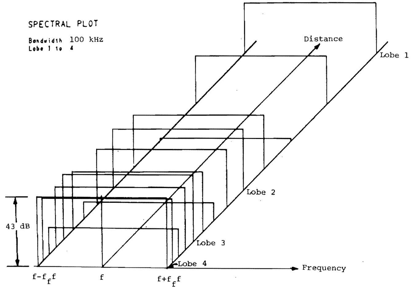
Figure 15. Spectral plot, ATC. Fading across flat spectra with 100 kHz bandwidth for the lobing structure in figure 6 and parameters of figure 1.
