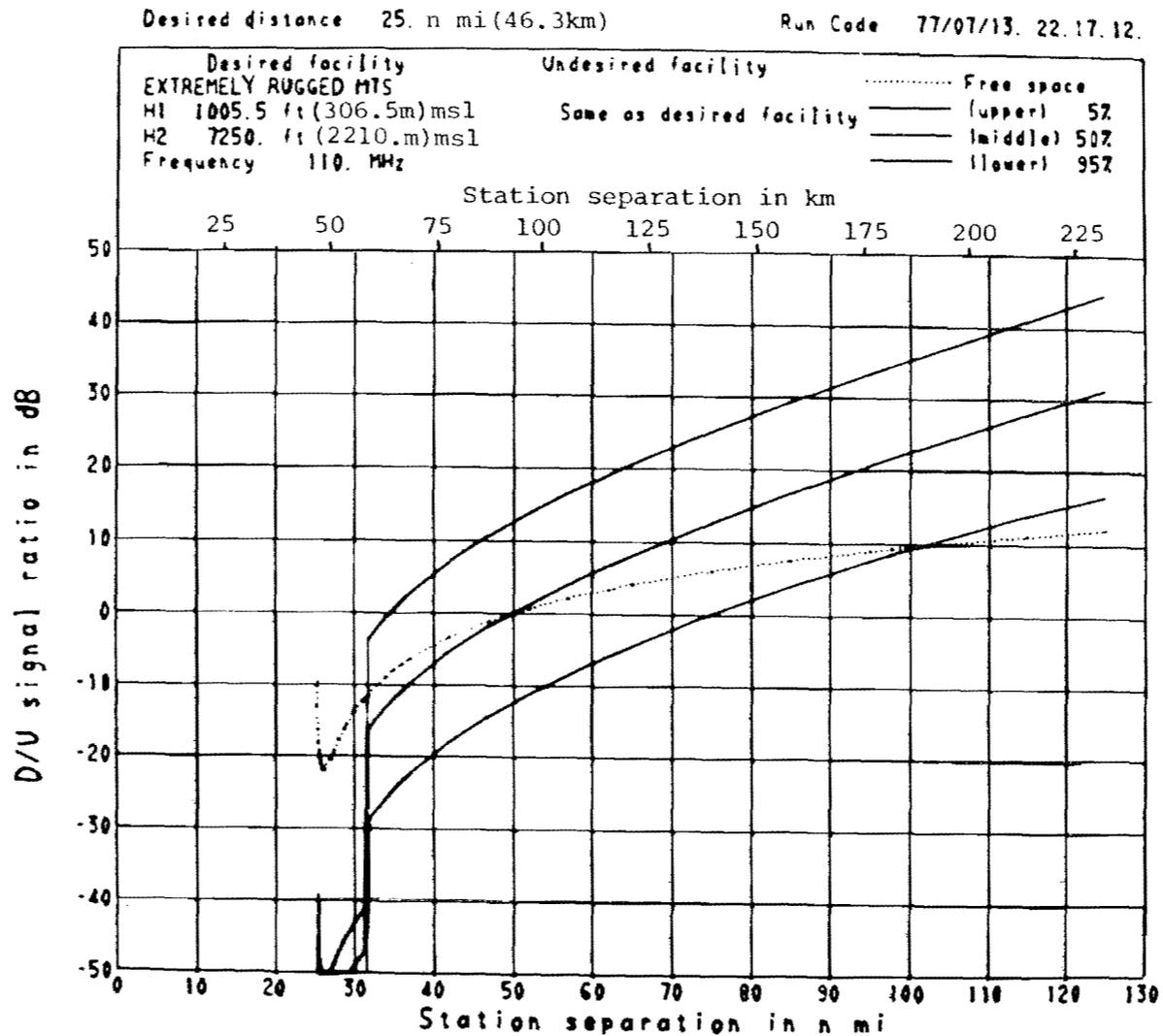
Figure A41. Signal ratio-S, ILS, extremely rugged mountains. Calculations were made for the parameters of figure A27 except with a  $\Delta h$  for extremely rugged mountains (2,625 ft; 800 m). Horizon parameters were calculated from  $\Delta h$ .
