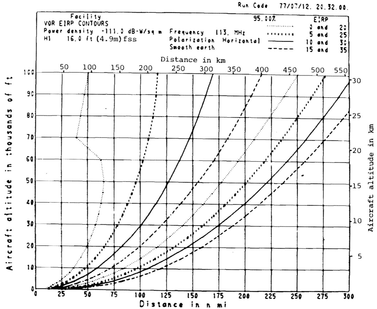
Figure 29. EIRP contours, VOR. EIRP contours are shown in the altitude vs. distance plane for a 95% time availability and the parameters of figure 5.
