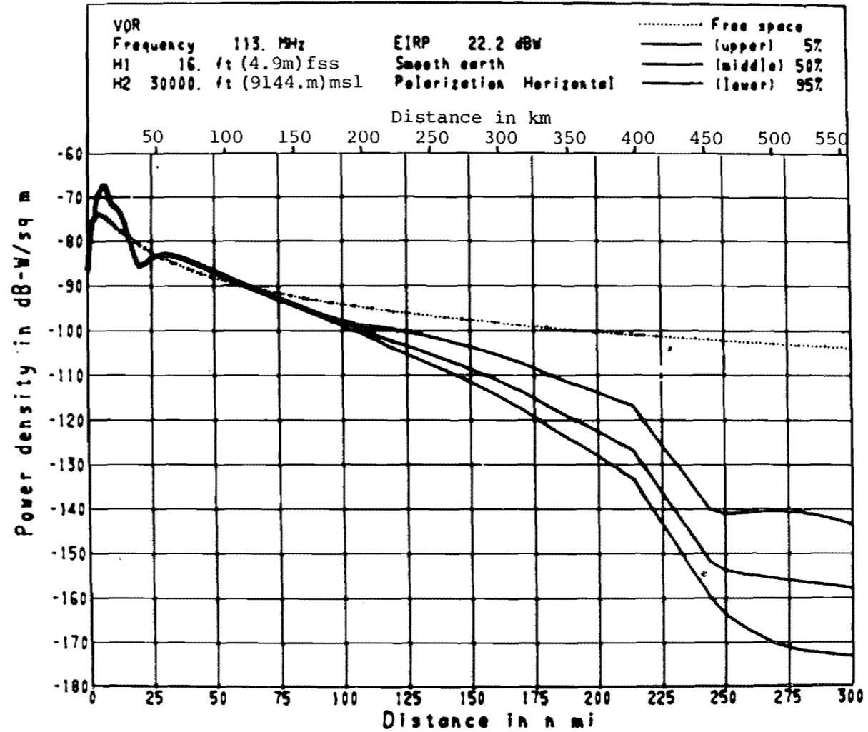
Figure 19. Power density, VOR. Parameters used in the calculations are summarized in figure 5.
