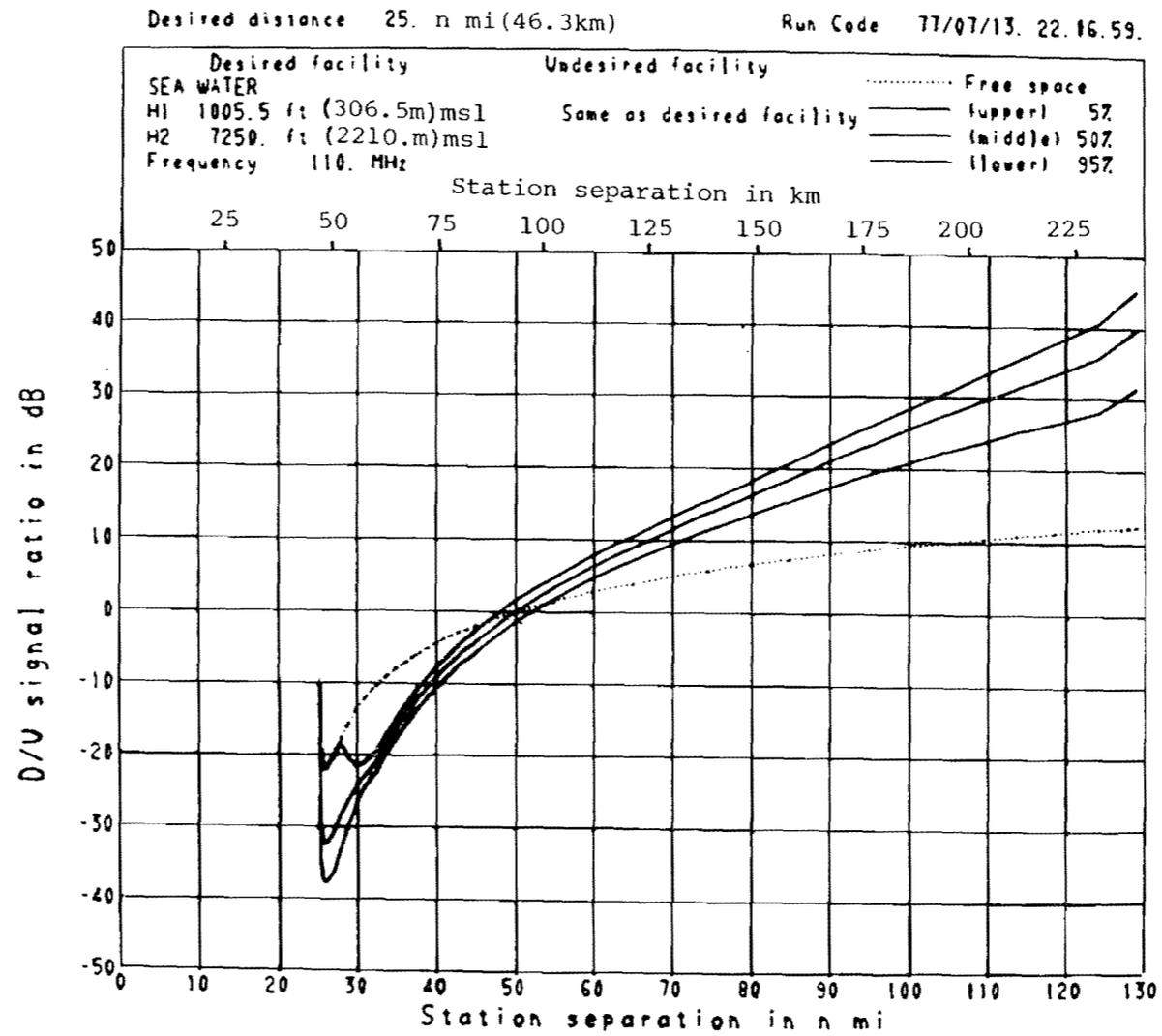
Figure A35. Signal ratio-S, ILS, sea water. Parameters are as given in figure A27 except for surface type.
