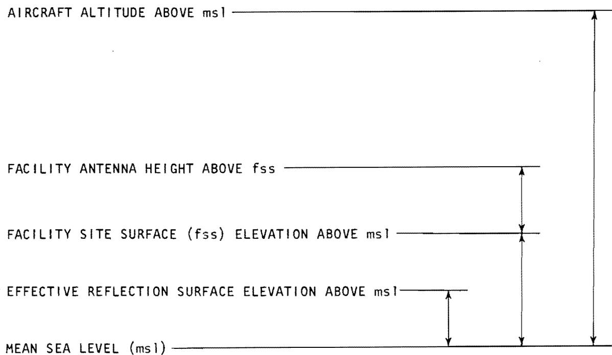
Figure 44. Antenna heights and surface elevations. Note that the aircraft altitude is elevation above msl while the facility antenna height is measured with respect to fss.
