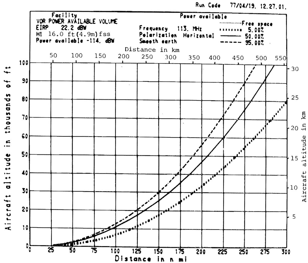
Figure 24. Power available volume, VOR. Power available volume for a single power available for 5, 50, and 95 percent time availability using the parameters in figure 5.
