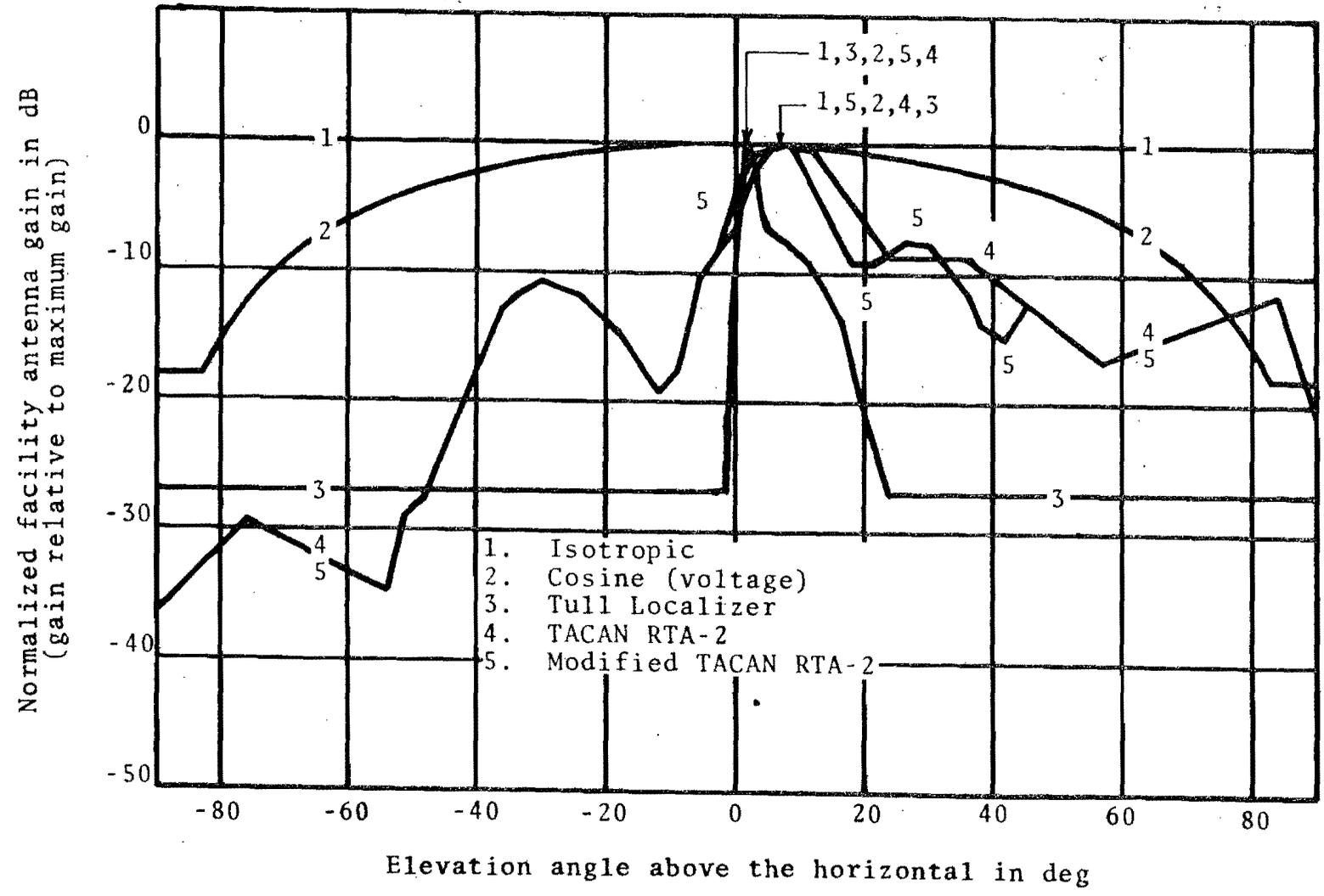
Figure 45. Normalized antenna gain vs. elevation angle.
