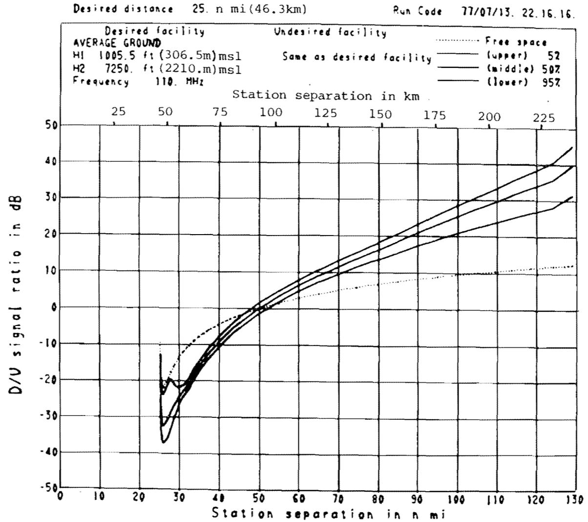
Figure A33. Signal ratio-S, ILS, average ground. Parameters are as given in figure A27.
