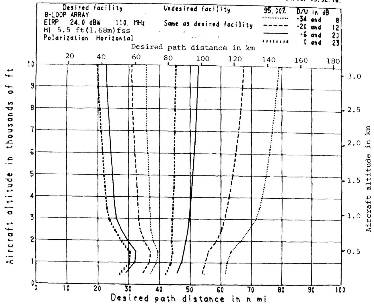
Figure 38. Signal ratio contours, ILS. Parameters used in the calculations are summarized in figure 2.
