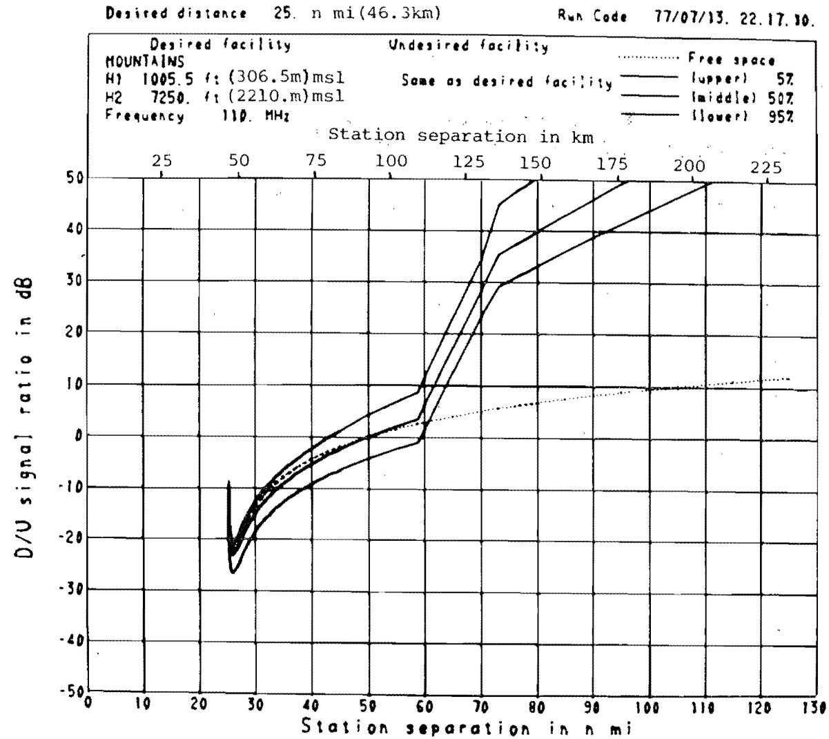
Figure A40. Signal ratio-S, ILS, mountains. Calculations were made for the parameters of figure A27 except with a  $\Delta h$  for mountains (740 ft, 226 m). Horizon parameters were calculated from  $\Delta h$ .
