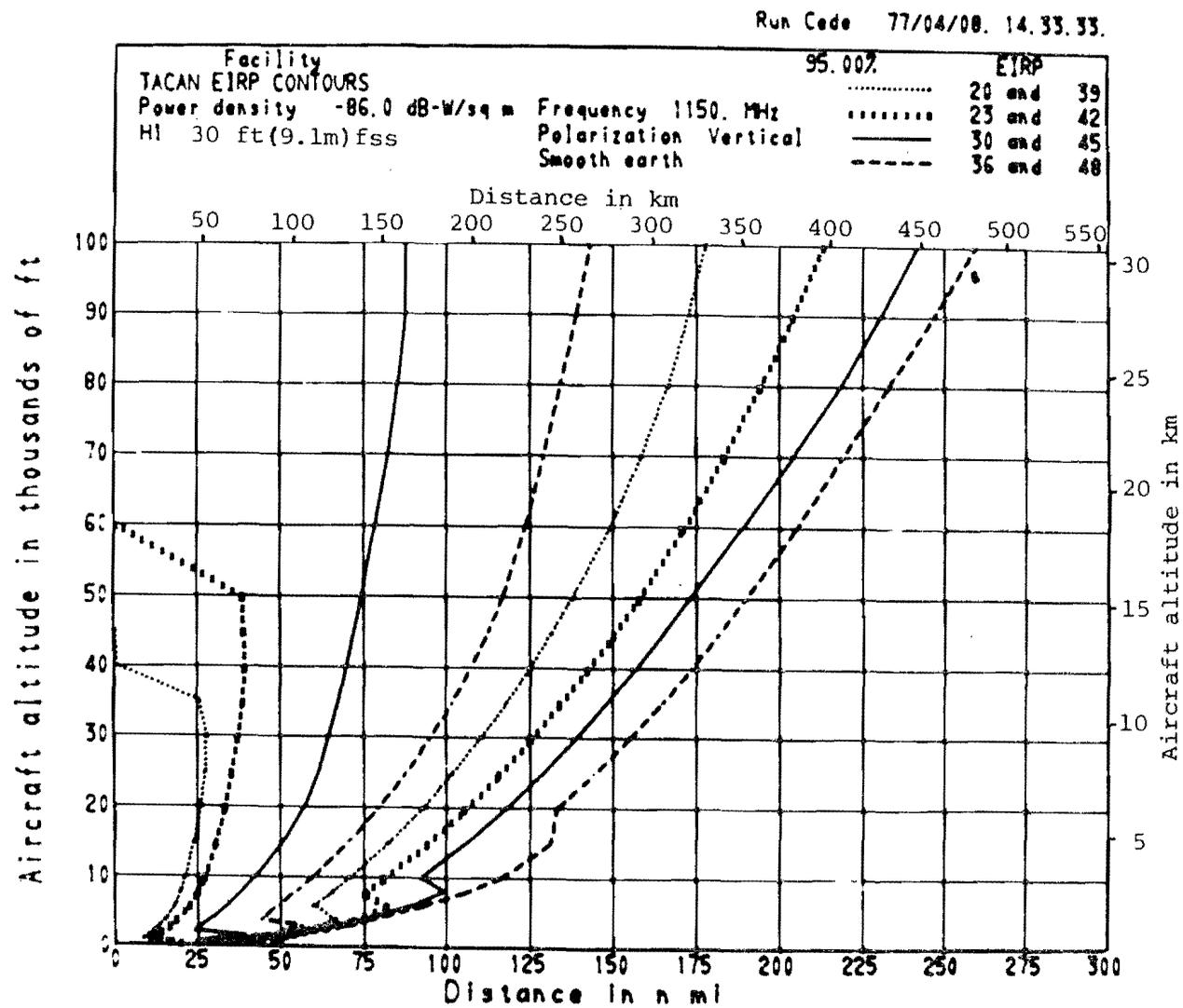
Figure 28. EIRP contours, TACAN. EIRP contours are shown in the altitude vs. distance plane for a 95% time availability and the parameters of figure 4.
