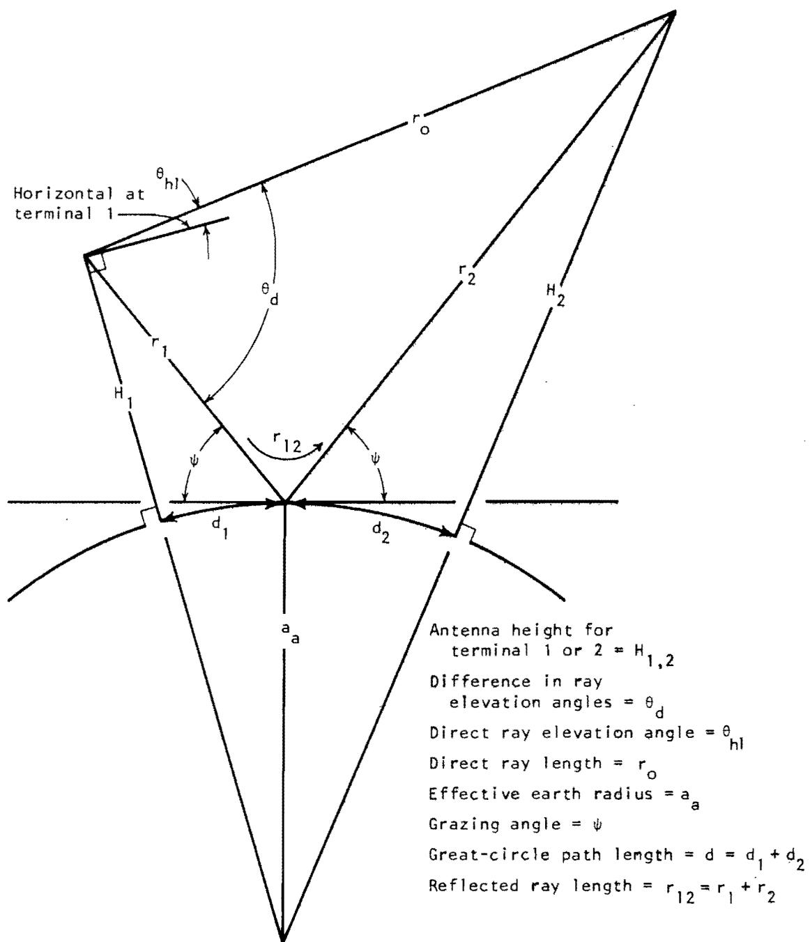
Figure 40. Geometry for reflection from spherical earth.
