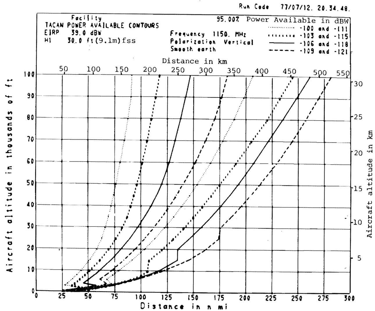
Figure 30. Power available contours, TACAN. Power available contours are shown in the altitude vs. distance plane for a 95% time availability and the parameters of figure 4.
