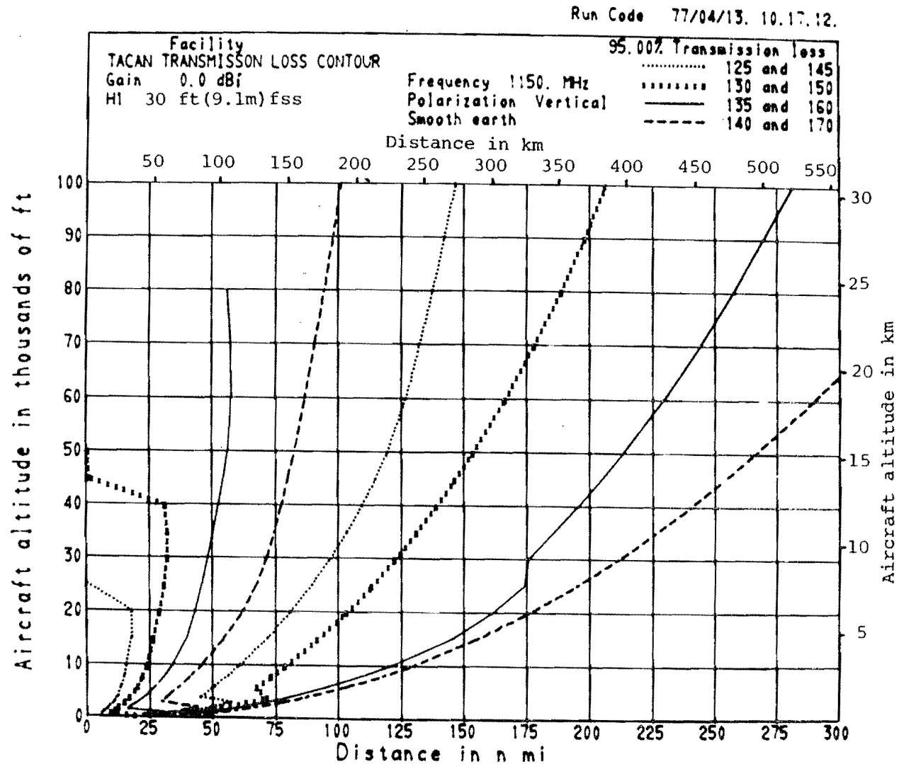
Figure 32. Transmission loss contours, TACAN. Transmission contours are shown in the altitude vs. distance plane for a 95% time availability, and the parameters of figure 4.
