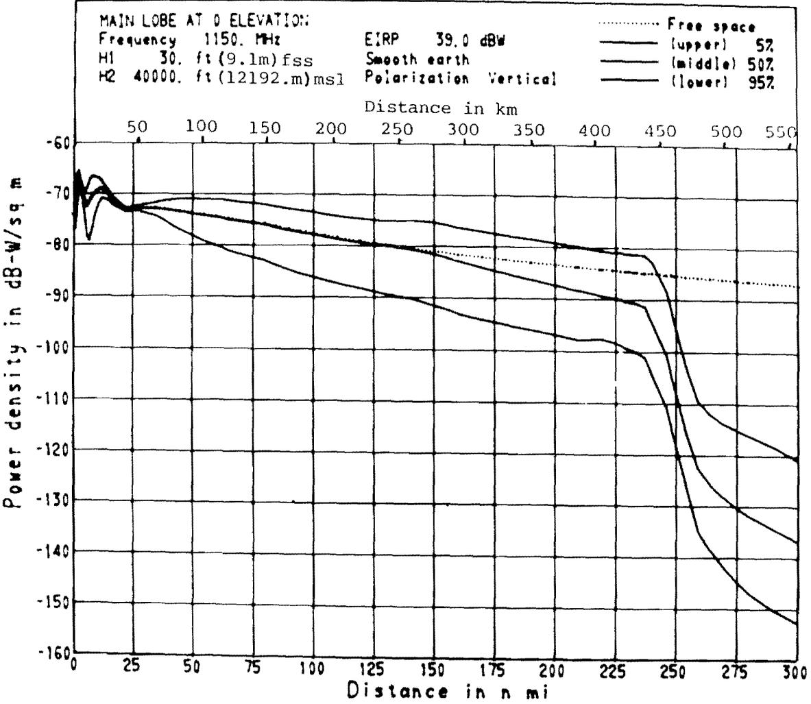
Figure A15. Power density, TACAN, main lobe at 0° elevation. Power density values were computed with parameters from figure A13 except for elevation angle.
