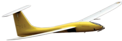
The Tempest UAV was developed to fly into severe storms to study tornadogenesis. Photo courtesy RECUV.
