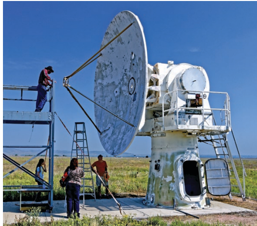
Wayde Allen, Linh Vu, Teresa Rusyn, and John Ewan take measurements of the dish antenna that will be used to collect GPS signal data for validating future propagation models. Photo by Tim Riley.
