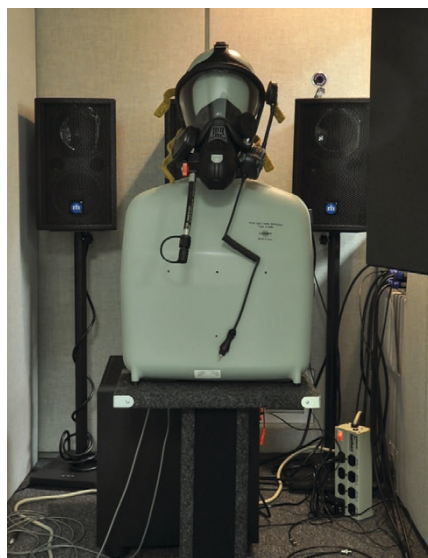
An ITU-Standard head and torso simulator (HATS) set up in a sound-isolated booth for testing public safety communications. Photo by Andrew Catellier.
