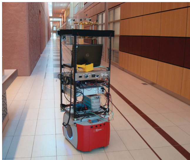
Figure 2. The robot carries all the components of an automated measurement system, including the omnidirectional antenna perched on top of the rack. It moves autonomously along a pre-programmed path, while the system collects data on signals being transmitted from up to 150 m away. Photo by P. Papazian.
