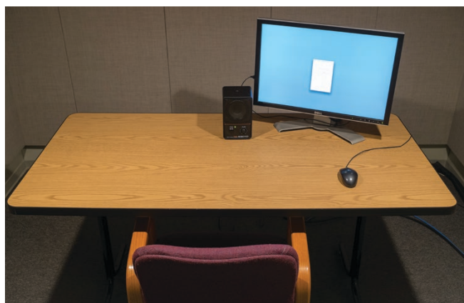
Setup for speech intelligibility testing in a standards-compliant sound isolation booth in the ITS lab. Photo by A. Catellier.
