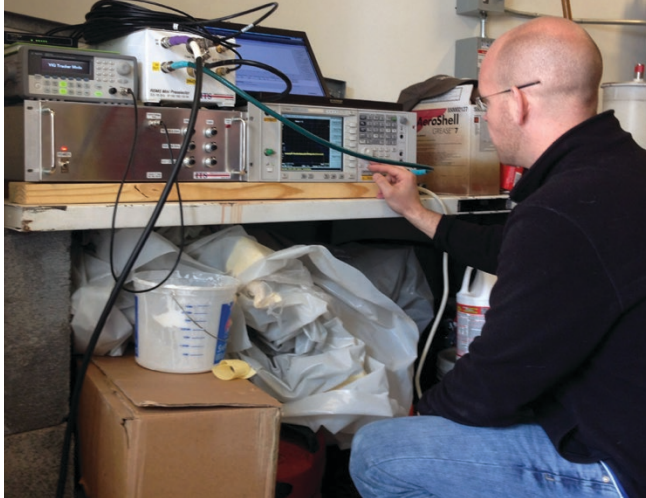
ITS engineer John Carroll setting up a suitcase radio spectrum measurement system at a field site. Photo by Frank Sanders.
