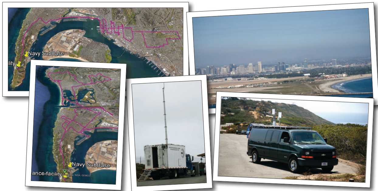
Figure 1. Snapshots of San Diego measurement campaign. Push pins in Google Earth™ show transmitting locations from the CNM maintenance facility and the Navy submarine base; drive routes are shown by the purple traces. The transmitting truck is shown in the center photo and the receiving van is shown in the lower right photo. Map data ©2015 Google.
