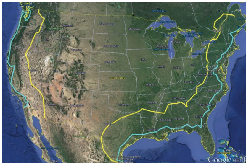
This screenshot from Google Earth™ shows the exclusion zones for the protection of radar operations in the lower 48 states before (yellow line) and after application of the new extended Hata model (blue line).
