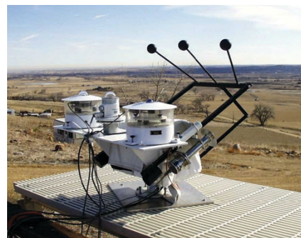
SURFRAD instruments mounted on a solar tracker on an instrument deck at Table Mountain. Photo courtesy NOAA.
