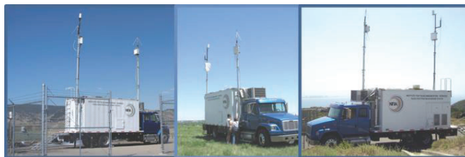
Fig. 1. The RSMS-4 truck shown at three locations for spectrum occupancy measurements: Table Mountain, CO; Denver, CO; and San Diego, CA.
