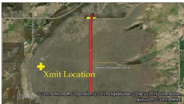
Fig. 5. Table Mountain map showing mobile drive route (red circles), the transmitting location (yellow cross), and the edge of the mesa (yellow horizontal line).
