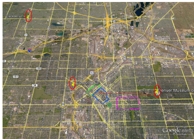
Fig. 10. This figure shows the three transmit locations (red circles) and three measurement routes on Google Earth®. The area outlined in green contains the low-rise downtown area buildings, the area outlined in purple contains the high-rise urban area buildings, and the area outlined in pink contains the area of residential buildings.
