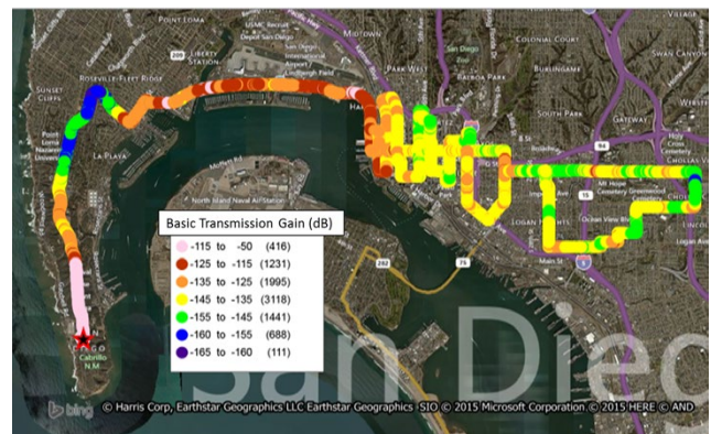
Fig. 7. Median basic transmission gain values along drive route 2 at a frequency of 1760 MHz.
