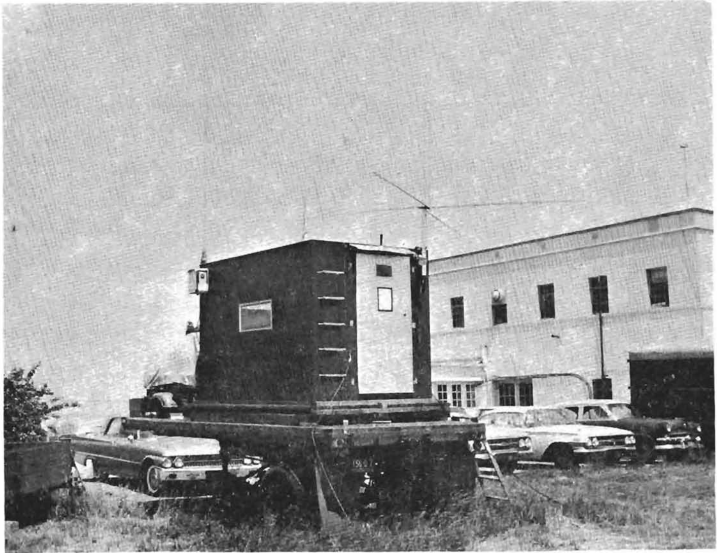
Figure 2. TRANSMITTER SHELTER FOR OHIO MEASUREMENTS
