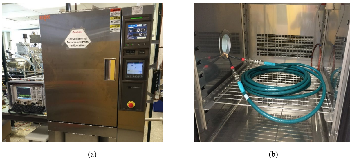
Fig. D-1: (a) NIST environmental chamber and (b) 15.2 m cable being tested within the chamber.
