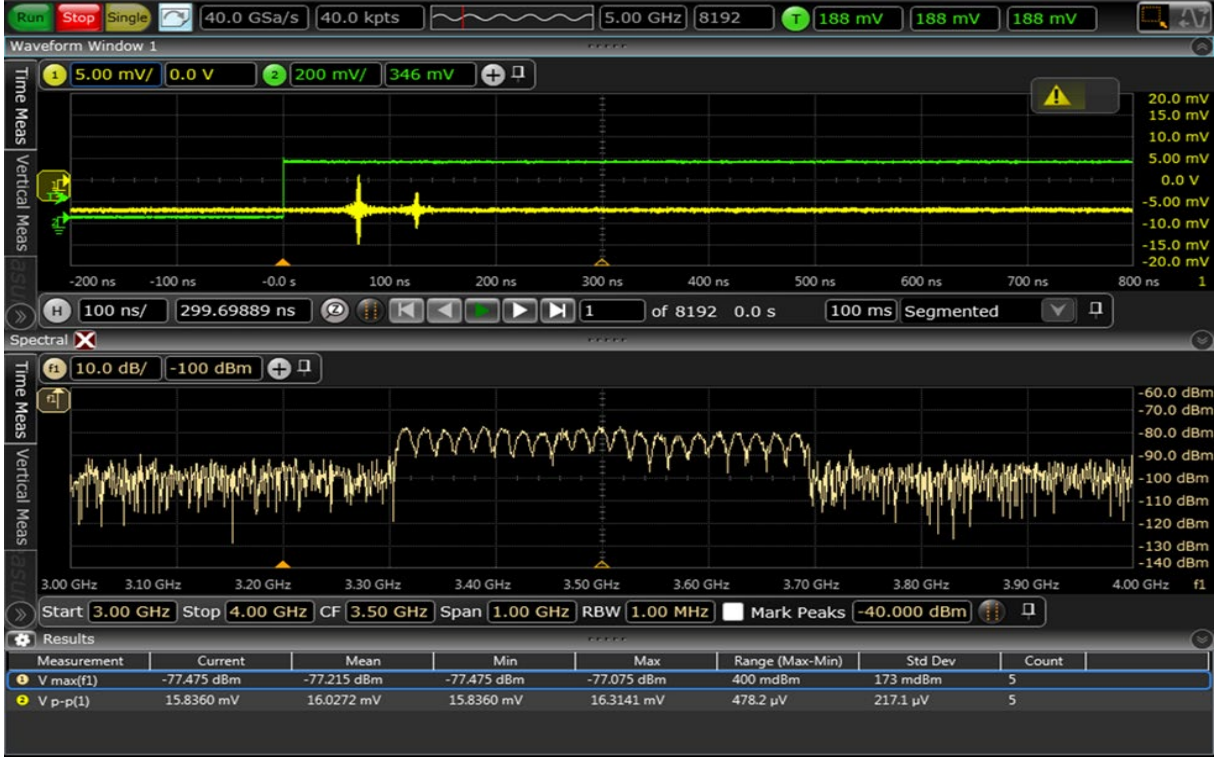
Fig. 5-9: Screen shot of the Direct-Pulse channel sounder for the direct-and-bounce-path channel. The mention of brand names does not imply an endorsement by NIST or NTIA. Other products may work as well or better.
