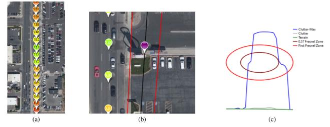
Fig. 6. (a) Roadway sign causing diffraction losses in a LOS classified path. (b) Satellite view showing geometry of direct ray (black) and first Fresnel zone (red). (c) Horizontal profile from re-extracted lidar point cloud data. Bing Maps screenshots reprinted with permission from Microsoft Corporation.
