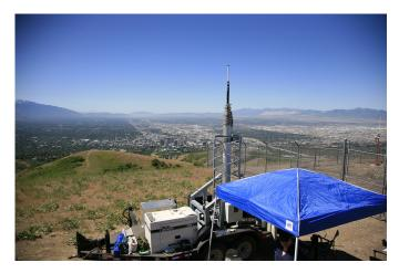
Fig. 1. View from transmitter site, looking south towards downtown Salt Lake City, UT. The paths from the transmitter site to the measurement area have first Fresnel zone clearance of the terrain located in the foreground.
