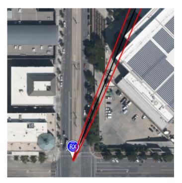
Fig. 5. A vertical grazing diffraction edge. The black line is the direct ray path and the red line is the first Fresnel zone. Bing Maps screenshot reprinted with permission from Microsoft Corporation.
