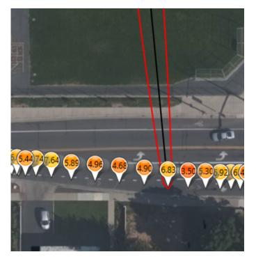
Fig. 7. Impact of metal screen on clutter loss for a traditionally defined lineof-sight path. The black line is the direct ray path and the red line is the first Fresnel zone. Bing Maps screenshot reprinted with permission from Microsoft Corporation.
