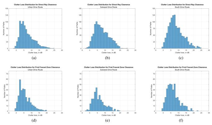
Fig. 3. Distribution of measured clutter loss for paths containing direct ray clearance for measurement routes (a) Urban, (b) Subwest, and (c) South. Distribution of measured clutter loss for paths containing first Fresnel zone clearance for measurement routes (d) Urban, (e) Subwest, and (f) South.
