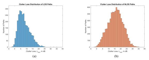
Fig. 4. Distribution of clutter loss (a) for line-of-sight (LOS) and (b) non-line-of-sight (NLOS) measurement data points.
