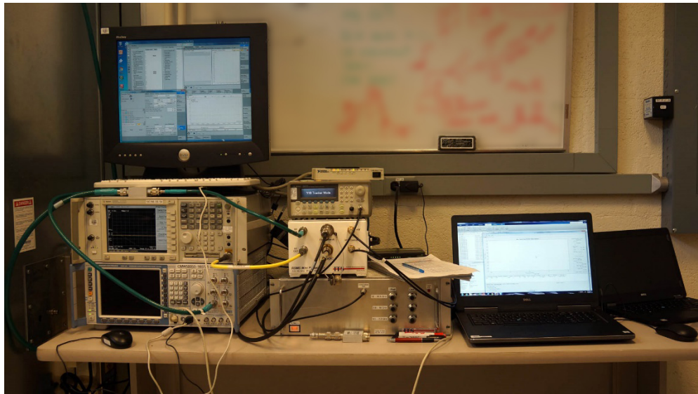
Figure 8. UE measurement system boxes including the CMW-500 (lower left), E4440A (on top of the CMW-500), RF front end (white box at center), RF front end auxiliary boxes (above and below it) and the controller laptop computer (far right).
